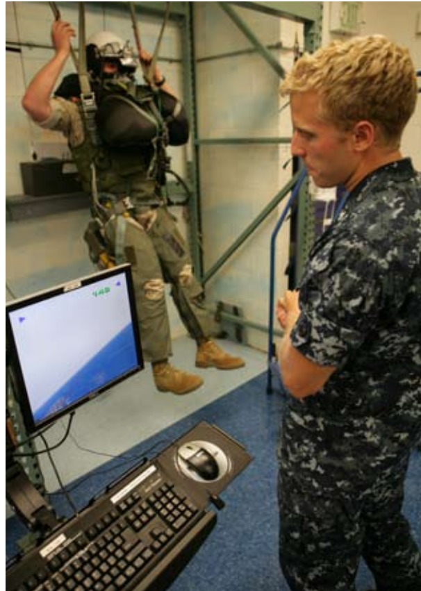
A Marine assigned to Marine Aviation Weapons and Tactics Squadron One (MAWTS-1) performs a virtual parachute landing while a Sailor operates the Virtual Parachute Trainer.
