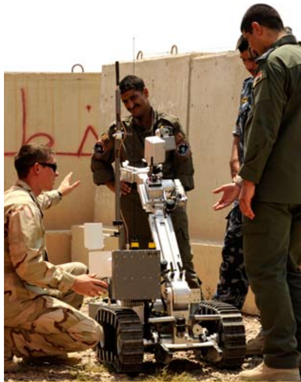
A Petty Officer 1st Class, assigned to Explosive Ordnance Disposal Mobile Unit (EODMU) 2, Company 2-2, discusses components of the mini Remote Ordnance Neutralization System robot with soldiers assigned to the 5th Iraqi Army Bomb Disposal Company.
