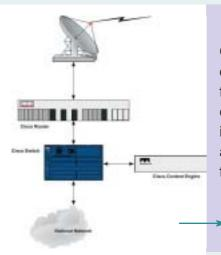
One earth station, composed of a satellite dish and a router to direct the Internet traffic, will be set up in each of the participating countries. NRENs are responsible for installing and maintaining their earth station and deciding which research and education facilities will be connected to it.
