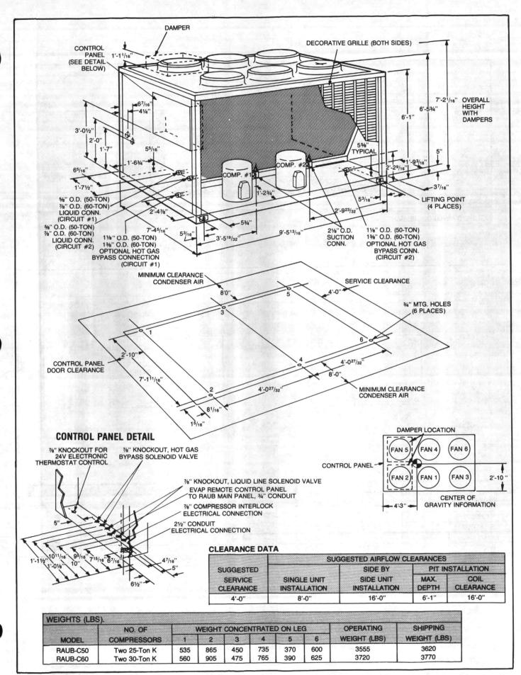
FIGURE 8 - Dimensional Data, RAUB C50 and C60
