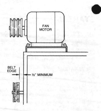
Figure 52 - Minimum Allowable Distance Between Frame Work and Fan Sheave.
