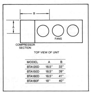
Figure 5 - Unit Center of Gravity Information
