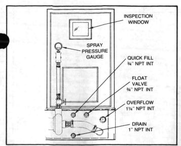
FIGURE 33A - Sprayed Coil Unit Tank Connections
