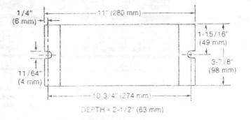
Figure 4. Mounting Dimensions
