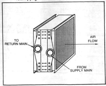
Figure 49 - Typical Piping for Type D, W or K Water Cooling Coils with End Connections.
