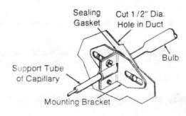
Figure 3. Duct Mounting with AT-208
