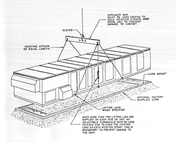
Units will have lifting lugs welded and/or bolted to the base when specified.
