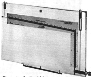
Figure 3 — Inclined Manometer
