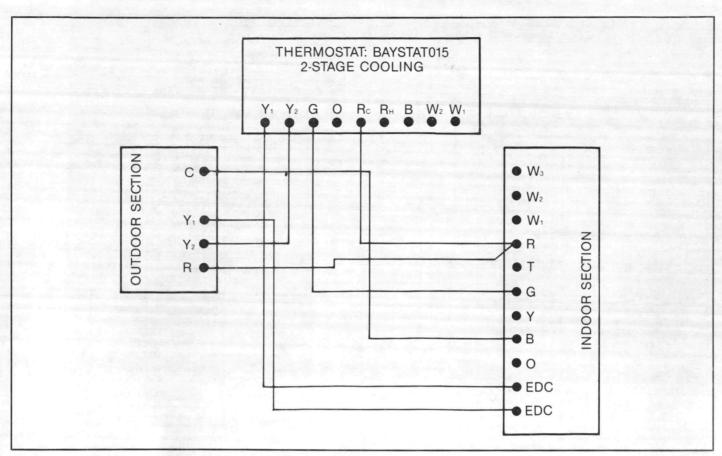
Figure 9 - Field Wiring for BTA120D with BTE120B Air Handler No Electric Heat
