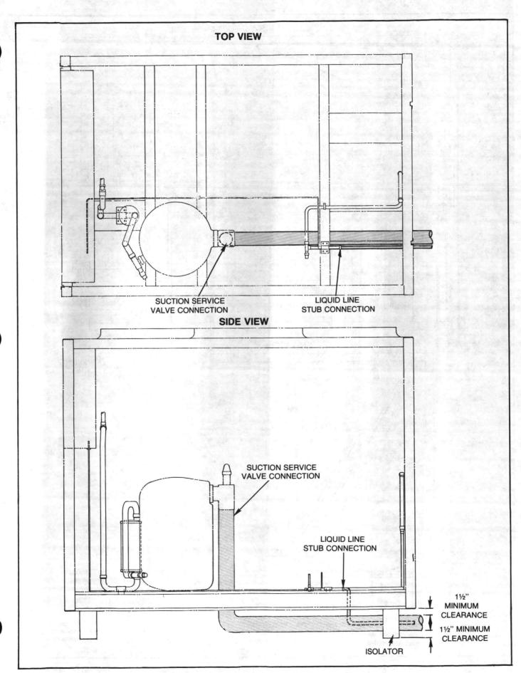
FIGURE 18 - Piping Installation: 20 Through 30-Ton Units With Isolators
