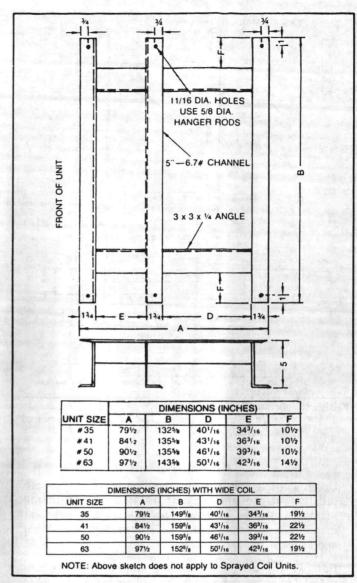
FIGURE 12 - Ceiling Suspension Mounting Frame and Dimensions for Unit Sizes 35 to 63
