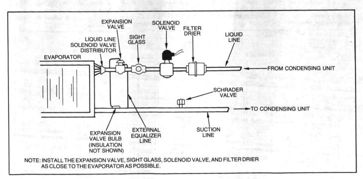
FIGURE 14 - Diagram of Refrigerant Piping Components in Liquid Line
