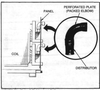
FIGURE 51 - Type F Refrigerant Coil
