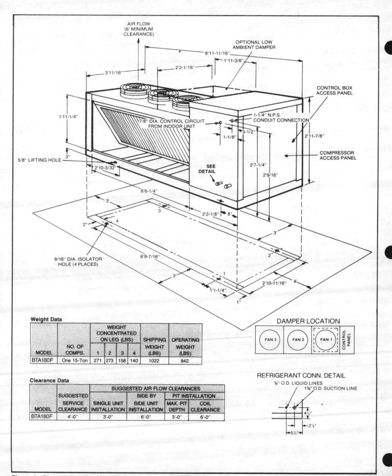
Figure 3 · Dimensions, Weights, and Clearances for BTA180F Units
