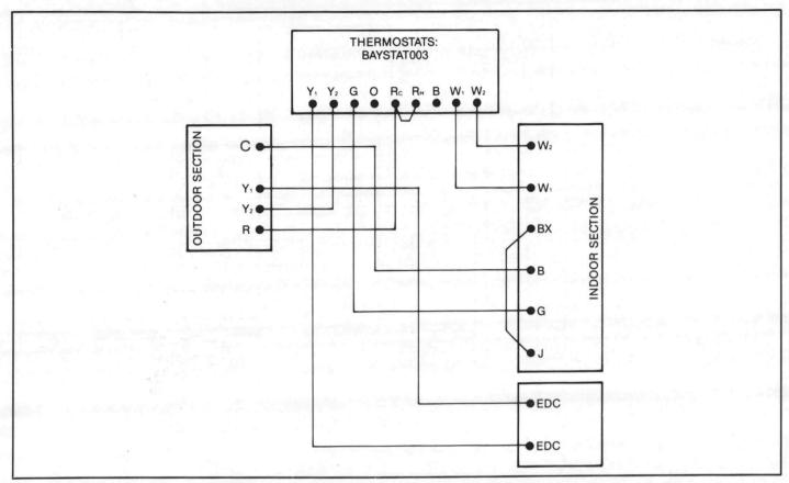
Figure 15 - Field Wiring for BTA150D, BTA180D and BTA180F With the BWV180B, BWH180B Air Handlers With Electric Heat
