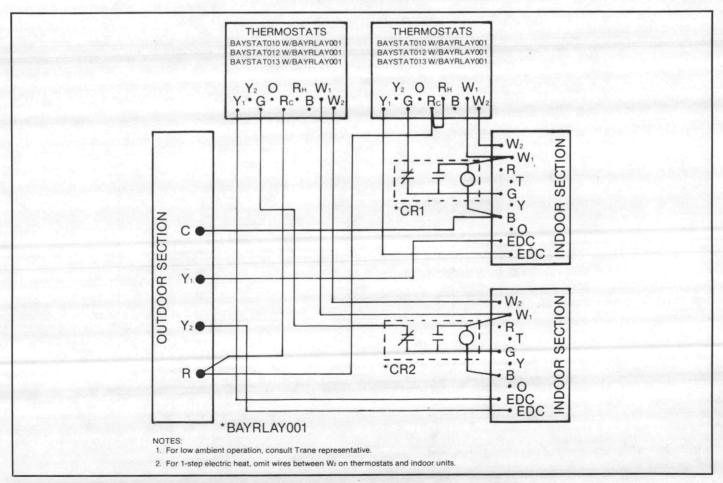
Figure 12 - Field Wiring for BTA150D and BTA180D With Two (2) BWE090C Air Handlers
