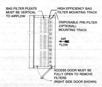
FIGURE 1 - Filter Mounting Track Location (Top View)
