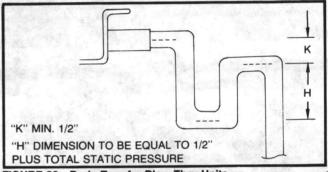
FIGURE 32 - Drain Trap for Blow-Thru Units
