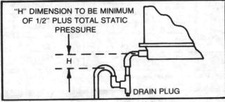
FIGURE 31 - Drain Trap for Draw-Thru Units
