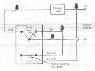
Figure 8. Typical of Parallel Cooling Anticipation (anticipator size determined by voltage)
