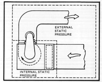
FIG. 37 - AIR MOVING SYSTEM
