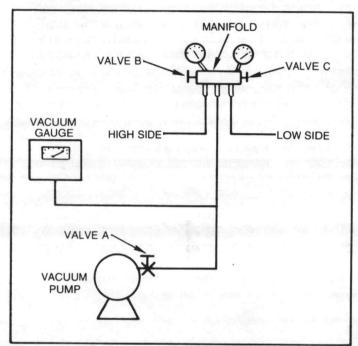
Figure 7 - Vacuum Pump Hook-Up
