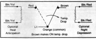
Figure 1. Switch Action and Lead Identification
