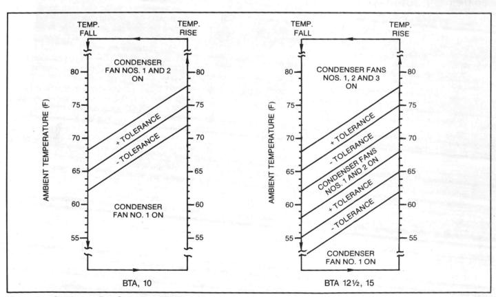
Figure 5 - Condenser Fan Operating Modes
