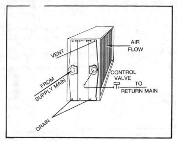
Figure 50 - Typical Piping for Type DD Water Cooling Coil with Center Connections.
