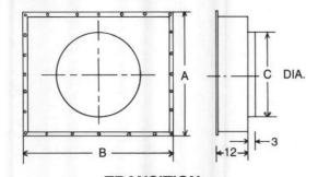
TRANSITION (Connected to air cleaner discharge at factory)
