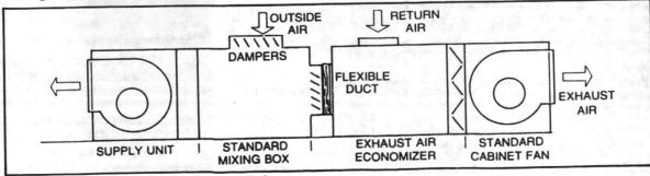
FIGURE 22 - Exhaust Air Economizer Installation
