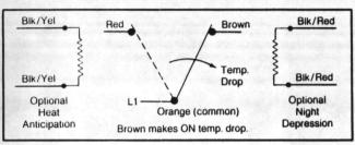
Figure 1. Switch Action and Lead Identification
