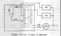
THERMOSTAT CYCLES HEAT AND COOL, HEAT-COOL SYSTEM SWITCH
