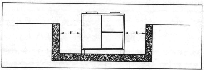
FIGURE 9 - Well Installation
