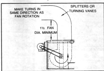
FIGURE 28 - Discharge Ductwork Recommendations
