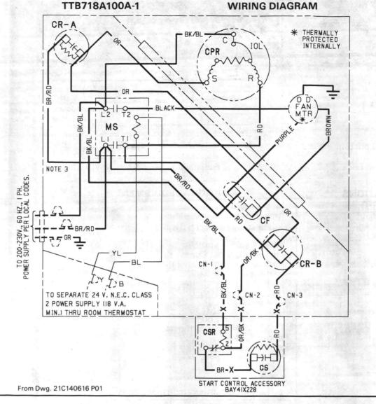
LEGEND Factory Wiring Line V 24 V. Field Wiring Line V. Field Installed **Factory Wiring** Ground Junction Wire Nut or Connector Coil -)-Capacitor Relay Contact (N.O.) Relay Contact (N.C.) o Internal Overload Protector o Motor Winding o Fuse Color of Wire Black Wire with Blue Marker Color of Marker Black Yellow Orange YL BL BR Green Brown WH White PR Fan Capacitor Run Capacitor CPR CS CRS
