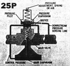
the pressure pilot and the control pressure bleeds back through the control orifice. This allows the main valve to hold the desired reduced pressure and it may close tight for a dead-end shutoff.
