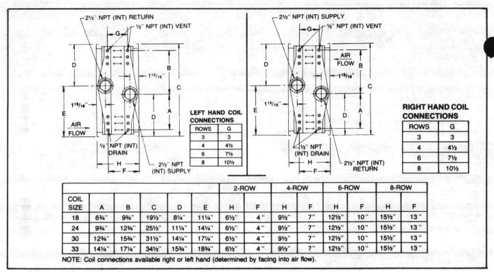
FIGURE 38 - Coll Type W Connections With Drain and Vent Locations (18", 24", 30", and 33" Headers)
