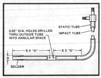
Figure 1 — Construction of Pitot Tube
