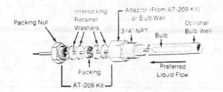
Figure 5. AT-201 or AT-203 Installation
