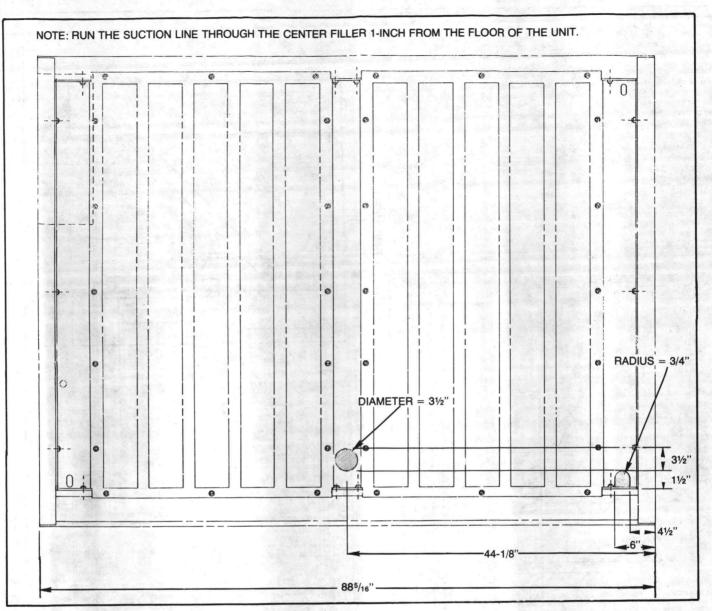
FIGURE 20 - Hole Locations: 20 Through 30-Ton Units
