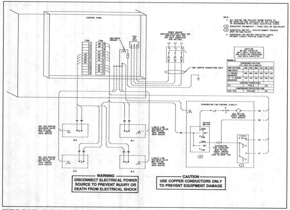
FIGURE 27 - Field Wiring: Two Step Controls (40, 50 and 60-Ton Units)
