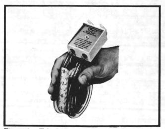
Figure 6 — Tube Manometer
