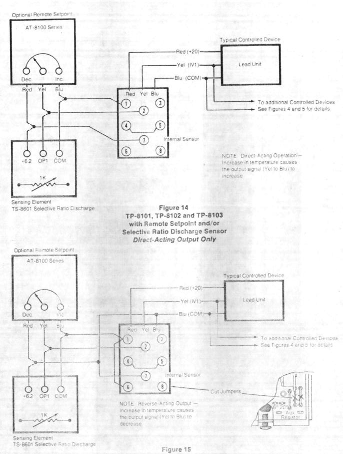
TP-8101, TP-8102 and TP-8103 with Remote Setpoint and/or Selective Ratio Discharge Sensor Reverse-Acting Output Only
