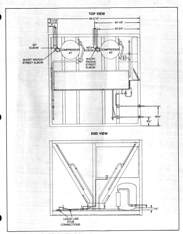
FIGURE 24 - Piping Installation: 40-Ton Units Without Isolators
