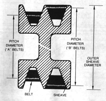
Figure 54 - Fan Sheave Pitch Diameter
