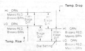
Figure 7. Two Stage Switch Sequence
