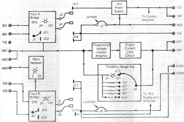
Figure 3. CP-8102 Controller Block Diagram
