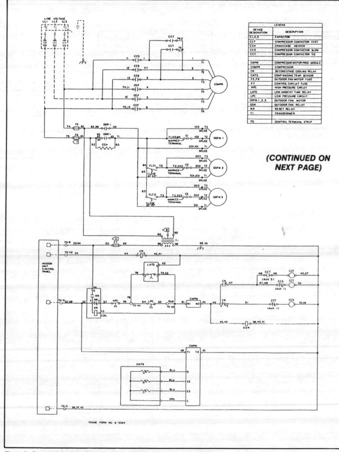
Figure 2 - Typical Unit Wiring Diagram (15 Ton Single Compressor Unit Shown)
