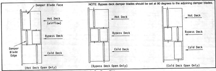
FIGURE 24B - Proper Three-Deck Multizone Damper Blade Configuration
