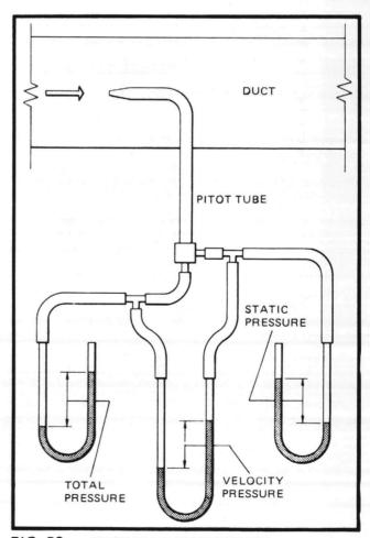
FIG. 32 - PITOT TUBE CONNECTIONS
