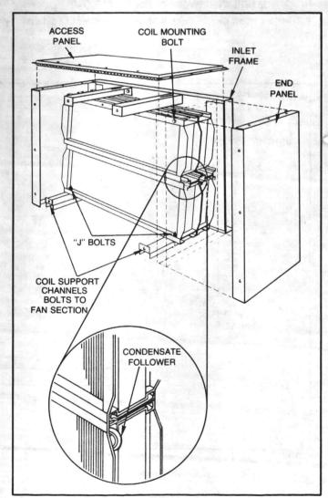
FIGURE 33B - Draw-Thru Unit Coil Section Details with View of Condensate Follower
