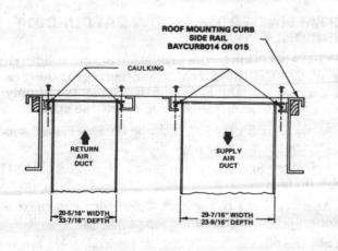
FIELD FABRICATED SIDE BY SIDE DUCTS INSTALLED FROM ABOVE CURB
