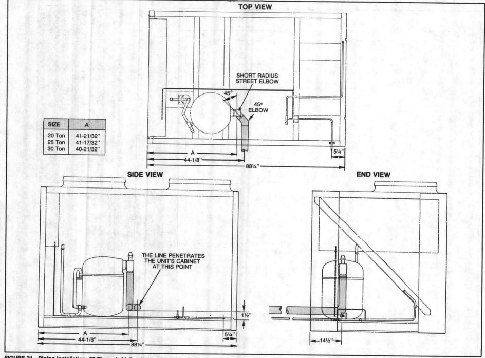
FIGURE 21 - Piping Installation: 20 Through 30-Ton Units Without Isolators
