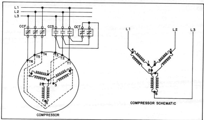
Figure 3 - High Speed Operation (Parallel Connected)
