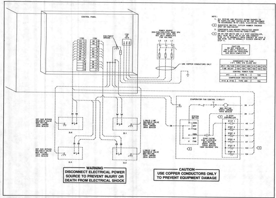
FIGURE 31 - Field Wiring, Multi-Step Controls, (40, 50 and 60-Ton Units)
