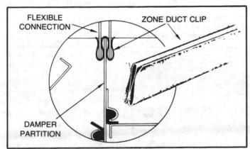
FIGURE 30 - Zone Duct Clip Installation
