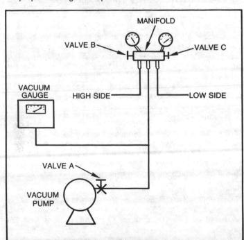
FIGURE 42 - Vacuum Pump Hook-up
