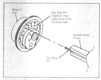
Figure 5. Dial Stop Pin Insertion
