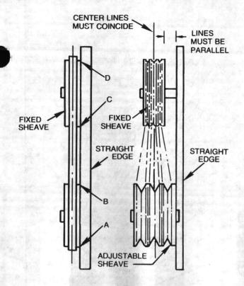
Figure 53 - Sheave Alignment
