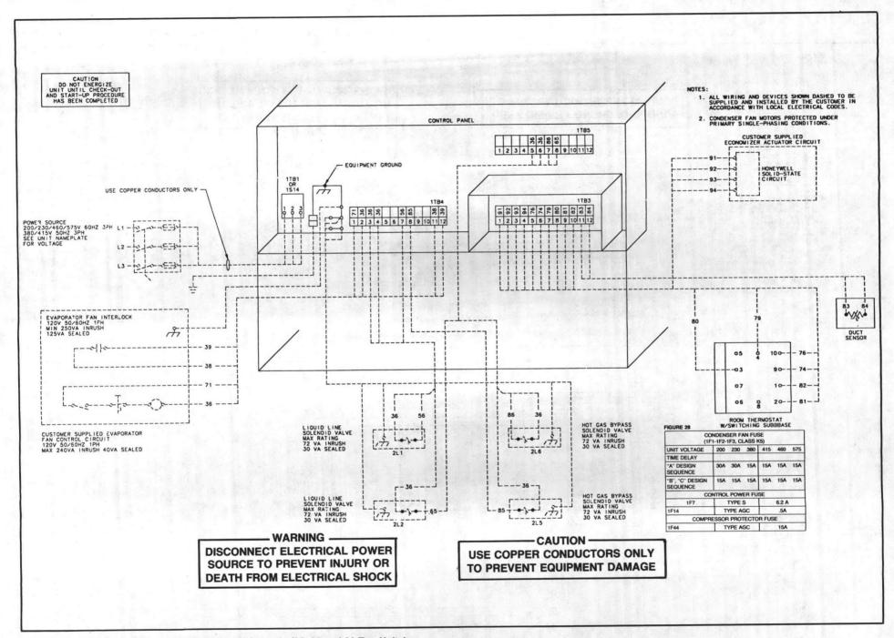
FIGURE 28 - Field Wiring, Electronic Thermostat Controls (20, 25 and 30-Ton Units)
