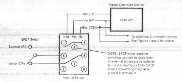
Figure 12. TP-8101, TP-8102 and TP-8103 with Single Pole Double Throw (SPDT) Winter-Summer Switching
