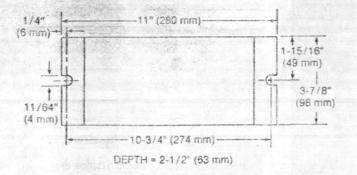
Figure 4. Mounting Dimensions
