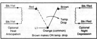
Figure 1. Switch Action and Lead Identification
