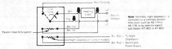
Figure 6. Typical of Parallel Heat Anticipation (heater size determined by voltage) with or without Night Depression
