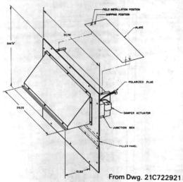
NOTE: Make sure that all screws are tight, so that gasket forms a water tight seal.
