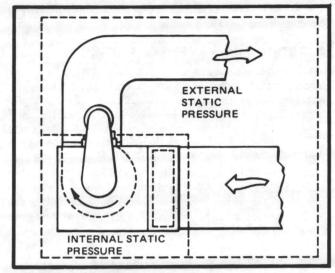
Figure 7 — Air Moving System
