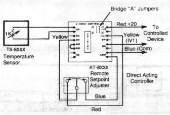
**NOTE:** If the controller bridge is reverse acting, the red and blue wires at the AT-8XXX Series must be reversed (red to common, blue to +6.2).
