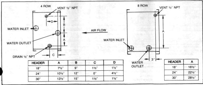
FIGURE 37 - Coll Type P8 Connections with Drain and Vent Locations (18", 24", and 30" Headers)
