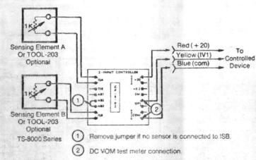
Figure 7. One or Two sensor Application
