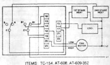
THERMOSTAT CYCLES HEAT & COOL, HEAT-COOL SWITCH, OFF-LOW-HIGH FAN SWITCH
