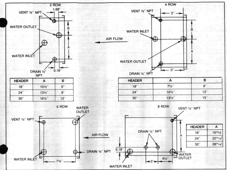
FIGURE 36 - Coil Type P4 Connections with Drain and Vent Locations (18", 24", and 30" Headers)
