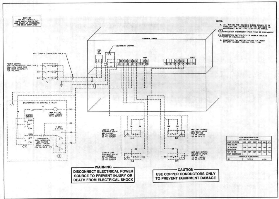
FIGURE 26 - Field Wiring, Two Step Controls (20, 25 and 30-Ton Units)
