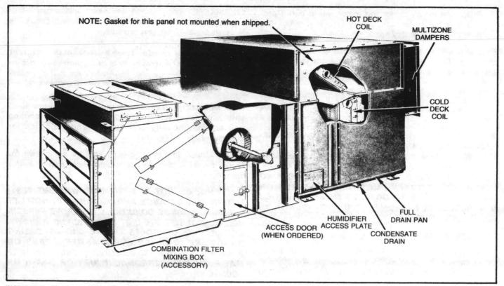
FIGURE 15 - Multizone Blow-Thru Climate Changers
