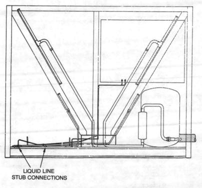
FIGURE 25 - Piping Installation: 50 and 60-Ton Units Without Isolators
