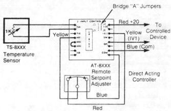
**NOTE:** If the controller bridge is reverse acting, the red and blue wires at the AT-8XXX Series must be reversed (red to common, blue to +6.2).
