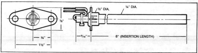
FIGURE 34 - Duct Sensor Dimensions
