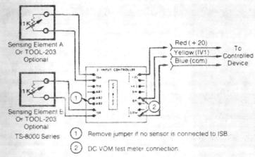
Figure 7. One or Two sensor Application
