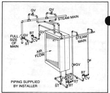
FIGURE 43 - Typical Piping for Type A Steam Colls, High Pressure, Vertical Tubes for Horizontal Airflow
