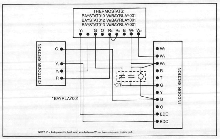
Figure 16 - Field Wiring for BTA120D With BTE120B Air Handler BTA-IN-5
