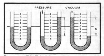
Figure 5 — "U" Tube Manometers
