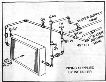
FIGURE 48 - Typical Piping for Type W or WA, 1-Row Water Coil
