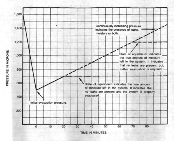
FIGURE 43 - Time Vs. Pressure Rise After Evacuation
