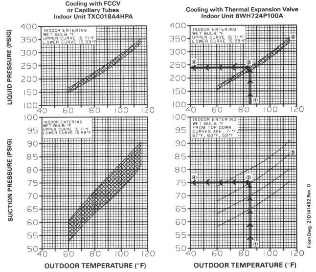
COOLING PERFORMANCE TO BE CHECKED WHEN OUTDOOR TEMP. IS ABOVE 75°F. HEATING PERFORMANCE CAN BE CHECKED WHEN THE OUTDOOR TEMP. IS BELOW 60°F.
