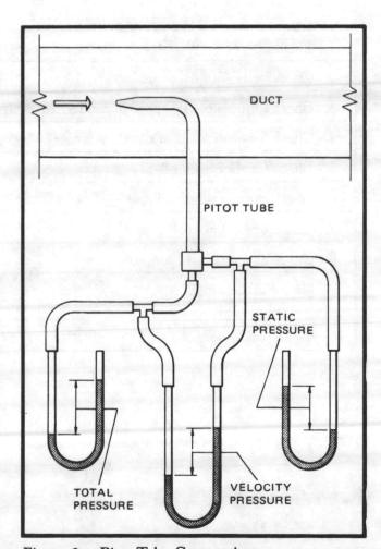
Figure 2 — Pitot Tube Connections
