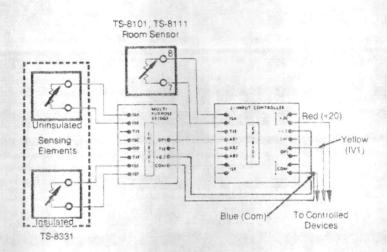
Figure 11. Derivative (Lagged) Sensor
