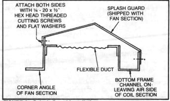
FIGURE 8 - Splash Guard Installation
