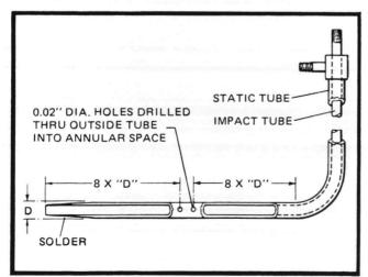
FIG. 31 — CONSTRUCTION OF PITOT TUBE
