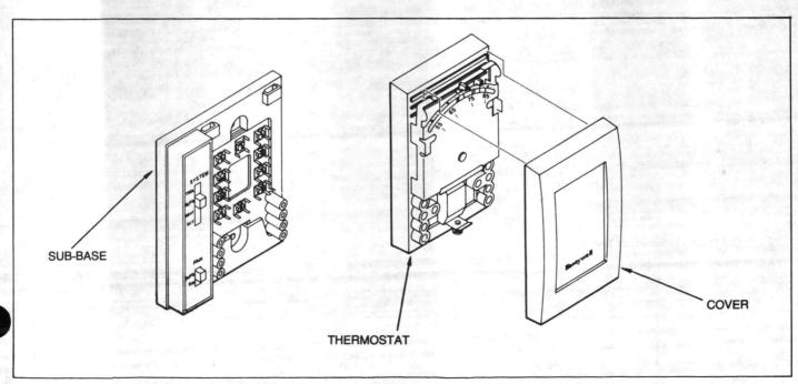
FIGURE 36 - Honeywell Electronic Thermostat With Switching Sub-base
