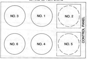
FIGURE 38 - Condenser Fan Sequence
