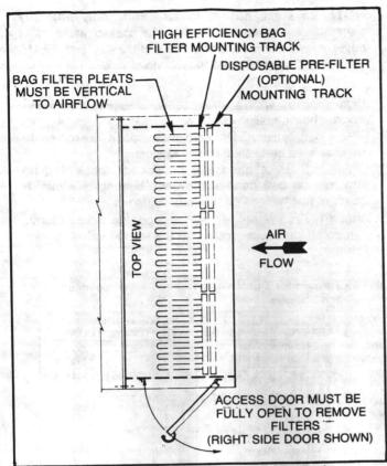
FIGURE 21 - Filter Mounting Track Location (Top View)
