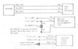
Figure 6. At Least One of the Controlled Devices in MP-52XX (Unfiltered)
