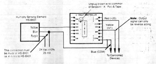
Note: Settings of 2-6 throttling range result in 2-6% RH throttling range for 3 Vdc output change. 6 TR is maximum setting.
