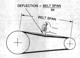
FIGURE 9 - Belt Tension Measurement
