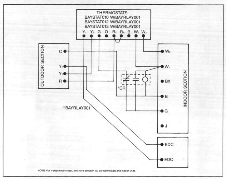
Figure 17 - Field Wiring for BTA150D, BTA180D and BTA180F With the BWV180B, BWH180F Air Handlers
