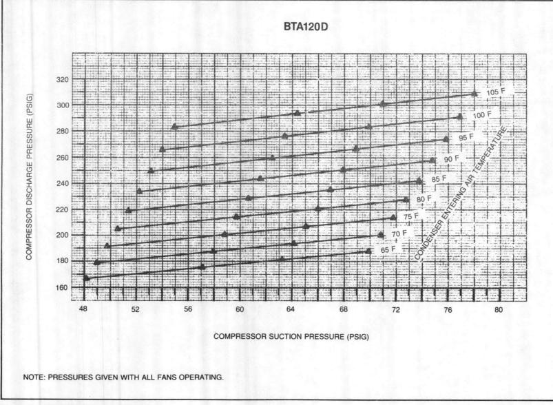
Figure 10 · BTA120D Operating Pressures
