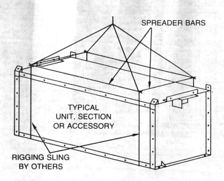
FIGURE 1 - Recommended Rigging Procedure
