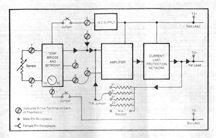
Figure 10 TP-8101, TP-8102 and TP-8103 Block Diagram
