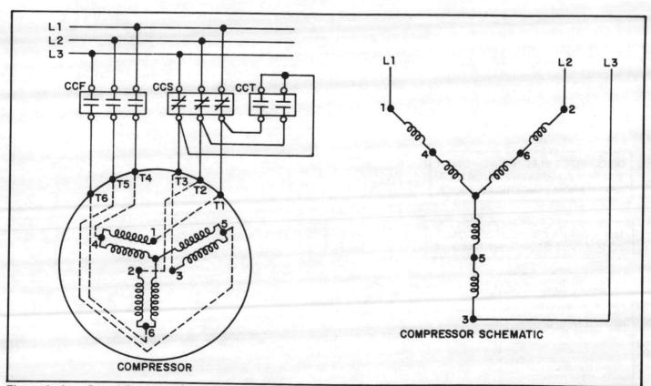
Figure 4 - Low Speed Operation (Series Connected)
