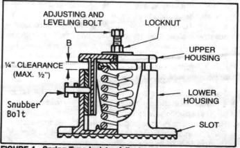
FIGURE 4 - Spring-Type Isolator Adjustment
