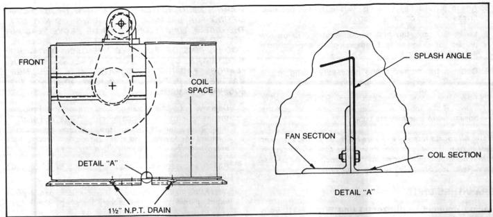
FIGURE 9 - Splash Angle Installation
