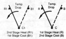
Note: Thermostat is designed for either heat or cool applications, not heat and cool.
