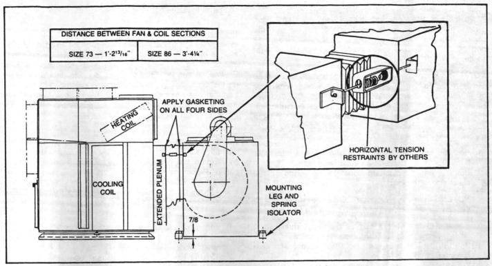
FIGURE 17 - Fan and Coil Section Ductwork Connections for Blow-Thru High Pressure Units
