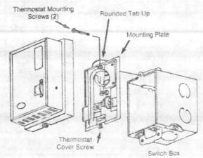
Figure 2. Thermostat Mounting
