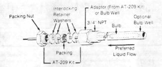
Figure 5. AT-201 or AT-203 Installation
