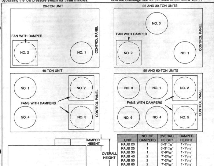
**FIGURE 40 - Low Ambient Dampers**
