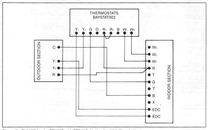
Figure 10 · Field Wiring for BTA120D with BTE120B Air Handler With Electric Heat
