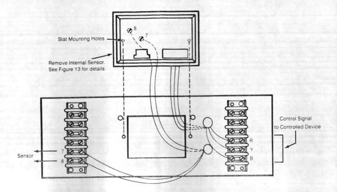
Figure 18 TP-8101, TP-8102 and TP-8103 Mounted on AD-8951
