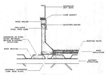
METHOD NO. 20 UNIFORMLY SUPPORTED OVER SHIMMED ROOF DECKING
