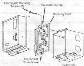
Figure 2. Thermostat Mounting
