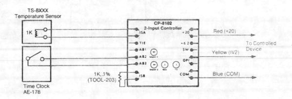
Install 1000 ohm 1% (TOOL-203) resistor in ISB. Install AE-178 7 day time clock. Set setpoint "B" as desired for night setback.
