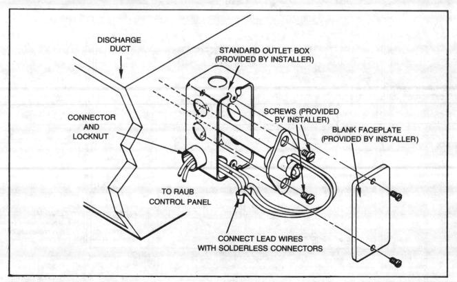
FIGURE 35 - Duct Sensor Assembly
