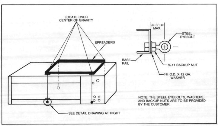
Figure 6 - Rigging the Unit
