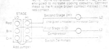
Two Compressor Packages May Be Sequenced With The Wiring Show
