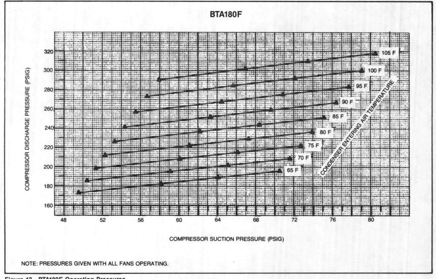
Figure 13 - BTA180F Operating Pressures
