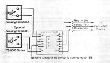
Figure 10. One or Two Temperature Sensor Application
