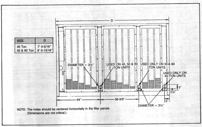
FIGURE 22 - Suction Line Hole Locations: 40 Through 60-Ton Units Without Isolators
