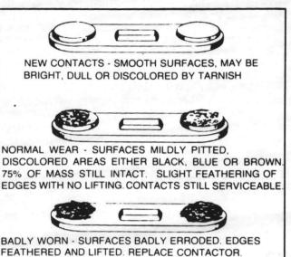
Figure 6 - Compressor Contactor Replacement Guide
