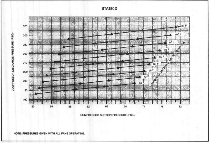
Figure 12 · BTA180D Operating Pressures
