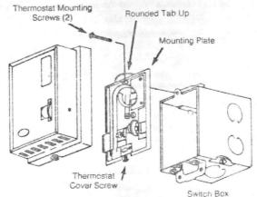
Figure 2. Thermostat Mounting
