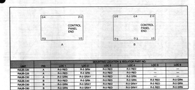
FIGURE 11 - Isolation Pad Selection and Location
