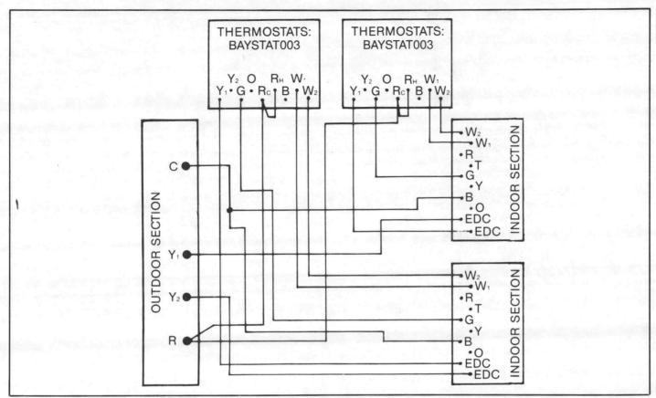
Figure 11 - Field Wiring for BTA150D and BTA180D With Two (2) BWE090C Air Handlers With Electric Heat
