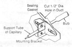
Figure 3. Duct Mounting with AT-208
