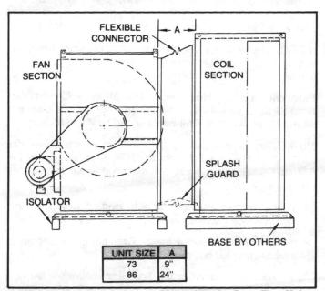
FIGURE 7 - Mounting Clearance Dimensions for Draw-Thru Units Sizes 73-86
