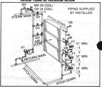
FIGURE 44 - Typical Piping for Type A or N Steam Coils, Horizontal Tubes for Horizontal Airflow
