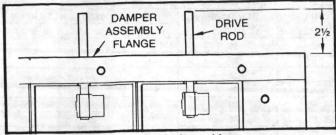
FIGURE 23 - Zone Damper Blade Assembly
