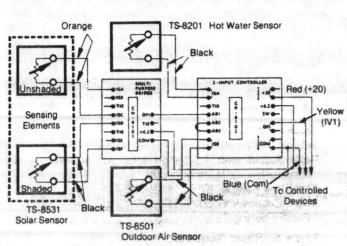
Figure 13. Solar and Outdoor Air Reset of Hot Water (Direct Acting Output)
