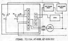
THERMOSTAT CYCLES HEAT & COOL, HEAT-COOL SWITCH, OFF-LOW-HIGH FAN SWITCH
