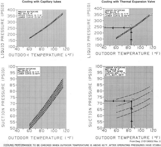
COOLING PERFORMANCE TO BE CHECKED WHEN OUTDOOR TEMPERATURE IS ABOVE 65°F. AFTER OPERATING PRESSURES HAVE STABILIZED: MEASURE INDOOR WET BULB TEMP - OUTDOOR TEMP - LIQUID & SUCTION PRESSURES. LOCATE OUTDOOR TEMP ① LOCATE INDOOR WET BULB ② FIND INTERSECTION OF OD TEMP & ID W.B. ③ READ LIQUID OR SUCTION PRESSURE IN LEFT HAND COLUMN ④
