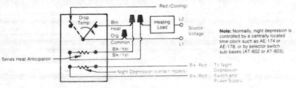
Figure 7. Typical of Series Heat Anticipation (heater size determined by ampere rating of load) with or without Night Depression
