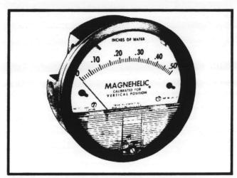
FIG. 34 - MAGNAHELIC PRESSURE GAUGE
