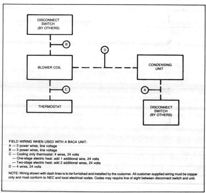
Figure 8 - Electrical Connections by Customer
