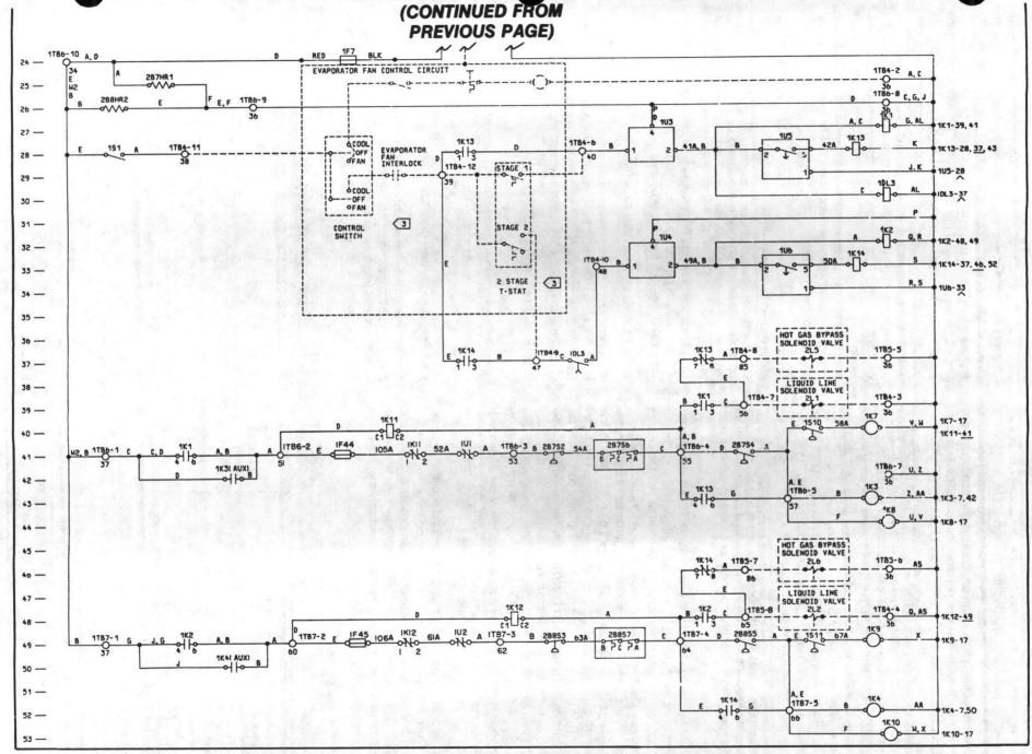
FIGURE 39 - System Wiring Diagram, 40, 50 and 60-Ton Units, Across-the-Line Start, 460/60/3, 2-Step Control
