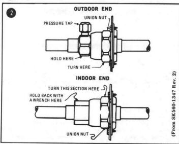
5. Advance the union nut another 1/4 turn. This final turn is necessary to insure a proper metal seal of the coupling halves, forming a leak-proof joint. Do NOT continue to tighten the coupling as distortion of the coupling nut will result in a leak.
