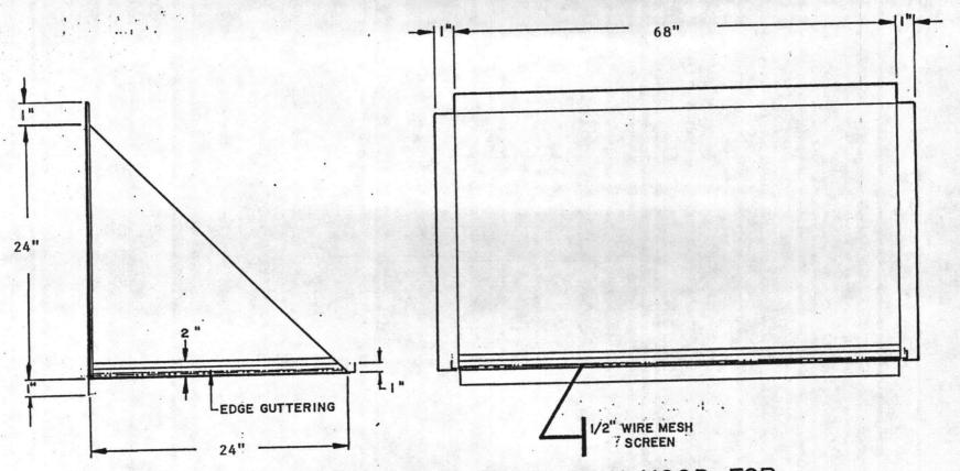
18 GA. GALV. STEEL RAIN HOOD FOR (x) OUTSIDE, () EXHAUST AIR
