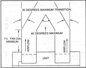
FIGURE 29 - Discharge Ductwork Recommendations for Two-Fan Units
