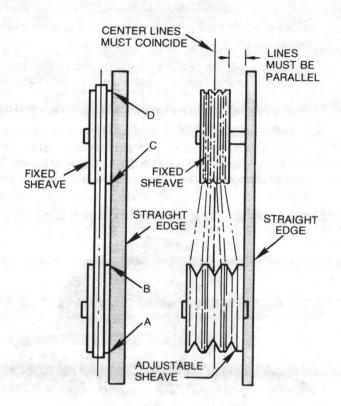
FIGURE 7 - Sheave Alignment
