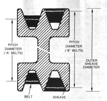
FIGURE 8 - Fan Sheave Pitch Diameter
