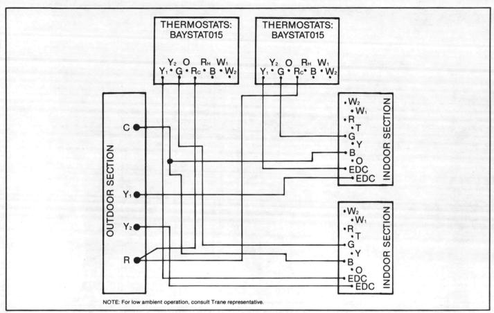
Figure 13 - Field Wiring for BTA150D and BTA180D With Two (2) BWE090C Air Handlers Without Electric Heat
