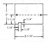
Figure 2. Field Supplied Duct Hole Cover Plate
