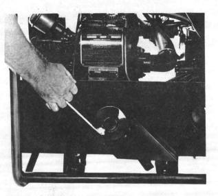
Figure 4-6. Use of Engine Starting Rope
