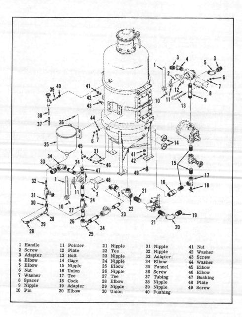
Fig 2-7. Exploded view of filter unit.
