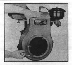
Fig 3-23. Winding of starting sheave.
