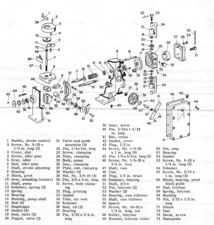
Figure 7-15. Hypochlorinator - Exploded
