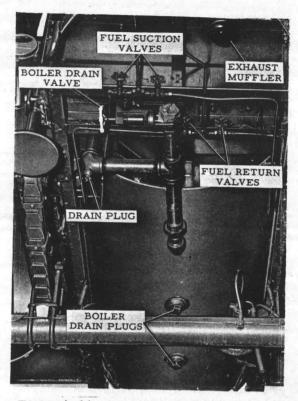
Figure 4-11. Bath unit, underneath view.
