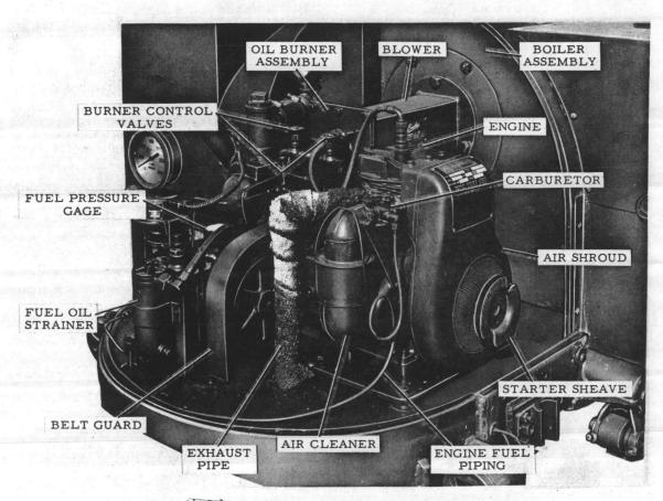
Figure 4-10 Operating components, right side view.
