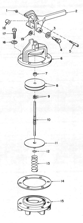
Figure 7-6. Air Release Valve - Exploded
