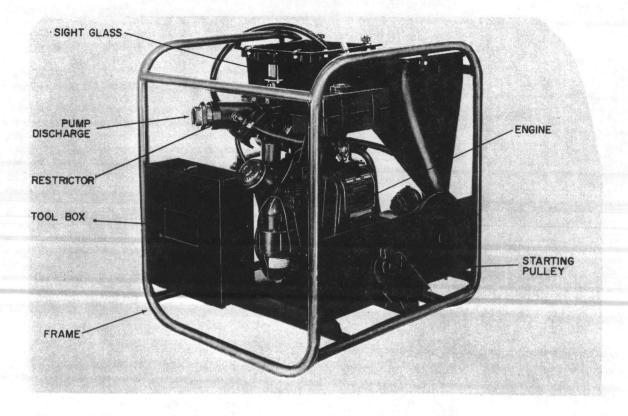
Figure 2-7. Machinery Section (Front View)
