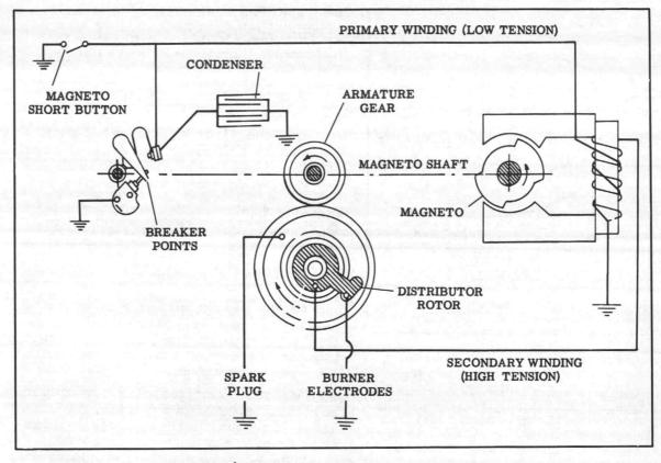
Figure 4-6 Engine and burner ignition system.
