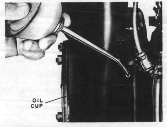
PUMP SHAFT SEAL: Daily (each 8 hours of operation) fill oil cup in pump seal area with SAE 10 oil.
