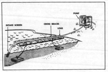
Fig 1-17. Float-type surface intake.
