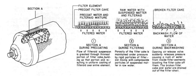
Figure 2-6. Filter Element With Section Removed
