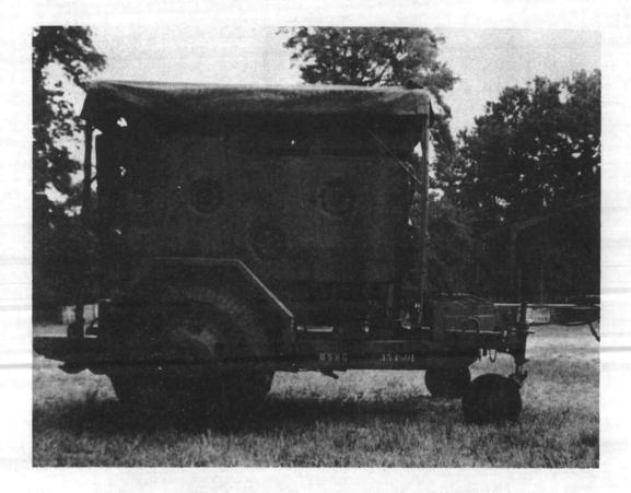
Fig 2-31. Distillation unit, 200-gph--side view.
