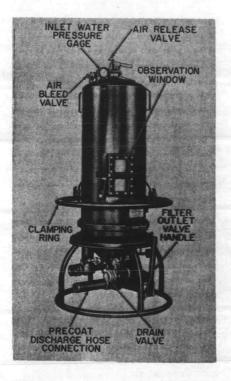
Fig 2-23. Filter section--front view.
