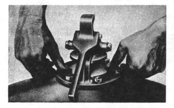
Figure 4-11. Air Release Valve -Positioned for Closing
