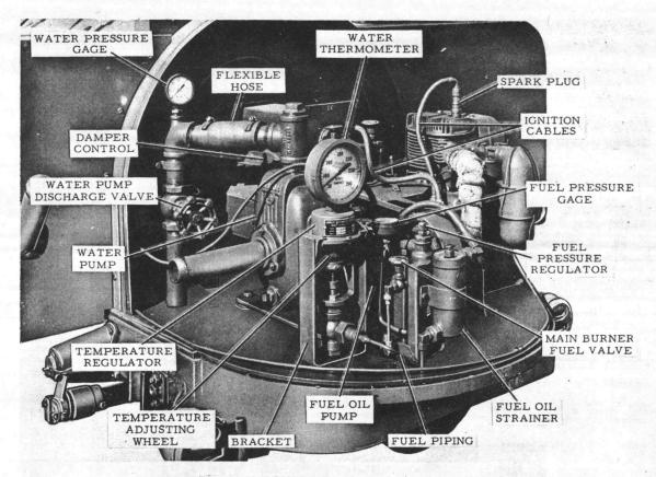
Figure 4-9 Operating components, left side view.
