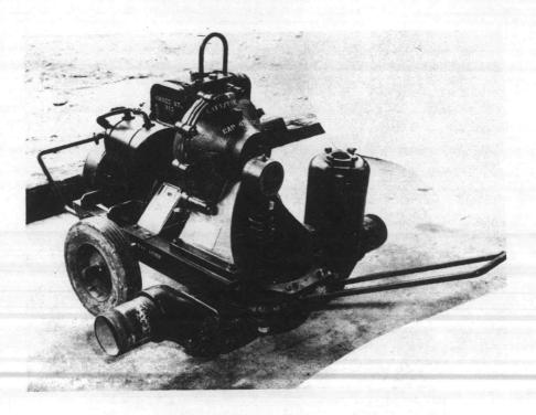
Fig 3-6. Pump, reciprocating, 100-gpm (Gorman - Rupp).
