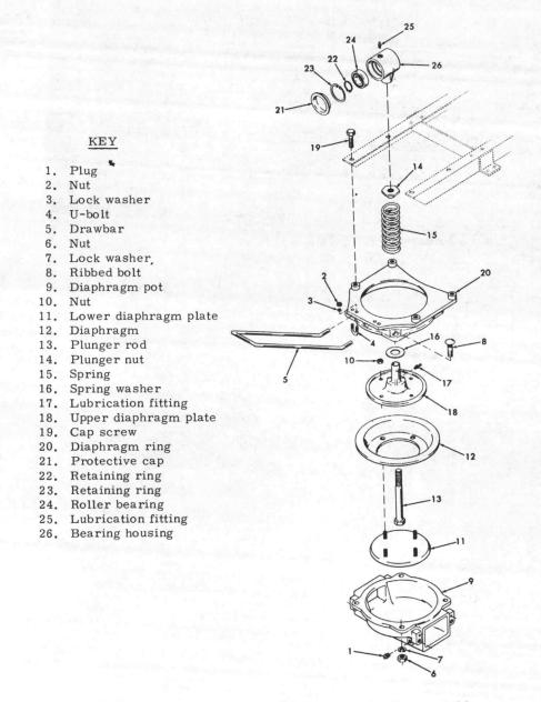
Fig 3-8. Diaphragm and plunger assembly.
