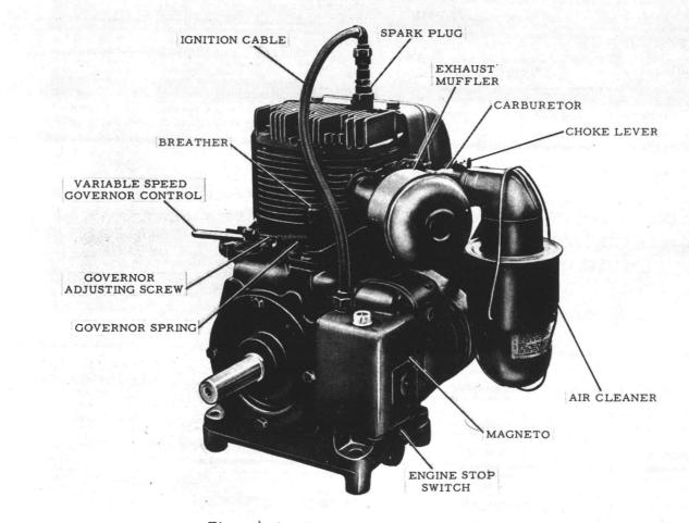
Figure 4-3. Gasoline engine, 3/4 view.
