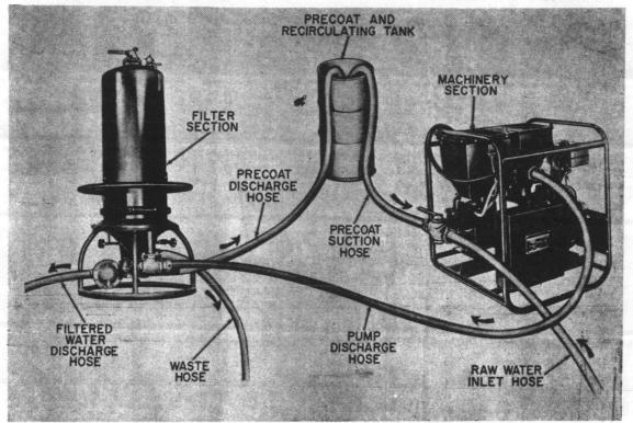
Fig 2-20. Water purification unit in operating position.
