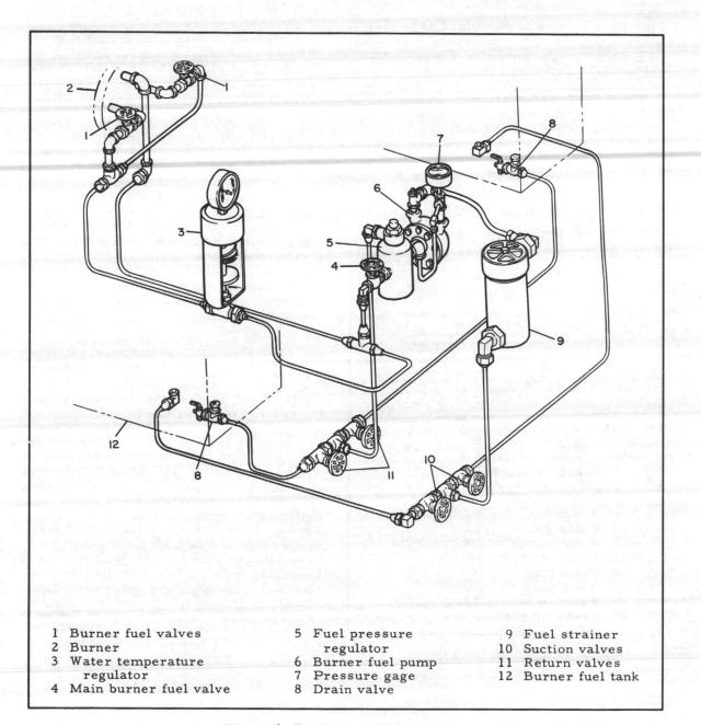
Figure 4-5 Burner fuel system.
