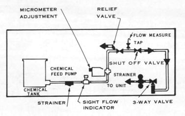
Fig 2-42. Chemical injection system schematic.
