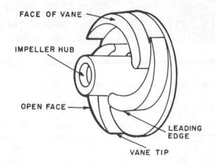
Figure 7-22. Pump Impeller Inspection
