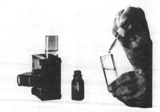
Figure 4-2. Installation of Comparator Prism
