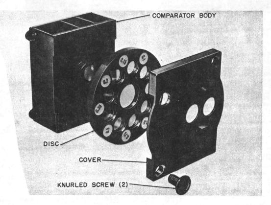
Figure 4-1. Installation of Comparator Disc
