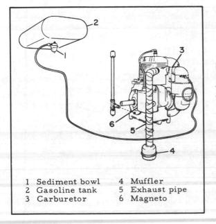
Figure 4-7 Engine fuel system.
