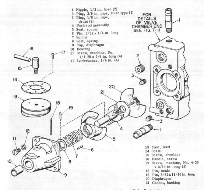
Figure 7-10. Mixing and Valve Chamber-Diaphragm End - Exploded
