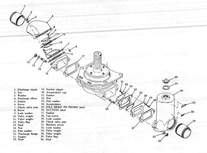
Fig 3-9. Pump assembly (suction and discharge sides).
