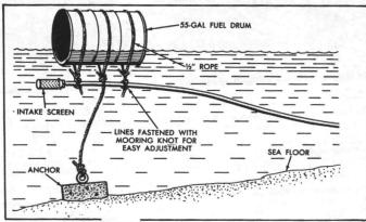
Fig 1-21. Float-type seawater intake.
