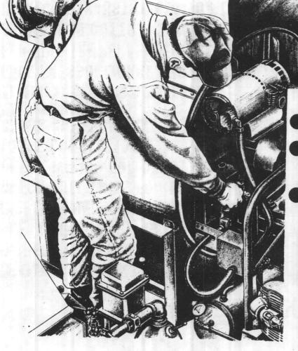
CLOSE AIR TANK DRAIN VALVE. PLACE ON-OFF SWITCH TO ON POSITION.
