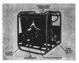
Fig 2-22. Machinery section -- rear view.
