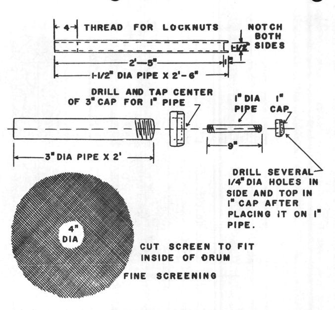
The urinoil may be improvised from a 55-gallen drum as shown in the drawing. The urinoil should be placed on a soakage pit when possible, or installed with a French drain.
