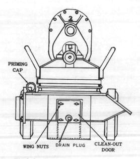
Fig 3-4. Pump body clean-out door.
