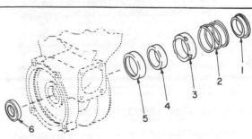
Figure 7-21. Details of Seal Ring Assembly
