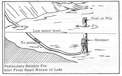
Fig 1-13. Direct intake with hose on bottom of water source.
