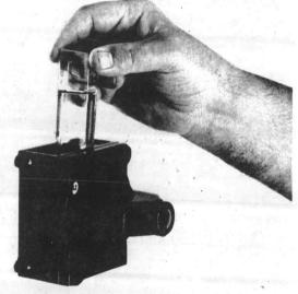
Figure 4-4. Insertion of Second Sample Tube
