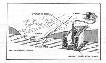
Fig 1-18. Gravel-filled gallery intakes.
