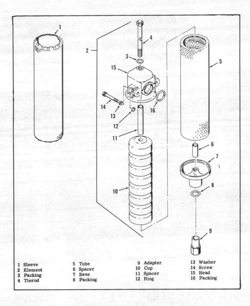
Fig 2-8. Exploded view of filter element.
