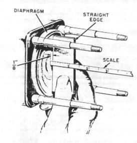
Figure 7-16. Hypochlorinator Diaphragm Adjustment
