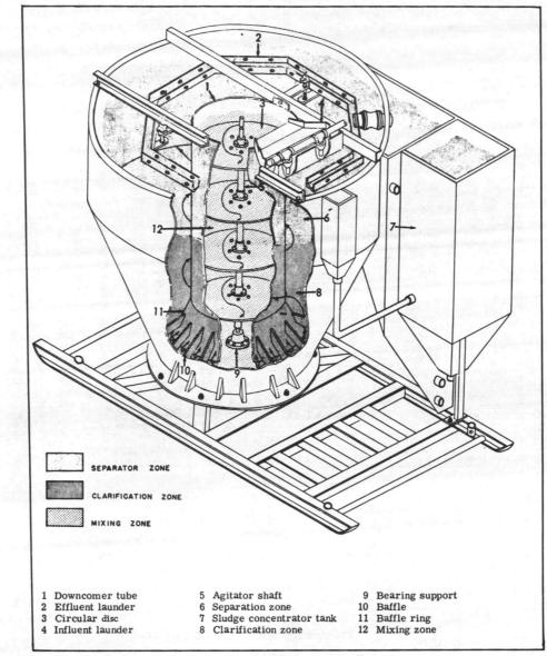
Fig 2-3. Cutaway view of erdlator.
