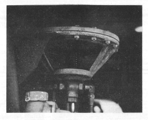
Fig 2-41. Automatic, water-bypass valve
