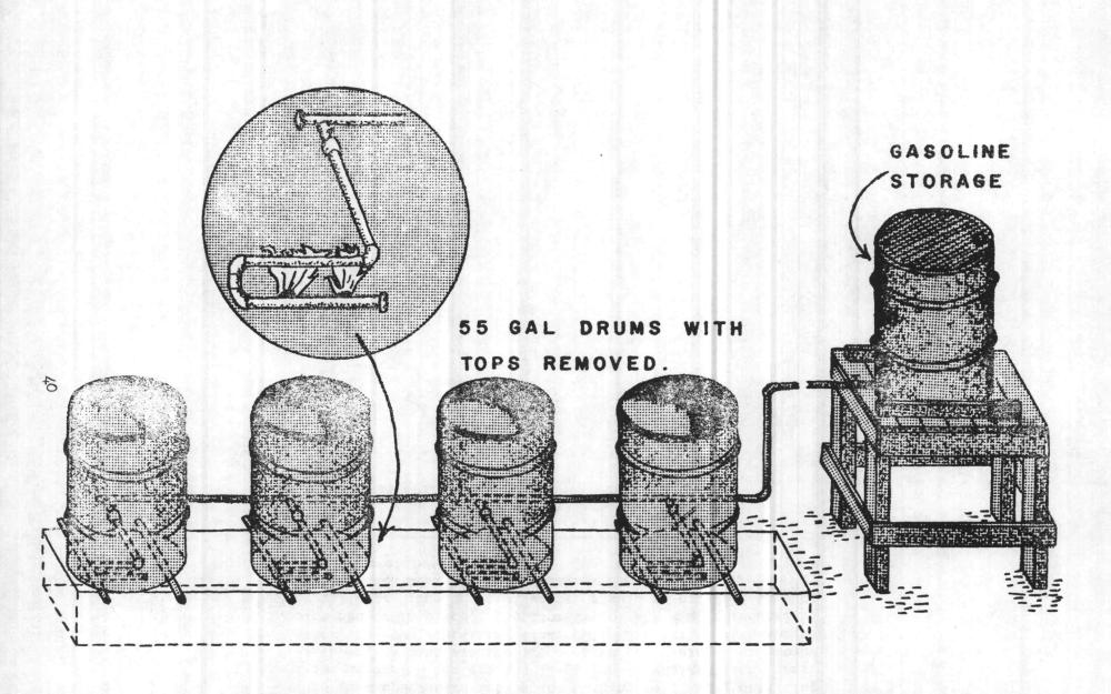
MESS KIT WASHING SET-UP VAPOR BURNER
