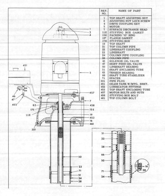
Fig 3-27. Above ground enclosed line shaft pump base.
