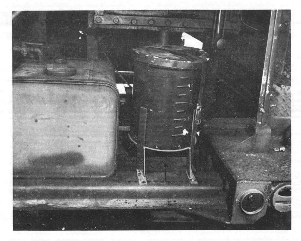
Fig 2-44. Chemical injector, 5-gallon supply tank.
