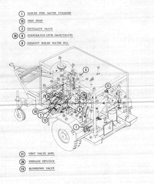
Fig 2-33. Distillation unit.
