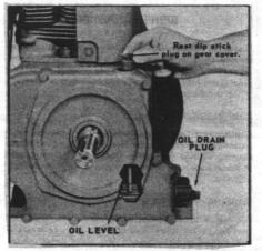
Fig 3-20. Dipstick and drain plug location.
