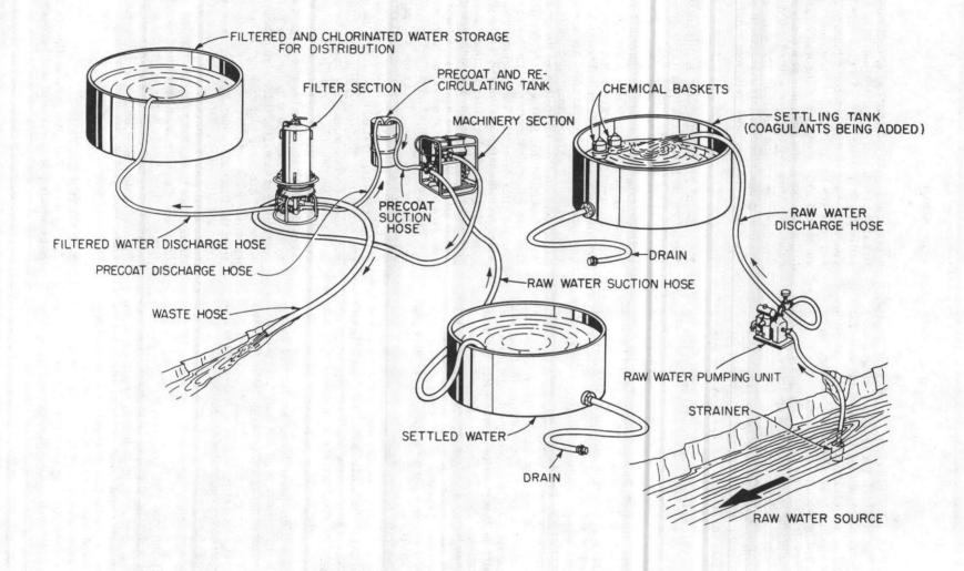
Figure 2-1. Typical Arrangement of Water Purification Equipment
