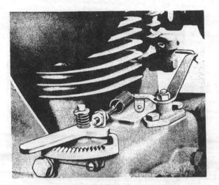
Figure 4-7. Engine Speed Governor Control
