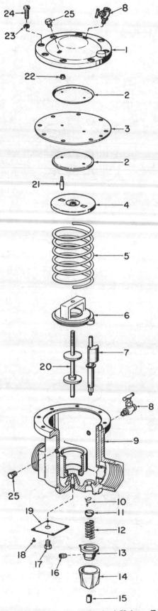
Figure 7-7. Adjustable Flow Control Valve - Exploded
