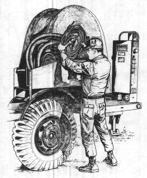
STOW FUEL DRUM ADAPTERS, GROUND ROD, AND CABLE ASSEMBLY INSIDE 7" DUCT.
