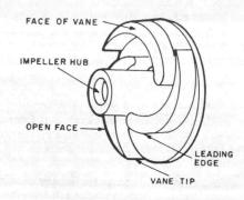
Fig 3-13. Pump impeller.
