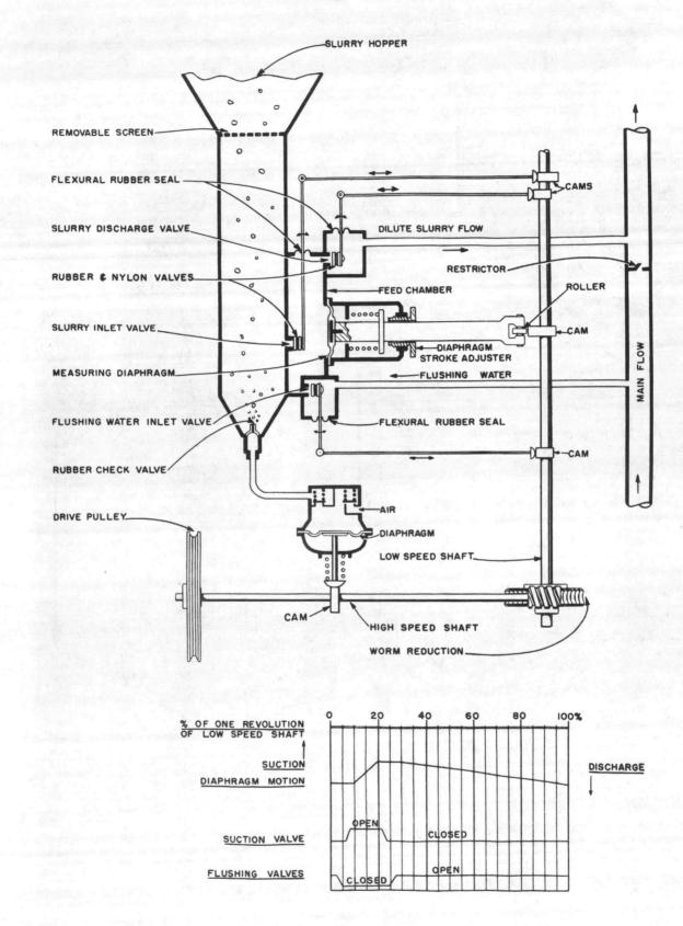
Figure 7-8. Slurry Feeder Operation - Schematic and Sequence Diagram
