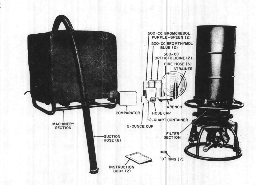
Figure 1-1. Water Purification Unit.
