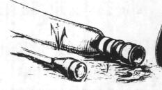
DISCONNECT SUCTION AND OUTLET HOSE AT WATER PUMP AND OPEN PETCOCK DRAIN.
