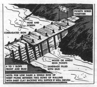
Fig 1-15. Improvised dam for impounding small streams.
