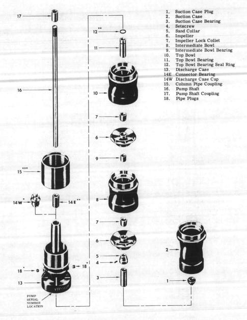
Fig 3-31. Pump bowl assembly--exploded view.
