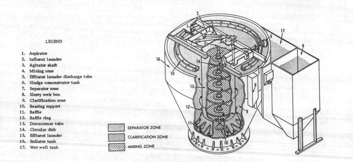
Fig 2-14. Erdlator assembly-cutaway view.
