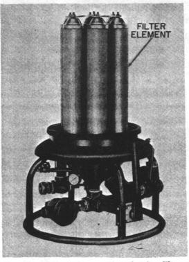
Fig 2-25. Dismantled filter section showing filter elements.
