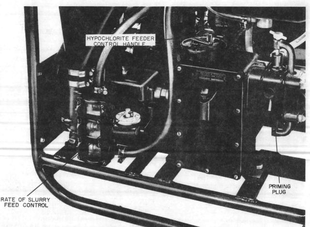
Figure 4-10. Slurry Feeder and Hypochlorinator Controls
