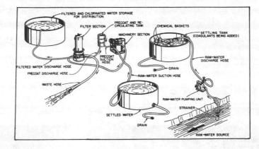
Fig 2-26. Typical arrangement of water-purification equipment.
