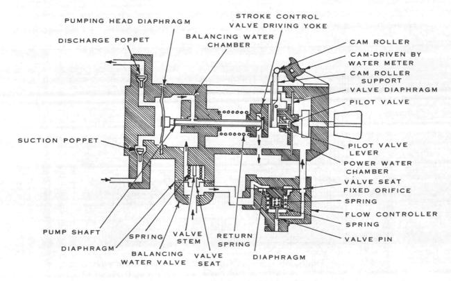
Fig 2-28. Operation of equipment.
