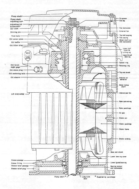
Fig 3-24. Typical vertical hollow-shaft motor.
