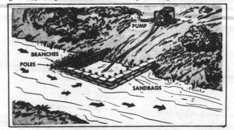
Fig 1-16. Baffle dam for protecting inlet strainer.
