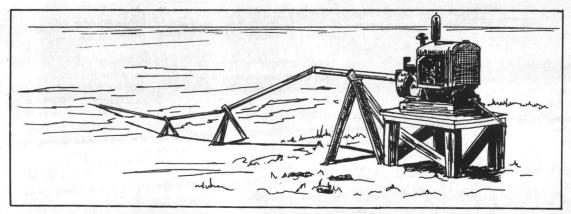
Fig 1-20. Rigid-pipe type seawater intake.
