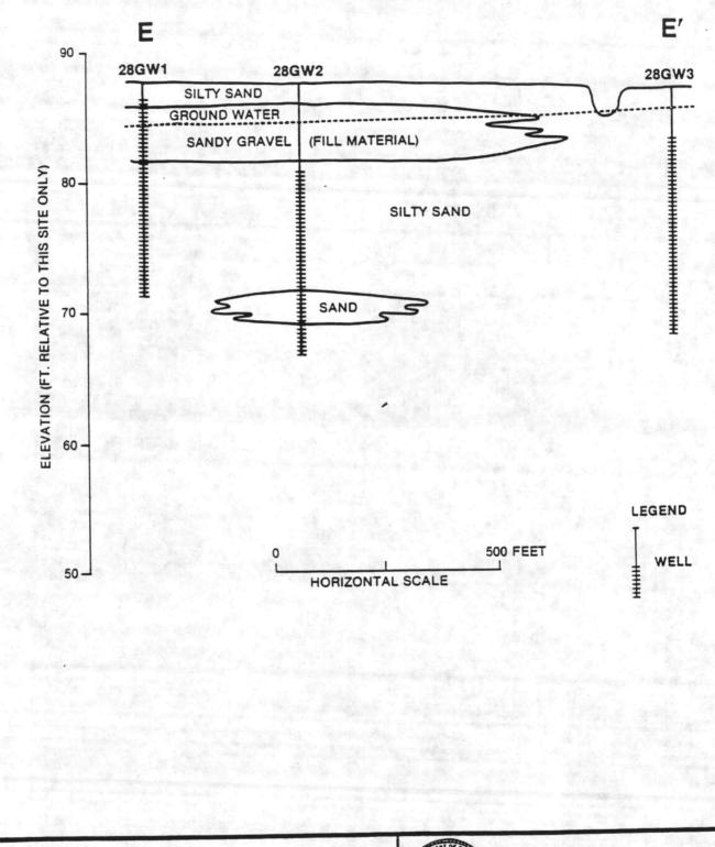
Figure 28-2 GEOLOGIC CROSS SECTION, SITE 28— HADNOT POINT BURN DUMP
