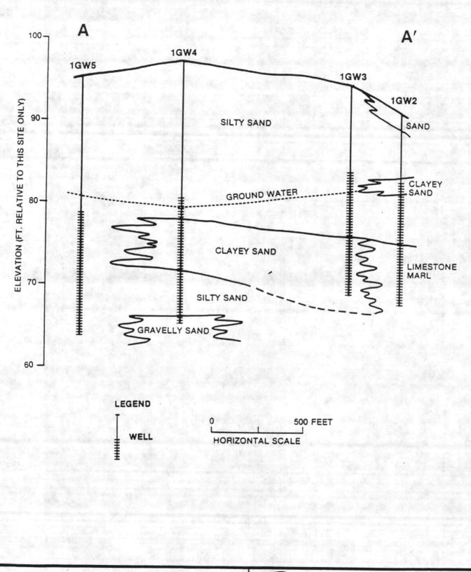
igure 1-2 GEOLOGIC CROSS SECTION, SITE 1-FRENCH CREEK LIQUIDS DISPOSAL AREA
