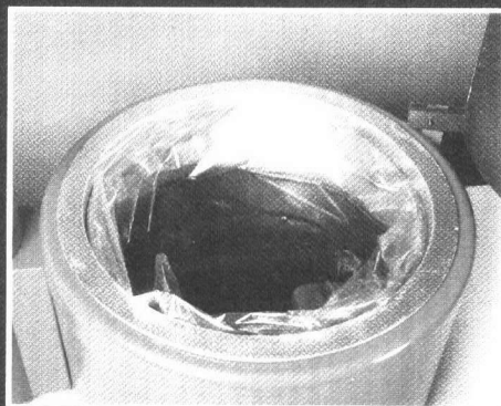
Contaminated solvent in STILBAG-lined vessel ready for startup
