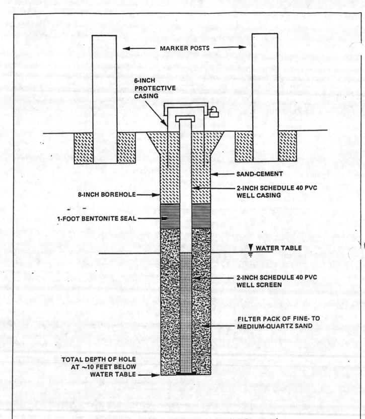
FIGURE A-1. Recommended Monitoring-Well Construction
