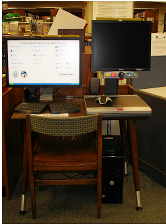
Figure 2: Example of an Accessible Workstation, with Desktop Magnifier.
