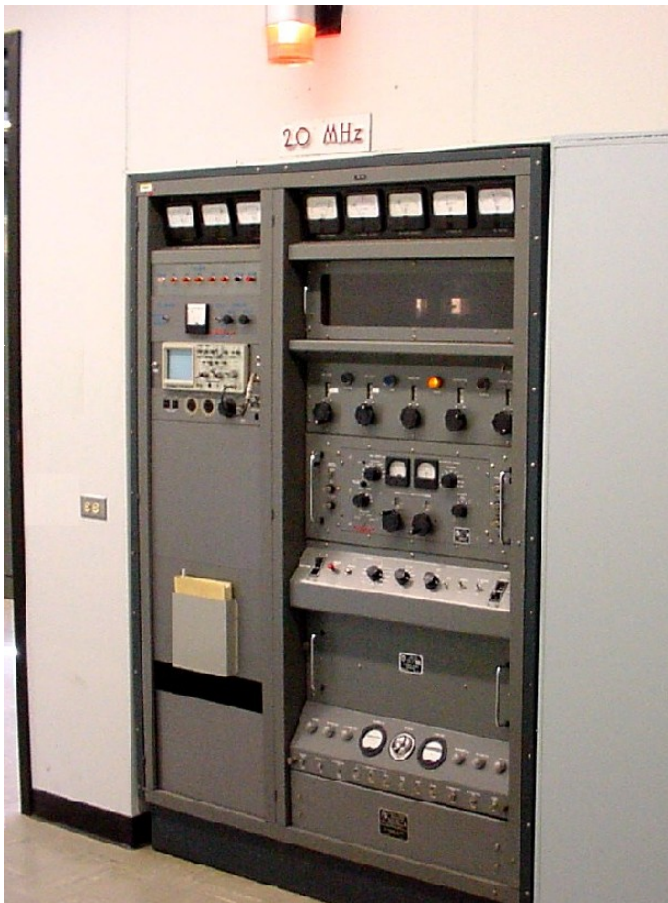
Figure 1.7. The 20 MHz transmitter at WWV.
