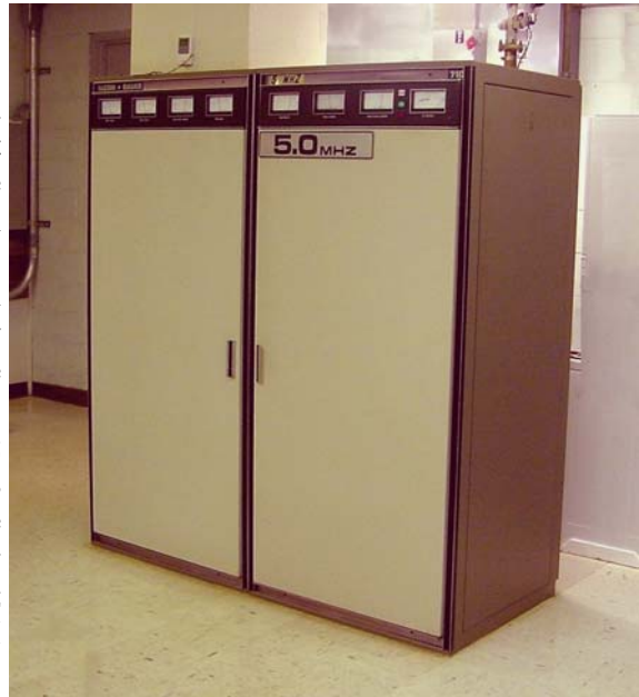
Figure 1.25. The 5 MHz transmitter at WWVH.
