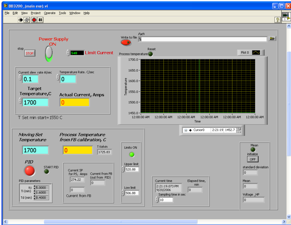
Figure Irr5.2. Front panel of the HTBB Control Program ( BB3200_(main.exe).vi )
