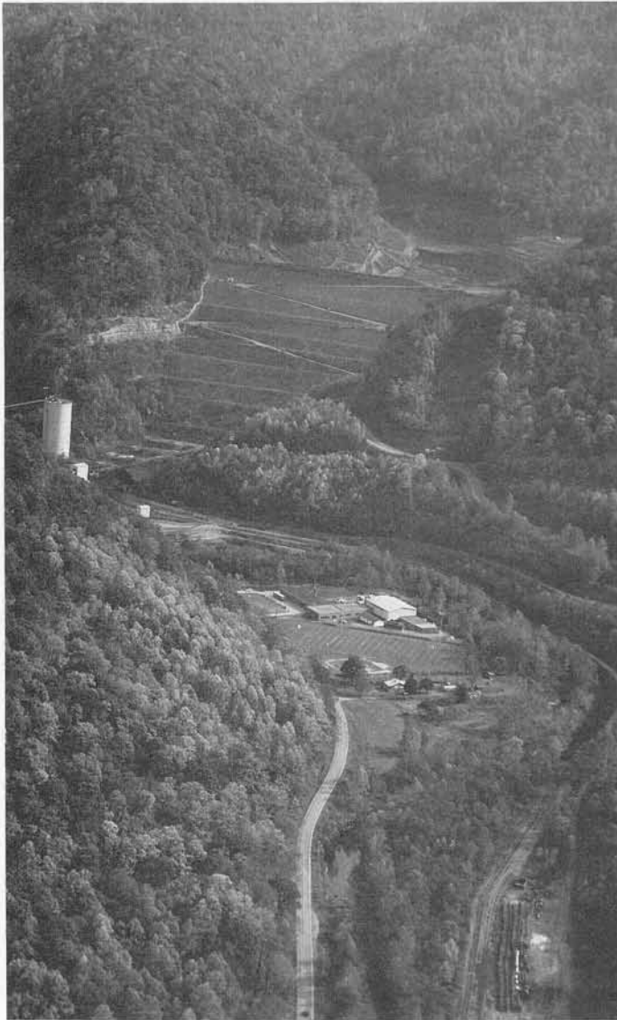
A slurry pond constructed on Shumate's Branch. "Slurry," the fine wet refuse from the coal cleaning process, is stored behind a dam engineered out of the coarse refuse. Though the dams are highly regulated, slurry has been elsewhere linked with severe flooding and "blowouts." "There's a saying around here," said one storekeeper. "We fear the river above more than the river below." In the foreground is the Marsh Fork Middle School. Photo by Lyntha Eiler
