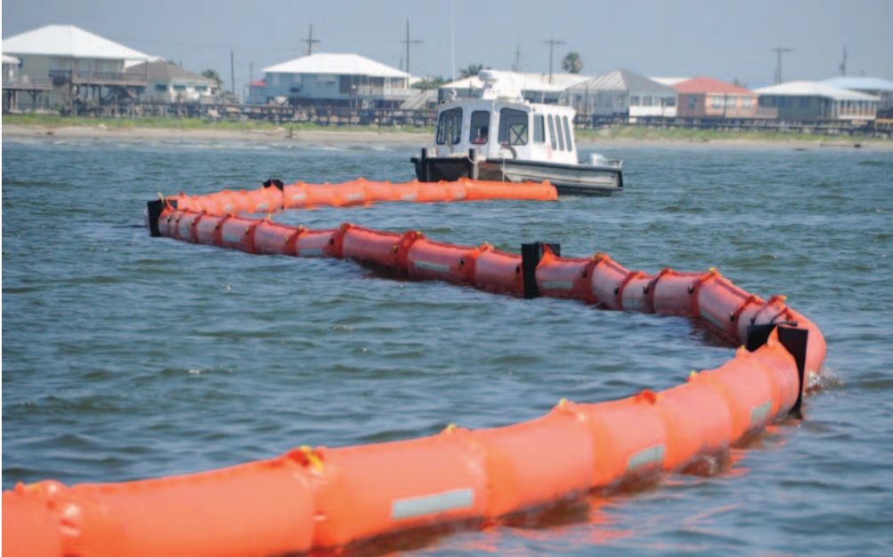
A vessel places containment boom in Louisiana's Barataria Bay. Hundreds of miles of boom were deployed along the Gulf coast, but politicians clamored for more of the highly visible barriers.
