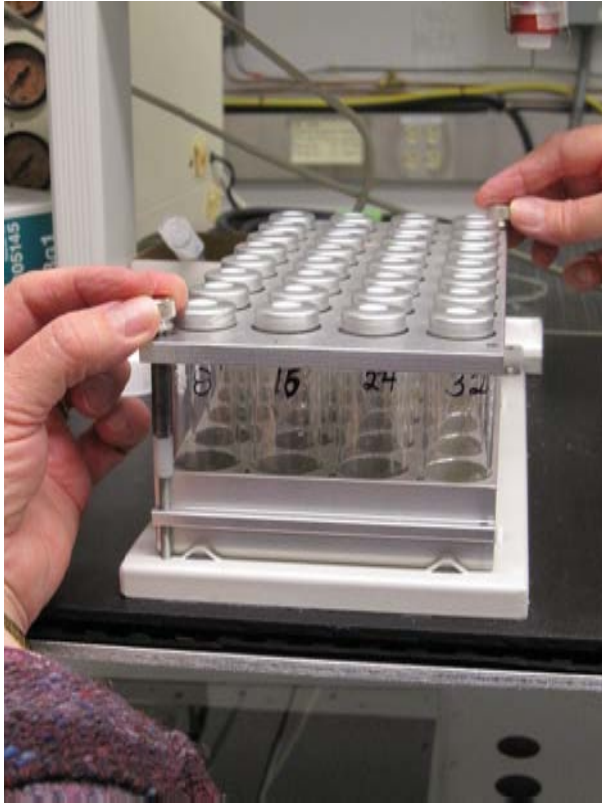
Figure C–19. Sample tray with 32 vials and a ¼-inch-thick aluminum plate to secure vials.
