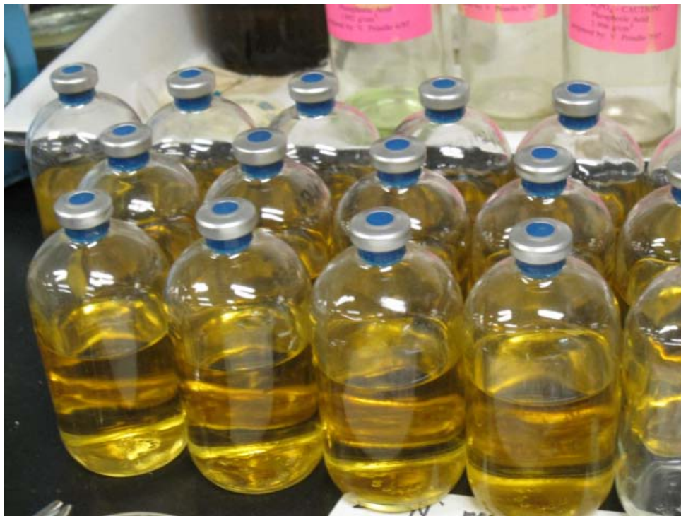
Figure C-4. Tryptic Soy broth (TSB) without \text{KNO}_3 , prepared with 100-mL aliquots in 125-mL serum bottles.
