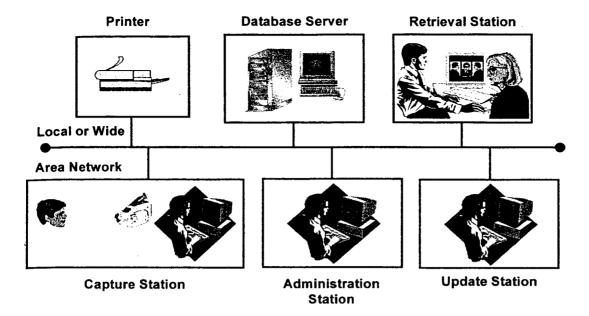
In smaller implementations, a site may choose to just use a single workstation for retrieval, updates, and administration. The capture station differs from other components since its configuration includes a digital camera.
