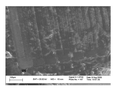
Figure 4. SEM image of a float glass sample following analysis by LA-ICP-MS using the rastering technique. The raster pattern can be seen in the image.
