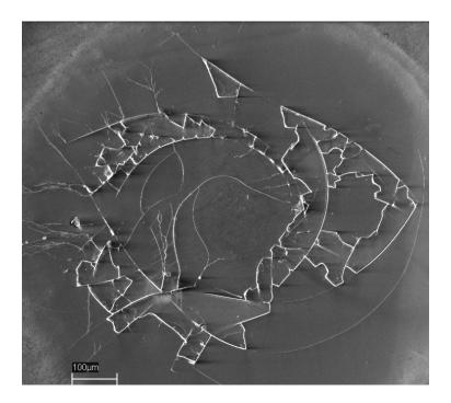
Figure 2. SEM image of the burn pattern and minimal destruction from a single LIBS event initiated by a 1064 nm laser pulse impinging on a float glass surface.
