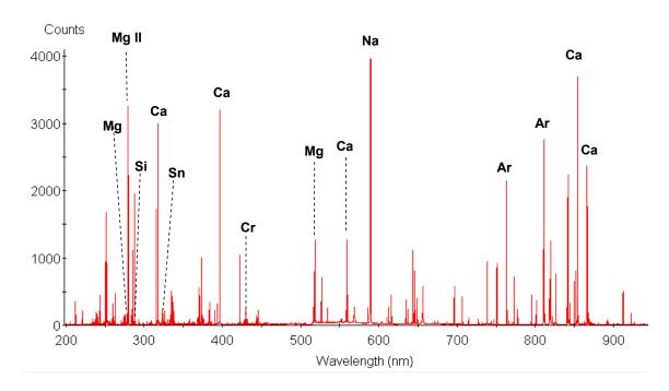
Figure 3. Typical LIBS spectrum of a float glass sample.
