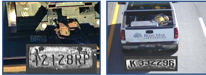
Figure 11: Bent, Dirty, or Damaged Plates
