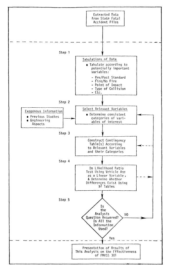
Figure 3-6 Proposed Statistical Analysis Scheme for analyzing fire-related fatal automobile accidents.
