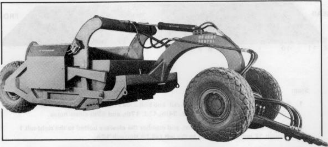
Figure 2-1. Murray model, towed, 7 1/2-cubic-yard earthmoving scraper.
