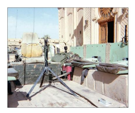
Figure K-10. Unit-produced tripod and modified armor.
