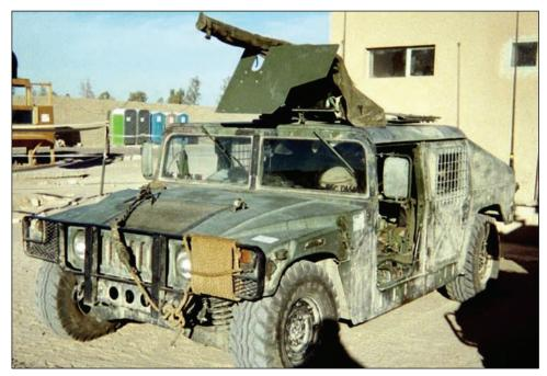
Figure K-1B. Army-issue, roof-mounted, gun-ring armor.
