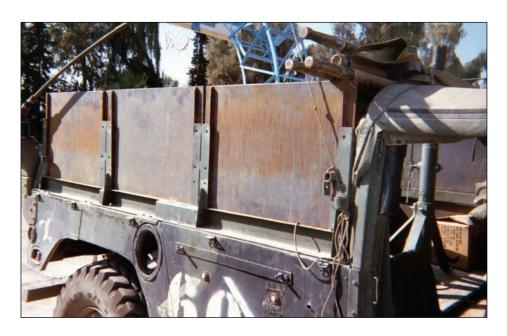
Figure K-12. Unit-installed steel armor.
