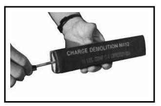
Figure 14-9. Priming of C4 demolition blocks with MDI.
