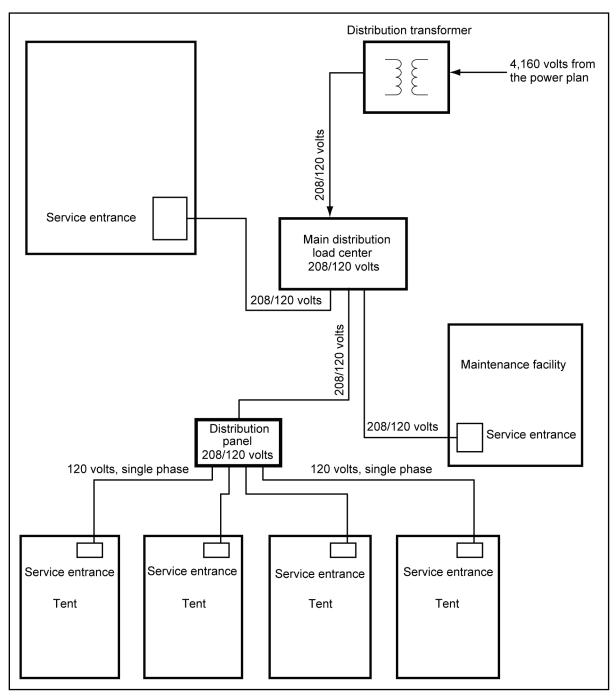
Figure D-6. Typical simple secondary distribution network
