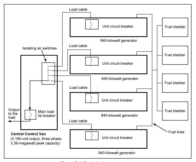
Figure D-1. Typical prime power plant
