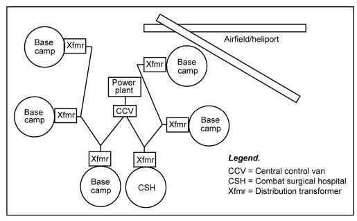
Figure D-2. Typical radial primary distribution network
