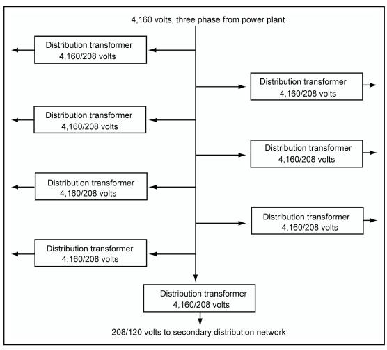
Figure D-4. Typical primary distribution feeder
