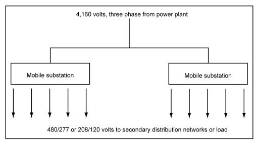
Figure D-5. Typical application of mobile substations
