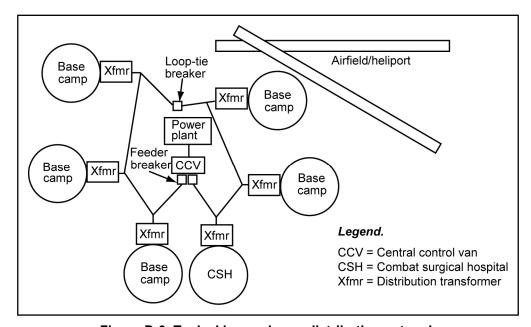
Figure D-3. Typical loop primary distribution network
