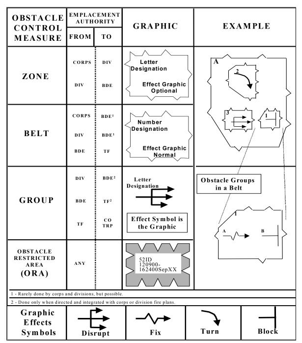
Figure 2-26. Obstacle Control Measure Graphics
