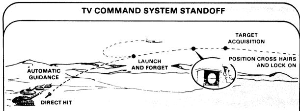
WHEN USING THE TV-COMMAND SYSTEM, THE PILOT DESIGNATES A TARGET TO THE SEEKER ON THE BOMB. THE SEEKER TRANSMITS THE TARGET IMAGE TO THE PILOT'S TV MONITOR PRIOR TO LAUNCH. THE BOMB LOCKS ONTO THE TARGET AND IS LAUNCHED. THE ELECTRO-OPTICAL BOMB HOMES AUTOMATICALLY ONTO THE DESIGNATED TARGET WHILE THE AIRCRAFT ESCAPES WITHOUT HAVING TO FLY OVER THE TARGET. THE ILLUSTRATION SHOWS THE TYPICAL SEQUENCE OF A TV-COMMAND SYSTEM.
