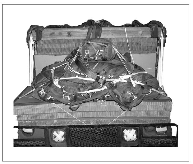
Figure 4-17. Deployment Parachute Installed
