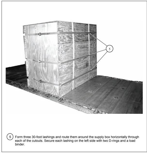
Figure 8-3. Supply Box Positioned (Continued)
