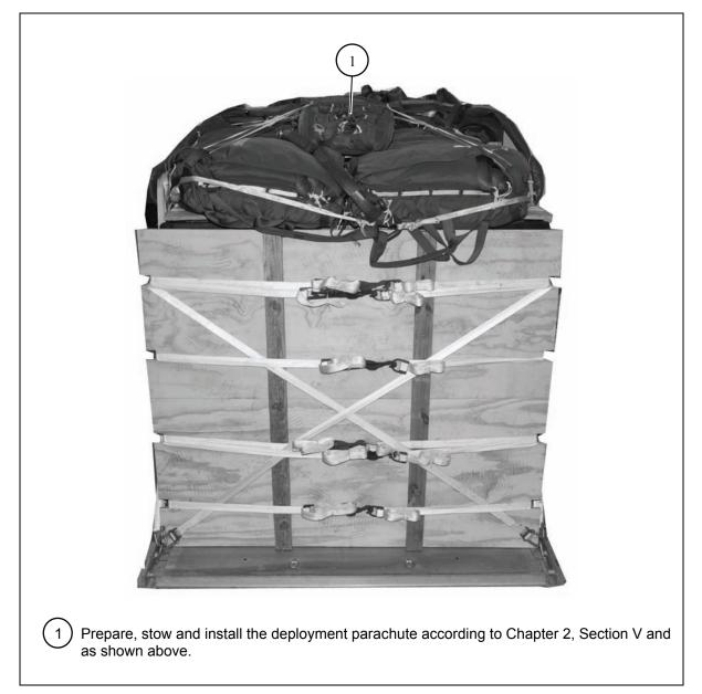
Figure 8-29. Deployment Parachute Installed
