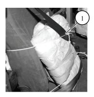
Remove the side view mirrors and wrap with cellulose wadding and tape. Secure them to the front passenger seat with type III nylon cord. Fasten the seat belt around the padded mirrors.
