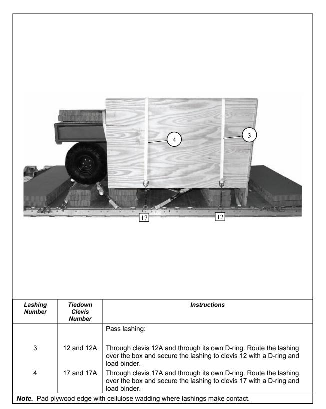
Figure 10-13. Lashings 3 and 4 Installed on M-Gator Box
