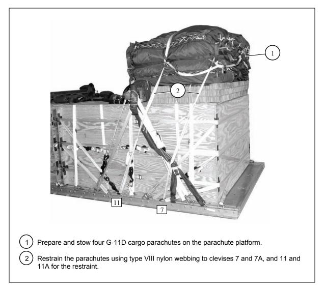
Figure 11-16. Cargo Parachute Stowed
