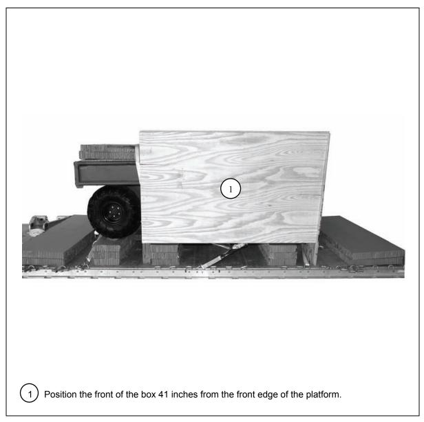
Figure 10-11. M-Gator Box Positioned
