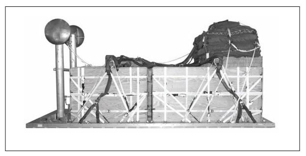
Figure 11-1. Mass Supply Load Rigged on DRAS Platform
