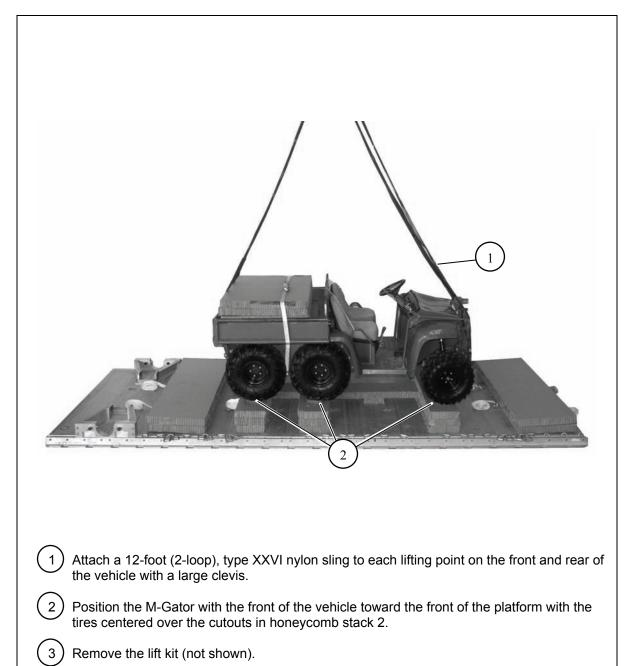
Figure 10-6. M-Gator Positioned
