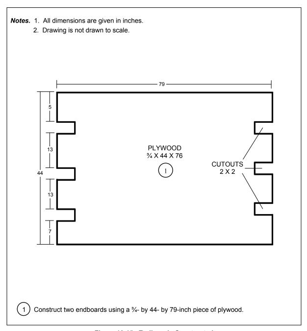
Figure 10-15. Endboards Constructed
