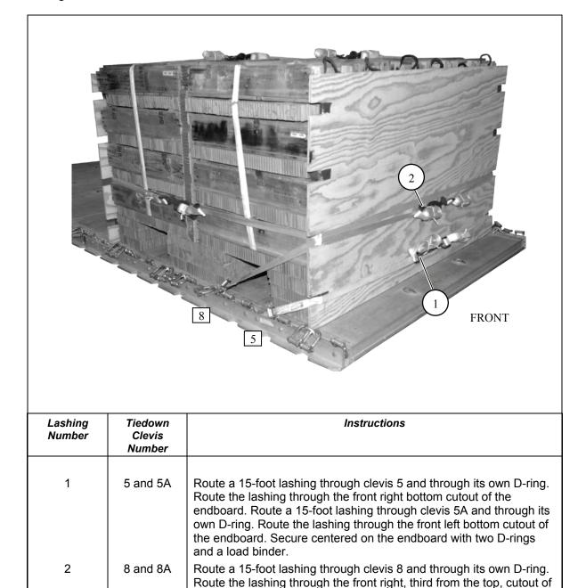
Figure 9-6. Lashings Installed for First Stack
