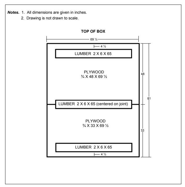
Figure 10-10. M-Gator Box Built
