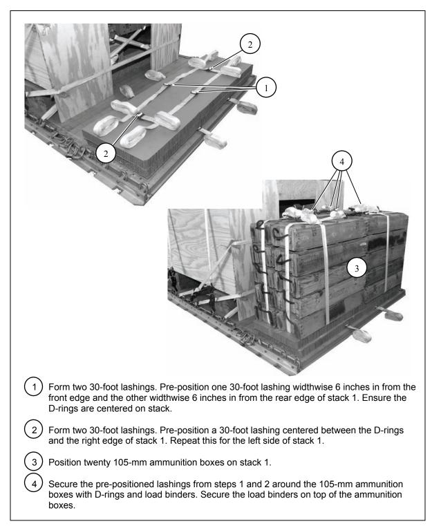
Figure 10-16. First Ammunition Stack Positioned
