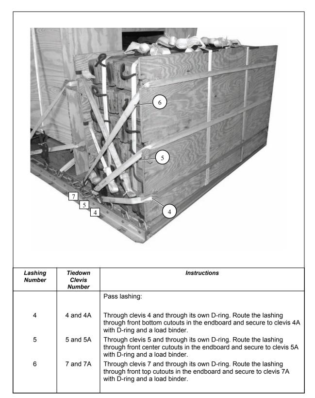
Figure 10-18. Lashings 4 Through 6 Installed on First Ammunition Stack
