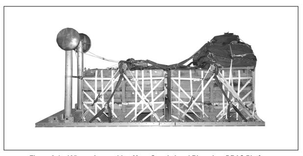
Figure 9-1. 105-mm Ammunition Mass Supply Load Rigged on DRAS Platform
