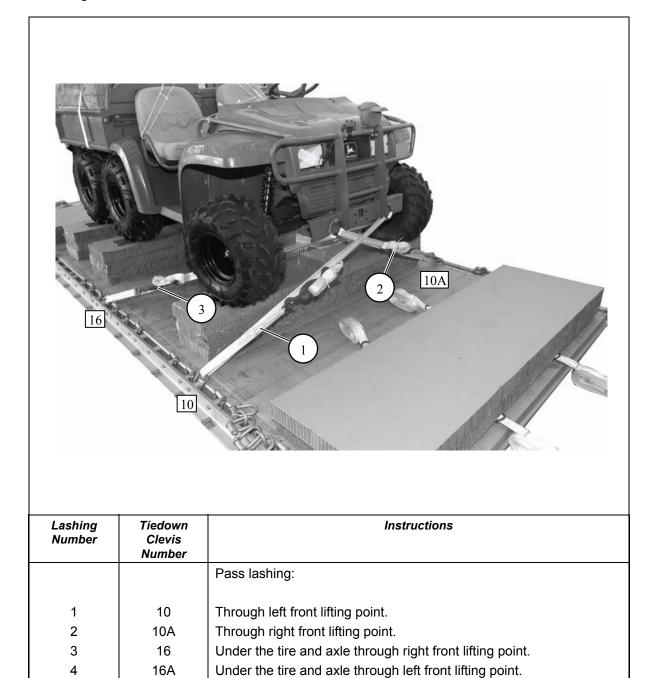
Figure 10-7. Lashings 1 Through 4 Installed
