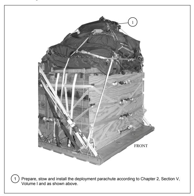
Figure 9-12. Deployment Parachute Installed
