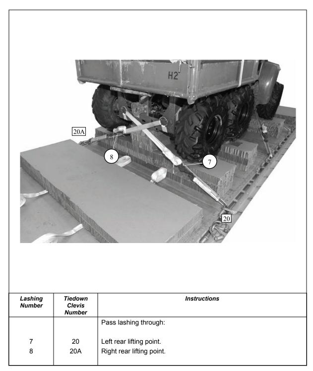
Figure 10-9. Lashings 7 and 8 Installed
