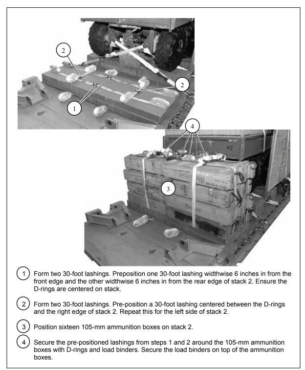
Figure 10-20. Second Ammunition Stack Positioned
