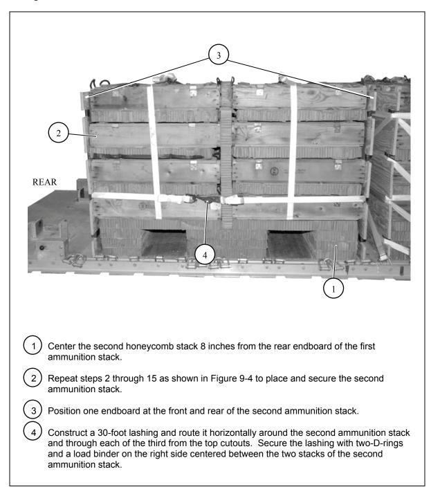
Figure 9-7. Honeycomb, Lashings, Ammunition and Endboards Placed for Second Stack
