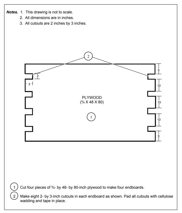
Figure 9-5. Endboards Constructed and Placed
