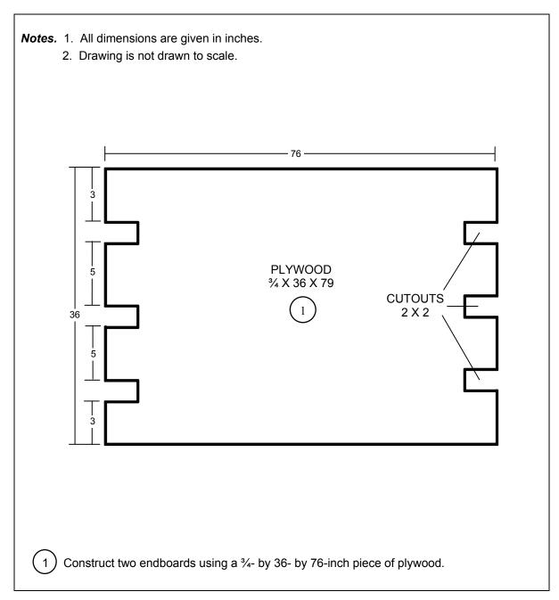
Figure 10-19. Endboards Constructed
