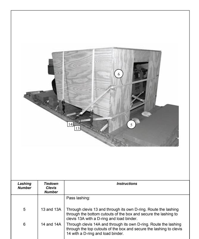
Figure 10-14. Lashings 5 and 6 Installed on M-Gator Box
