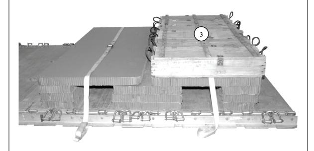
Position six 105-mm ammunition containers on top of the honeycomb and centered on the pre-positioned lashings on the front of the stack.
