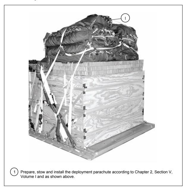
Figure 11-17. Deployment Parachute Installed
