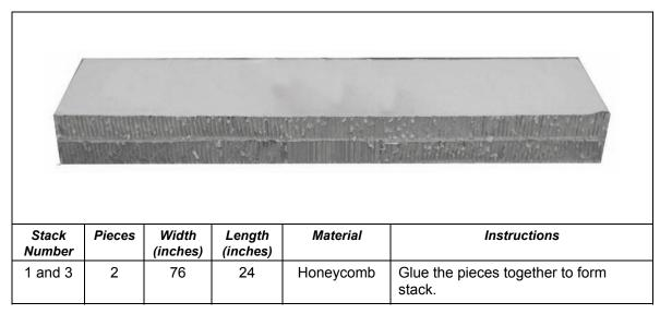
Figure 10-3. Honeycomb Stacks Prepared
