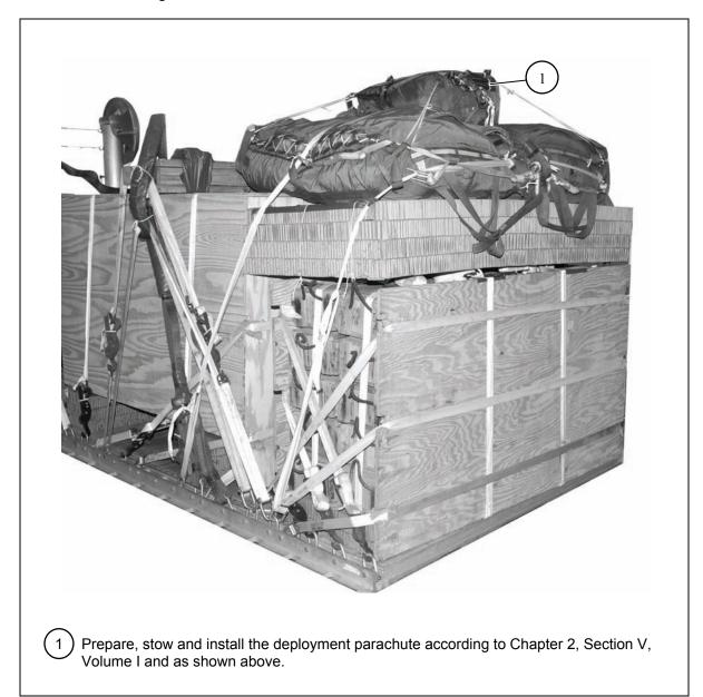
Figure 10-26. Deployment Parachute Installed
