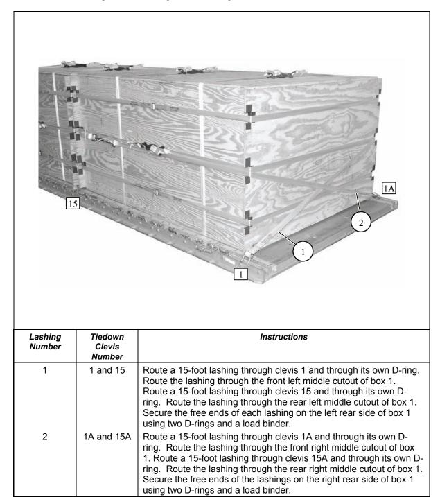
Figure 11-6. Lashings 1 and 2 Installed
