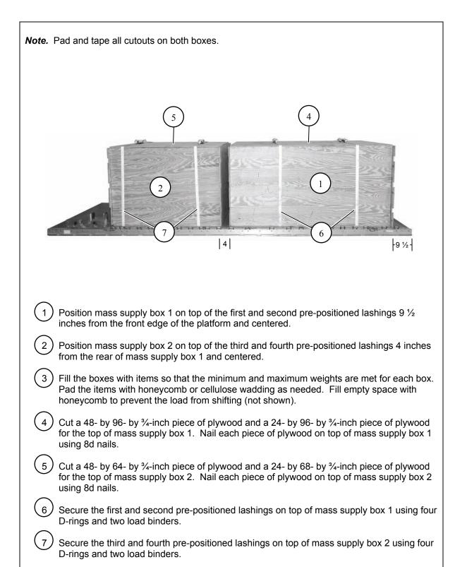
Figure 11-5. Mass Supply Boxes Positioned
