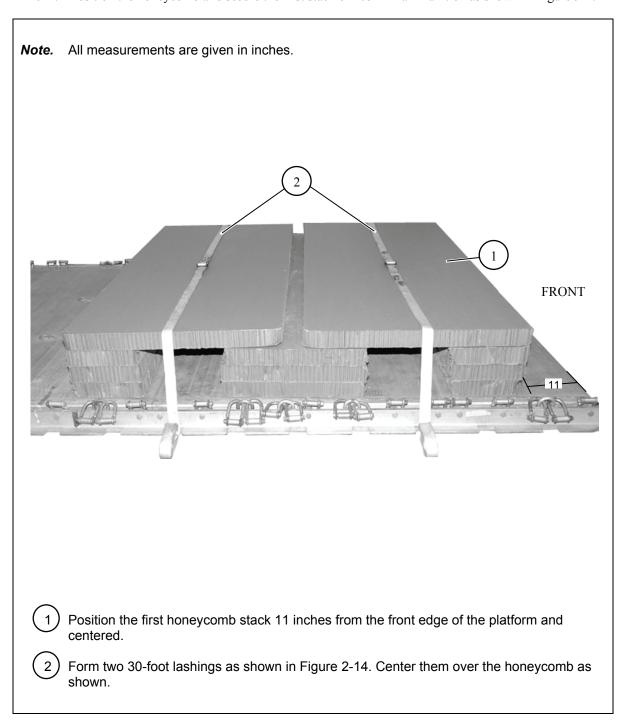
Figure 9-4. Honeycomb Positioned and Ammunition Secured
