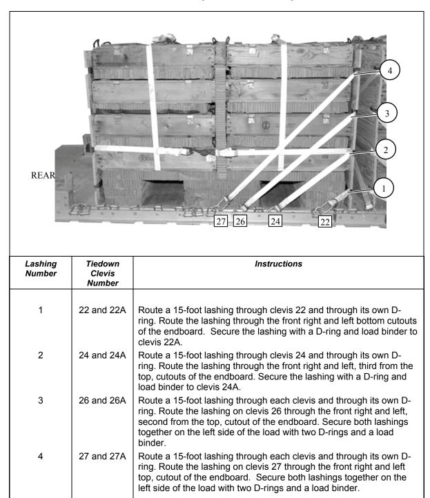
Figure 9-8. Lashings Installed for Second Stack
