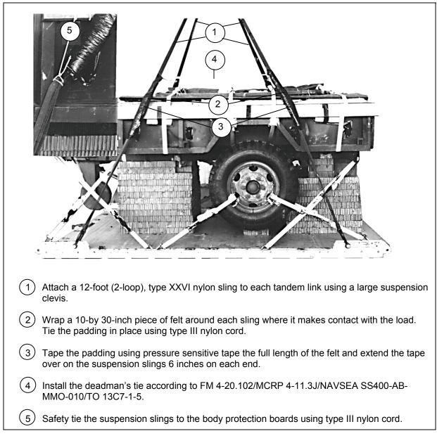
Figure 4-14. Suspension Slings Installed and Safety Tied
