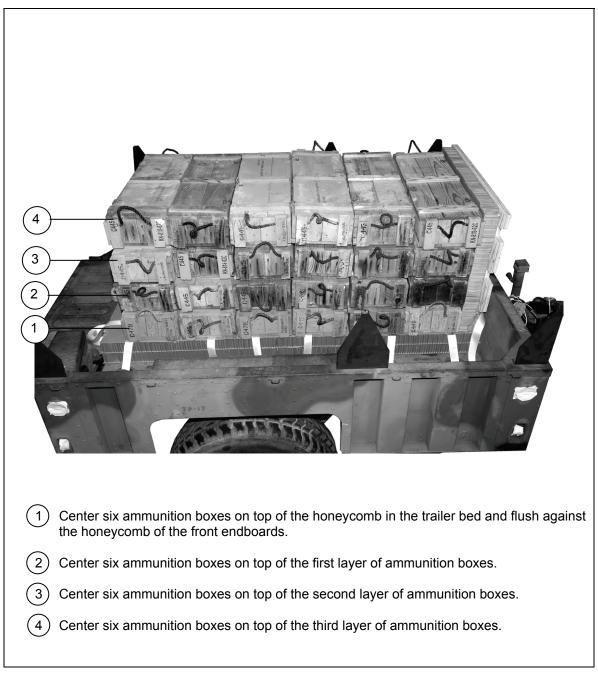
Figure 3-10. Accompanying Load Positioned
