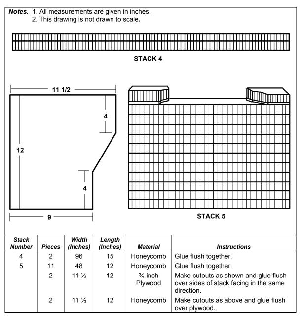
Figure 7-6. Stacks 4 and 5 Prepared
