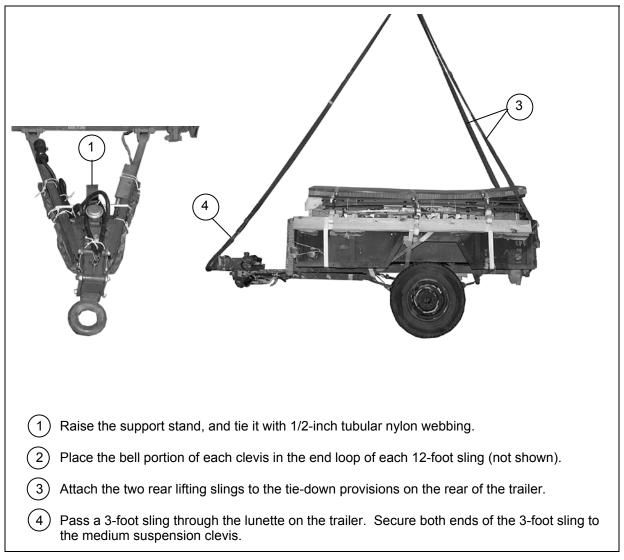
Figure 2-16. Lifting Slings Installed
