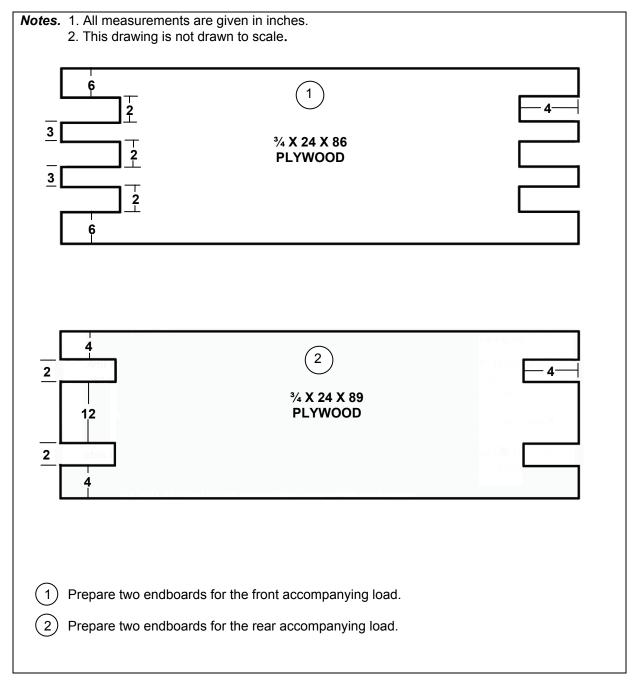
Figure 6-3. Endboards Constructed
