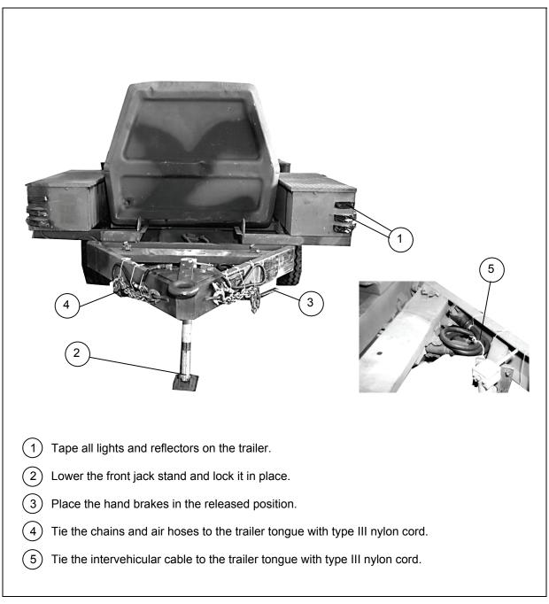
Figure 9-9. Front of Trailer Prepared
