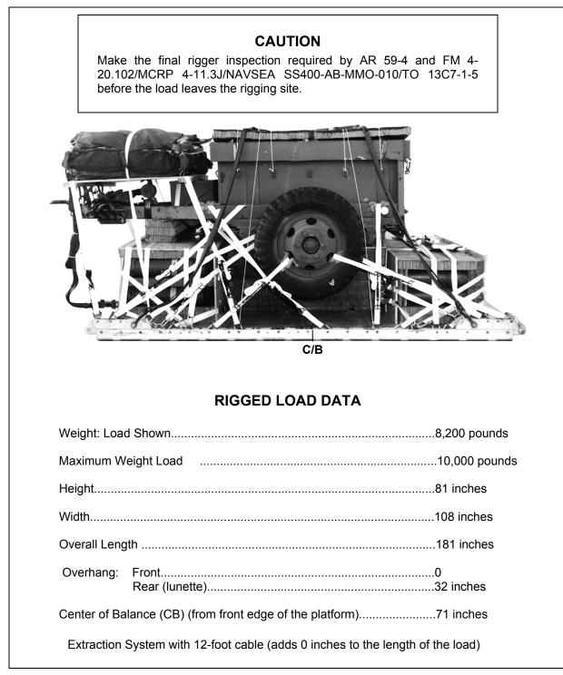
Figure 6-20. 1 <sup>1</sup>/<sub>2</sub>-Ton Ammunition Trailer Rigged on a 12-Foot, Type V Platform for Low-Velocity Airdrop
