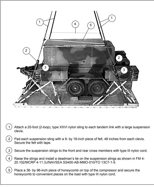
Figure 9-21. Suspension Slings Installed and Safety Tied
