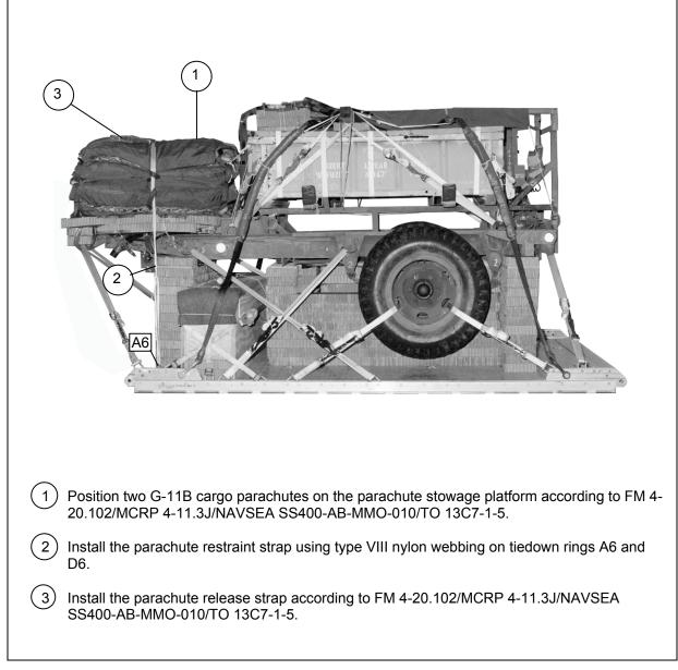
Figure 7-15. Cargo Parachutes Positioned and Restrained
