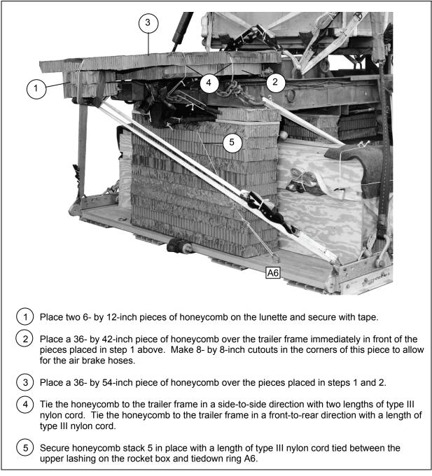
Figure 7-14. Parachute Stowage Platform Built and Secured
