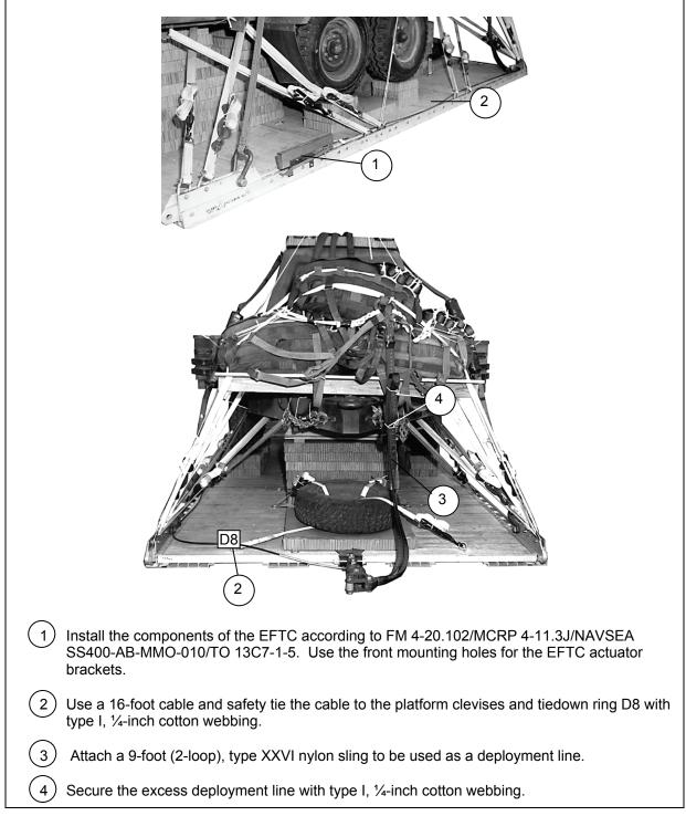
Figure 9-26. Extraction System Installed
