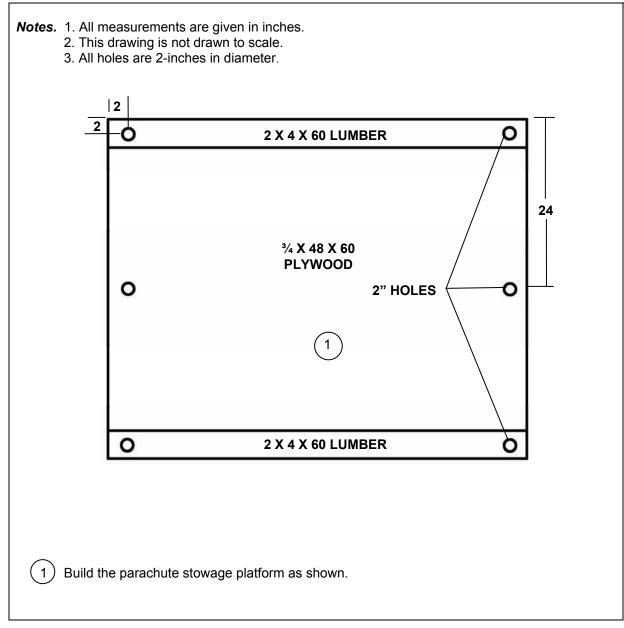
Figure 8-19. Parachute Stowage Platform Built
