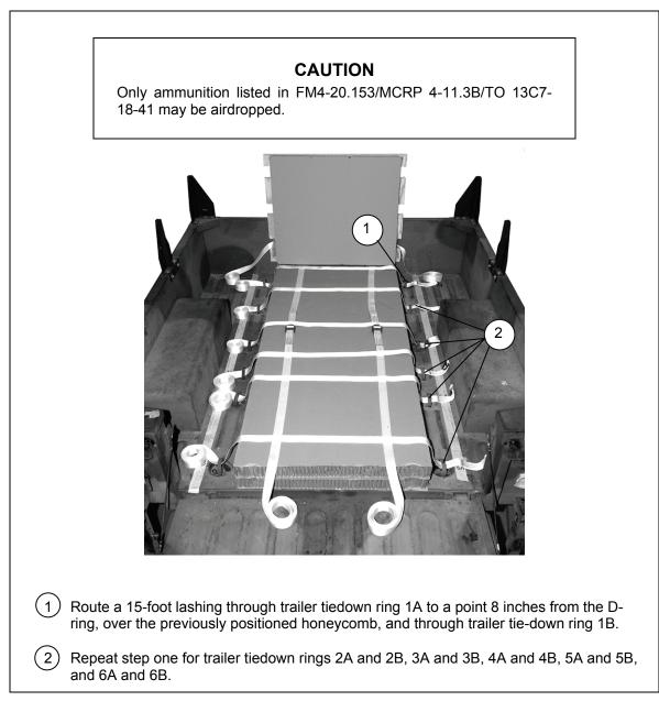
Figure 3-9. Lashings Pre-Positioned on the Trailer Bed
