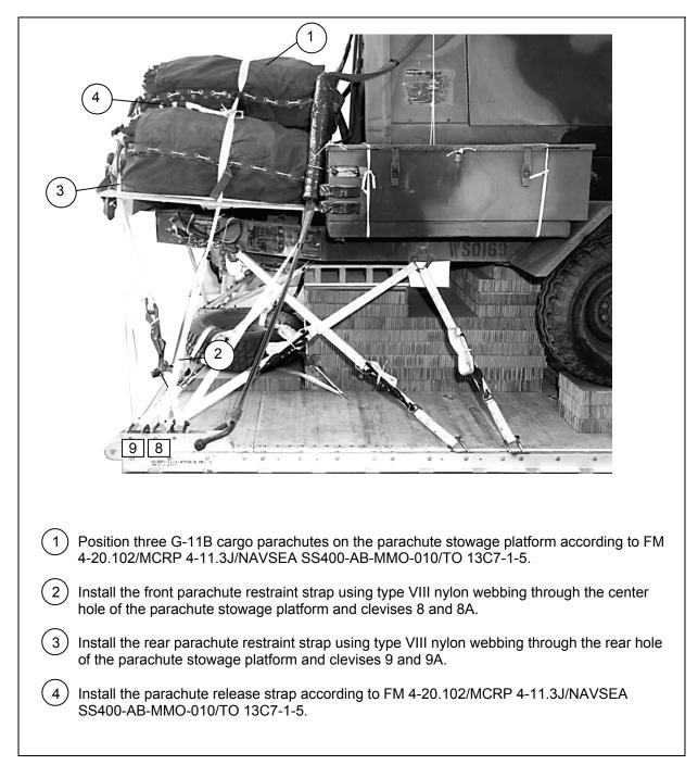
Figure 9-24. Cargo Parachutes Positioned and Restrained
