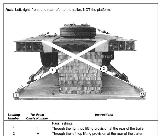
Figure 8-14. Lashings 1 and 2 Installed
