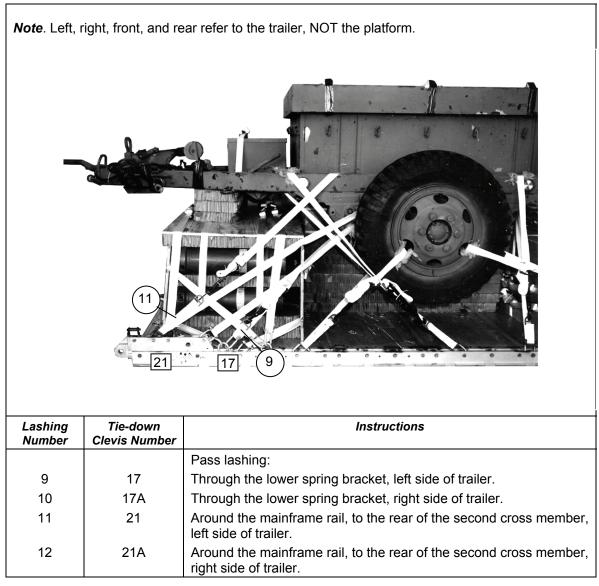
Figure 6-13. Lashing 9 through 12 Installed
