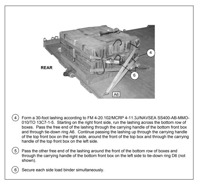
Figure 2-6. Ammunition Boxes Lashed and Secured on the Rear of the Platform (Continued)
