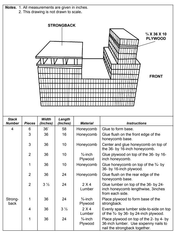
Figure 9-5. Stack 4 Built
