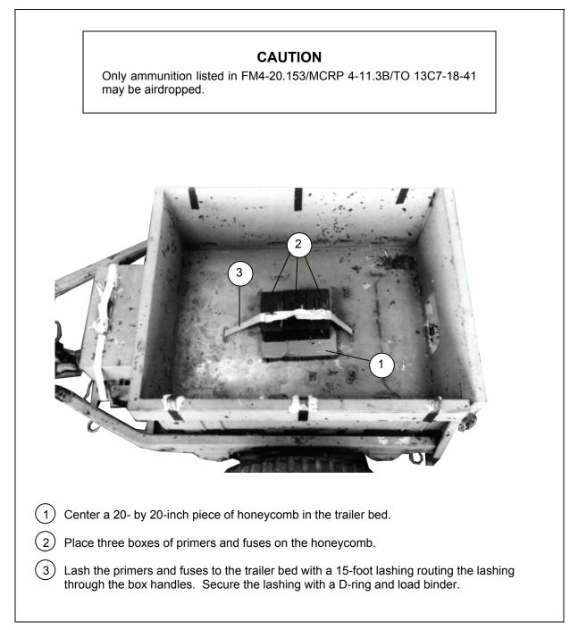
Figure 6-10. Accompanying Load Stowed in Trailer
