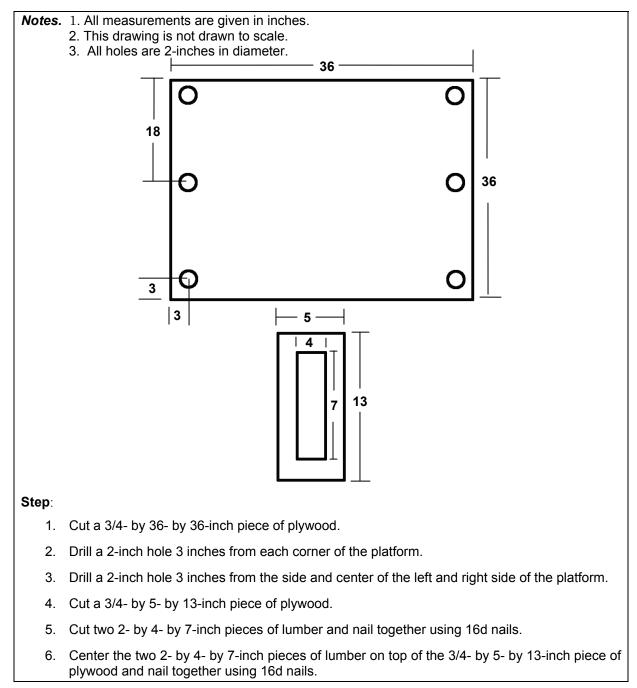
Figure 2-20. Parachute Stowage Platform Built
