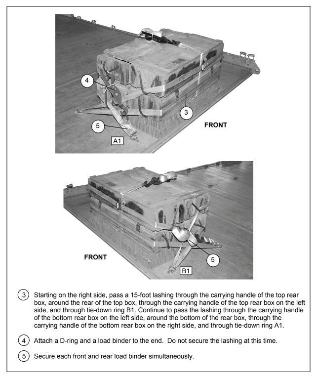
Figure 2-4. Ammunition Boxes Lashed and Secured on the Front of the Platform (Continued)
