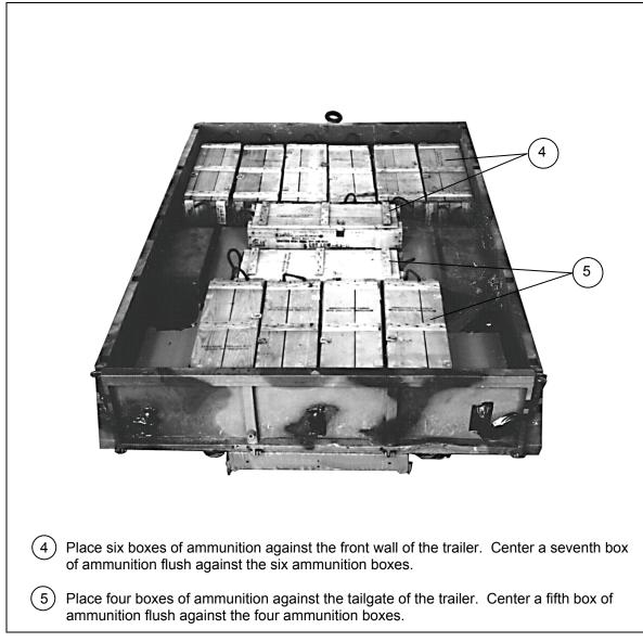
Figure 4-8. Accompanying Load and Trailer Components Stowed (Continued)
