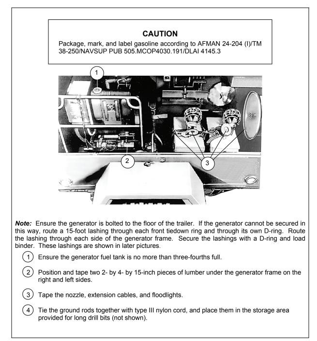
Figure 10-6. Right Side of Trailer Prepared
