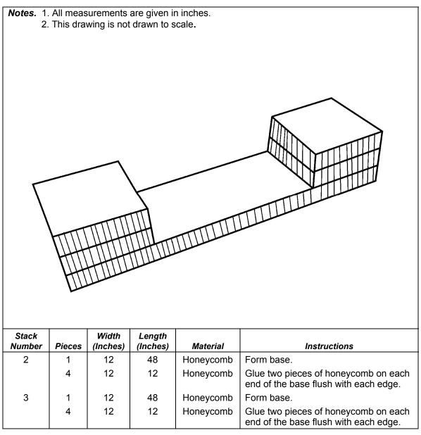
Figure 9-4. Stacks 2 and 3 Built
