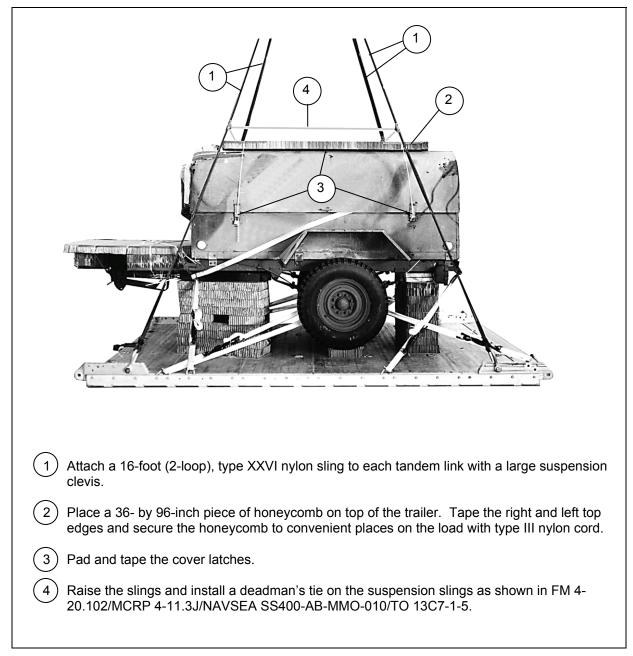
Figure 10-12. Suspension Slings Installed and Safety Tied
