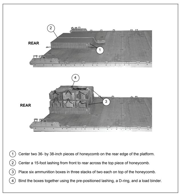
Figure 2-5. Ammunition Boxes Positioned on the Rear of the Platform
