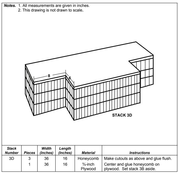
Figure 7-4. Components of Stack 3 Prepared (Continued)
