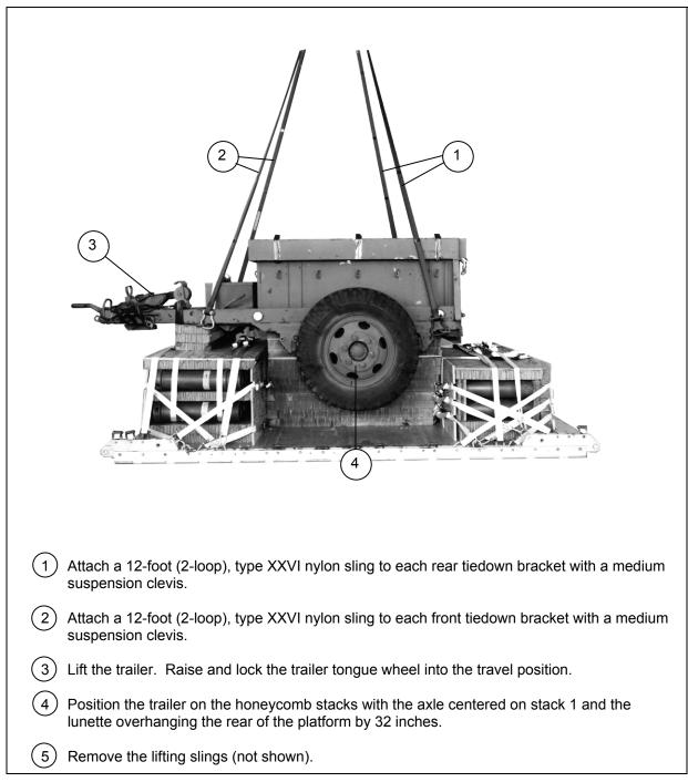
Figure 6-11. Lifting and Positioning the Trailer
