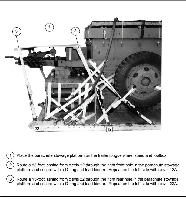
Figure 6-16. Parachute Stowage Platform Installed
