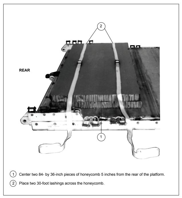
Figure 6-6. Rear Accompanying Load Prepared and Stowed on Platform
