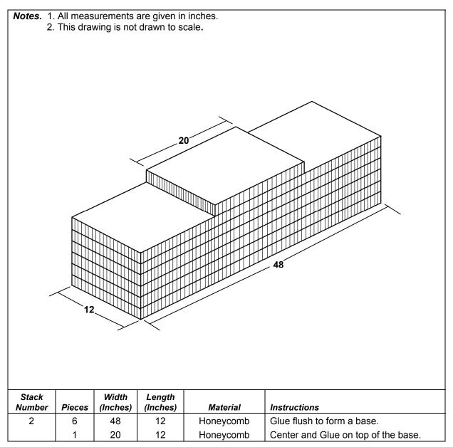
Figure 5-4. Honeycomb Stack 2 Prepared
