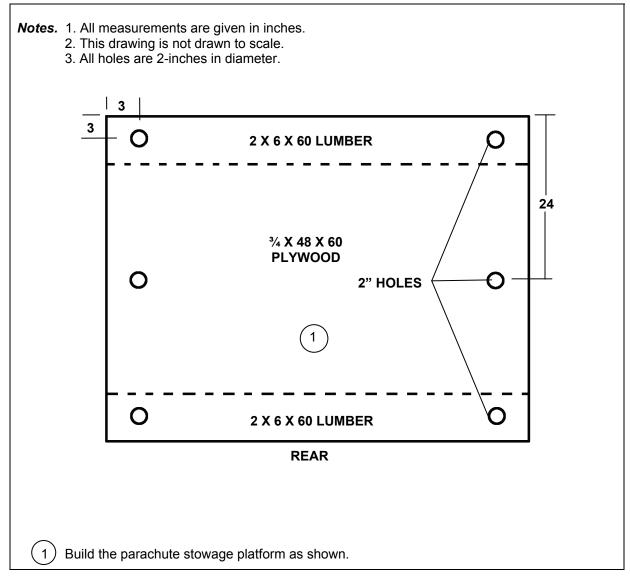
Figure 6-15. Parachute Stowage Platform Built
