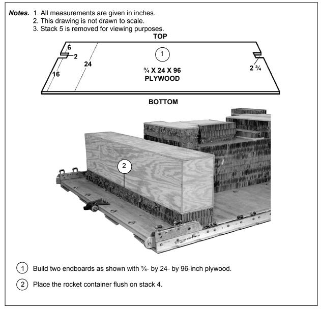
Figure 7-9. Rocket Container Stowed on Platform
