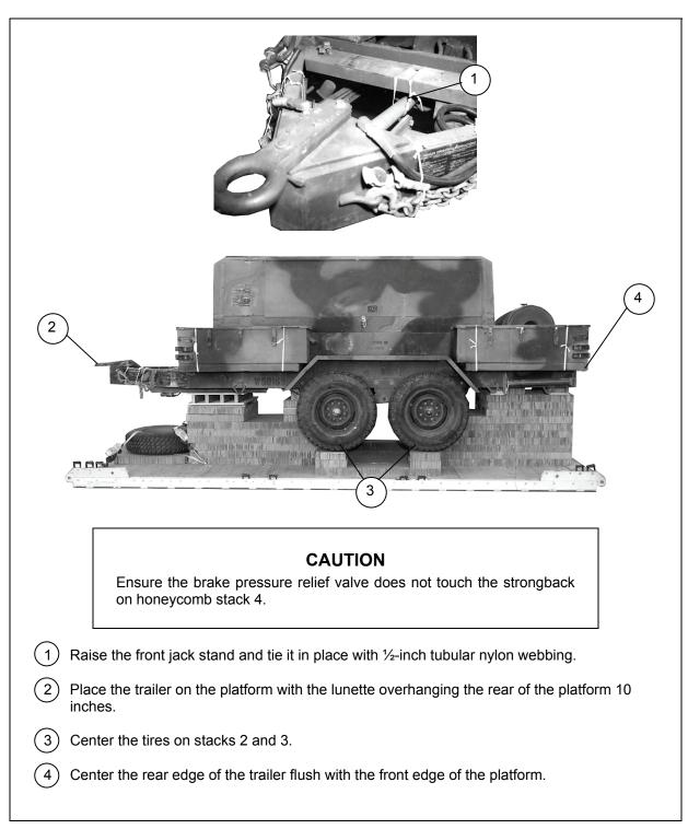
Figure 9-18. Trailer Positioned on Platform
