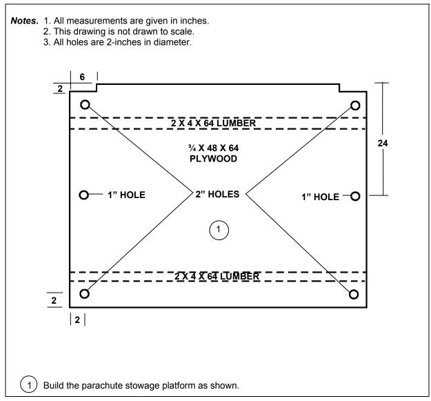
Figure 9-22. Parachute Stowage Platform Built
