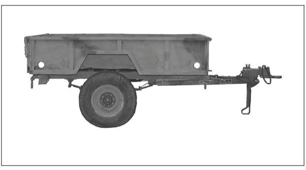
Figure 2-1. M101A2, <sup>3</sup>/<sub>4</sub>-Ton Cargo Trailer
