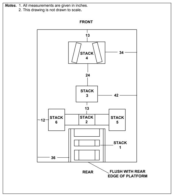
Figure 5-7. Honeycomb Stacks Positioned on Platform
