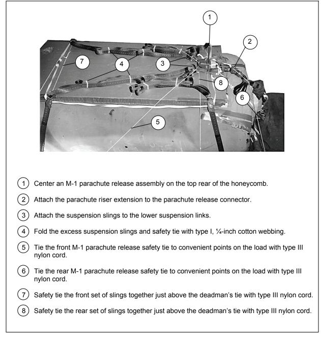
Figure 10-14. M-1 Parachute Release Installed
