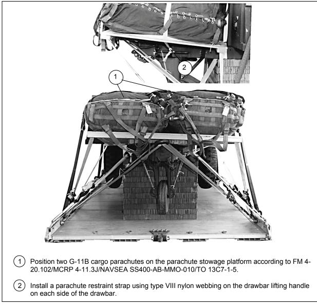
Figure 4-17. Cargo Parachutes Positioned and Restrained
