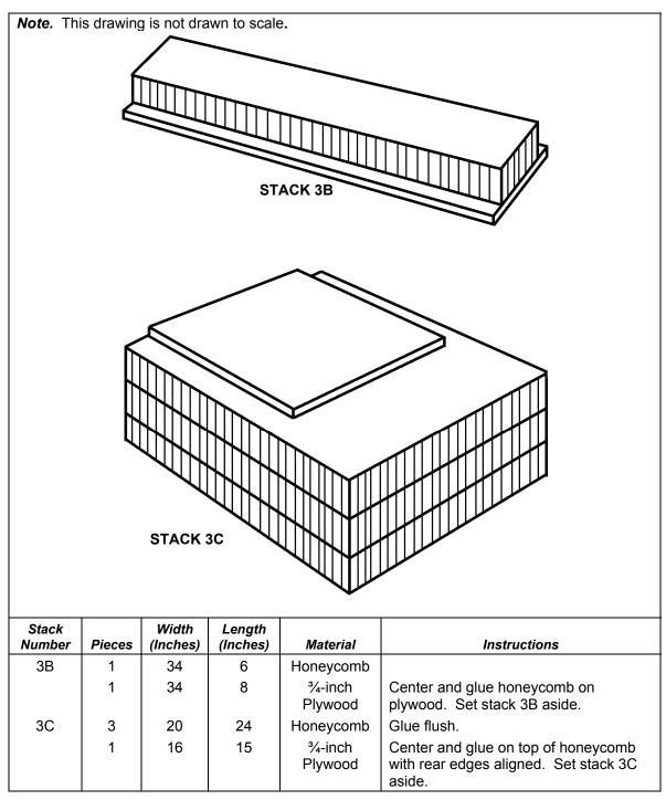
Figure 7-4. Components of Stack 3 Prepared (Continued)
