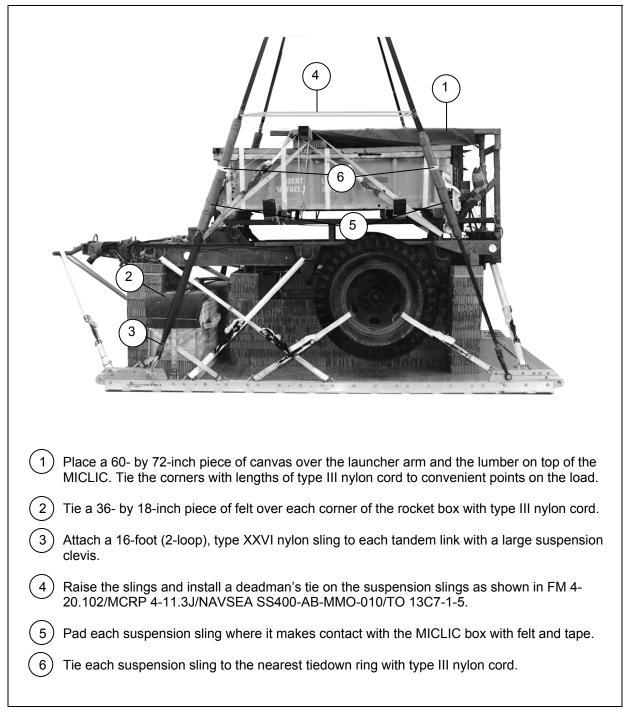
Figure 7-13. Suspension Slings Installed and Safety Tied
