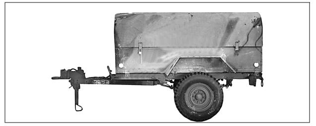
Figure 10-1. Trailer-Mounted Engineer Electrical Tool Outfit
