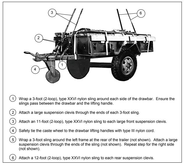
Figure 4-11. Trailer Lifting Slings Installed
