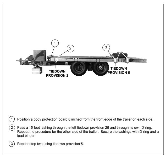
Figure 8-12. Body Protection Boards Secured
