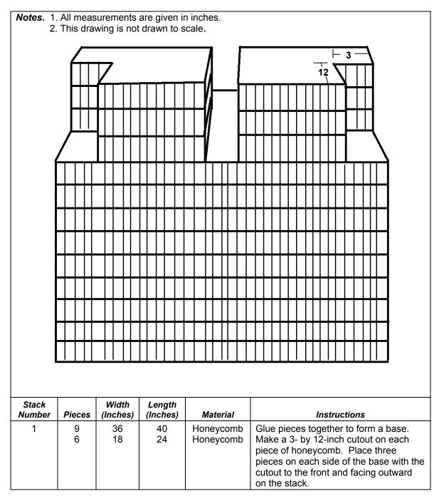
Figure 4-3. Honeycomb Stack 1 Prepared
