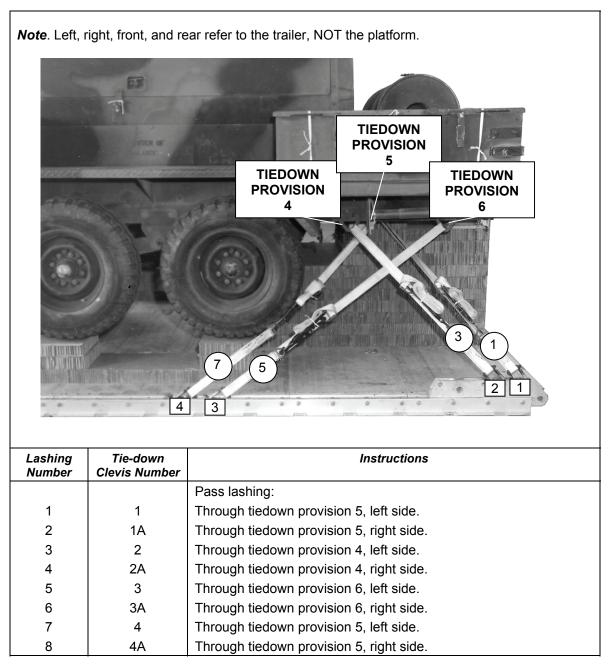
Figure 9-19. Lashings 1 through 8 Installed
