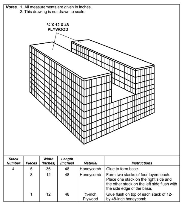
Figure 8-5. Stack 4 Built
