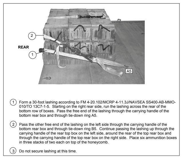
Figure 2-6. Ammunition Boxes Lashed and Secured on the Rear of the Platform
