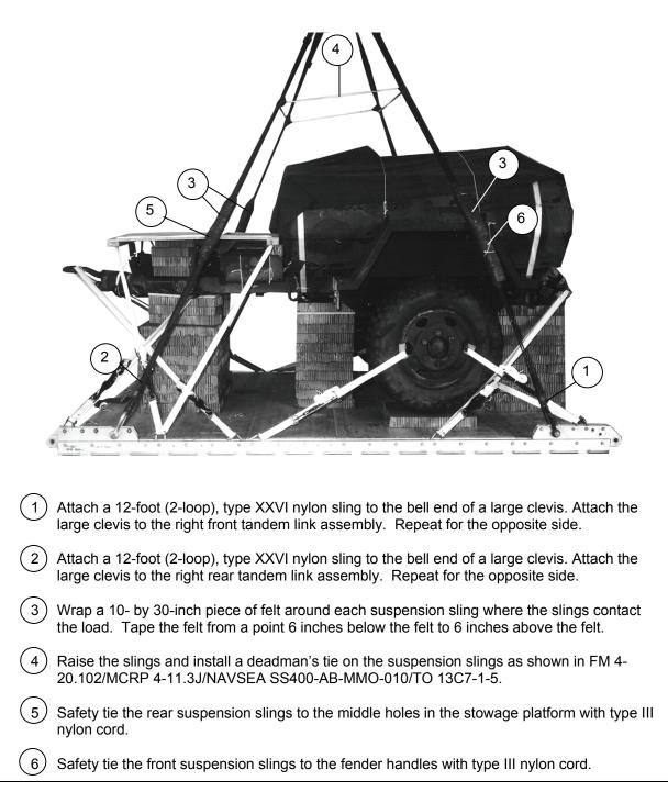
Figure 5-15. Suspension Slings Installed and Safety Tied
