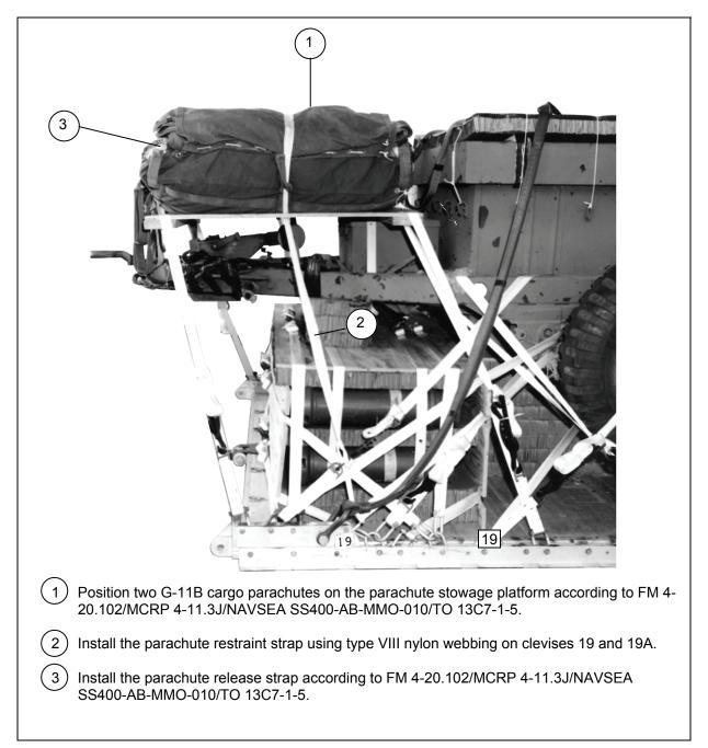
Figure 6-17. Cargo Parachutes Positioned and Restrained
