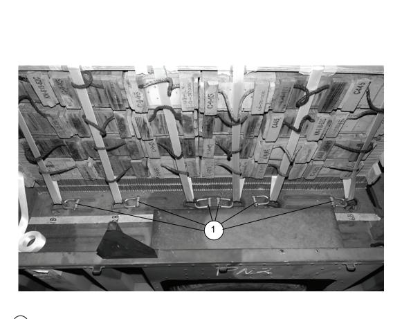
1) Attach a type V, platform clevis to each trailer tie-down provision. Face the clevises on 1A, 2A, 3A, 1B, 2B and 3B toward the rear of the trailer. Face the clevises on 4A, 5A, 6A, 4B, 5B and 6B toward the front of the trailer.
