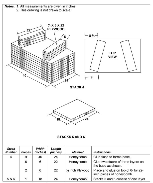
Figure 5-6. Honeycomb Stacks 4 through 6 Prepared
