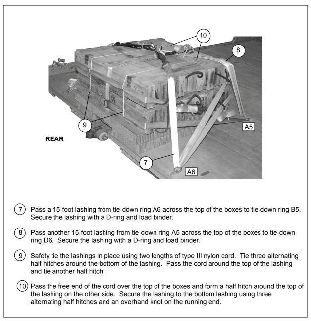
Figure 2-6. Ammunition Boxes Lashed and Secured on the Rear of the Platform (Continued)
