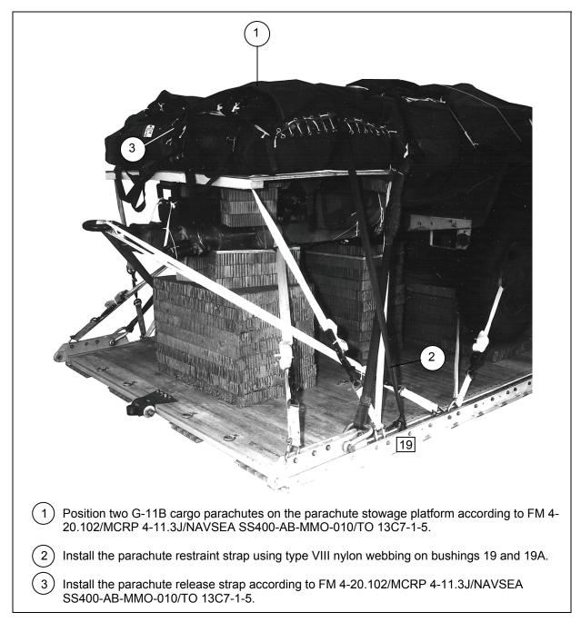
Figure 5-16. Cargo Parachutes Positioned and Restrained
