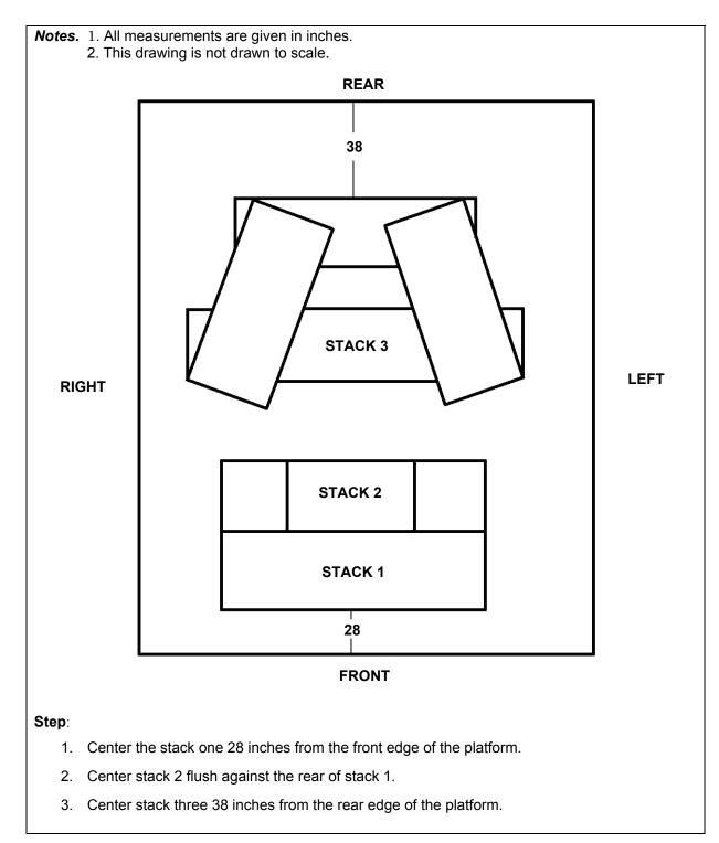
Figure 2-10. Honeycomb Stacks Positioned on the Platform
