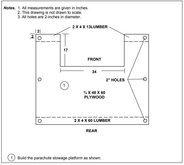
Figure 5-12. Parachute Stowage Platform Built
