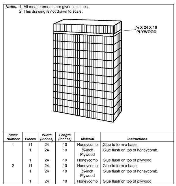
Figure 7-3. Honeycomb Stacks 1 and 2 Built
