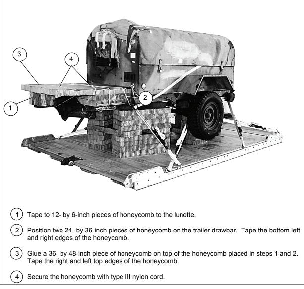
Figure 10-11. Parachute Stowage Platform Prepared and Positioned
