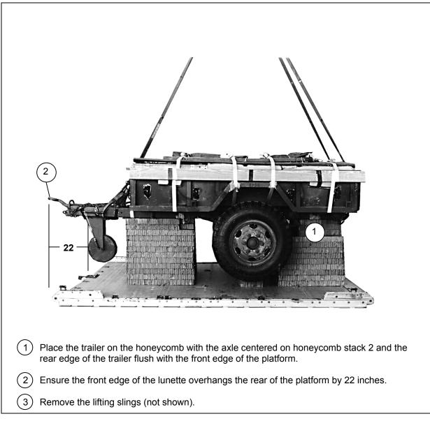
Figure 4-12. Trailer Positioned
