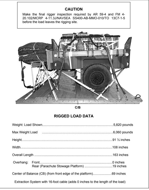
Figure 3-27. M1101 HMT-L <sup>3</sup>/<sub>4</sub>-Ton Trailer Rigged on a 12-Foot, Type V Platform for Low-Velocity Airdrop
