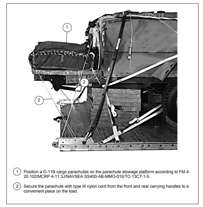
Figure 10-13. Cargo Parachute Positioned and Restrained
