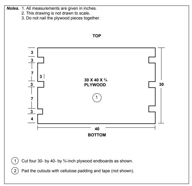
Figure 3-7. End Boards Built
