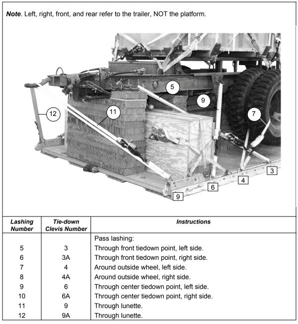
Figure 7-12. Lashing 5 through 12 Installed
