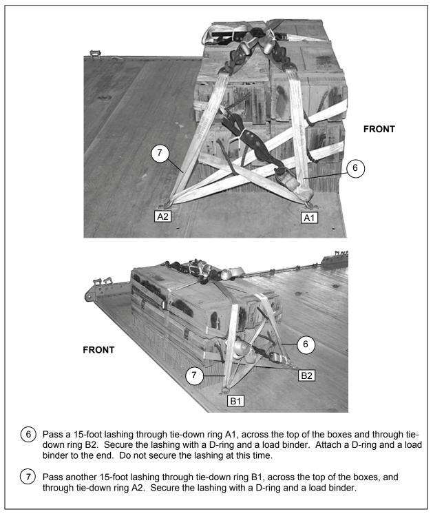
Figure 2-4. Ammunition Boxes Lashed and Secured on the Front of the Platform (Continued)
