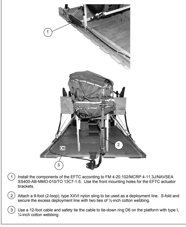
Figure 3-26. Extraction System Installed
