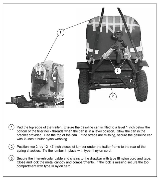
Figure 10-8. Outside of Trailer Prepared
