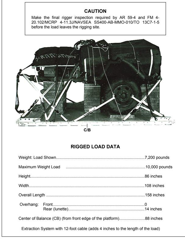
Figure 5-19. M149A1 400-Gallon Water Trailer Rigged on a 12-Foot, Type V Platform for Low-Velocity Airdrop
