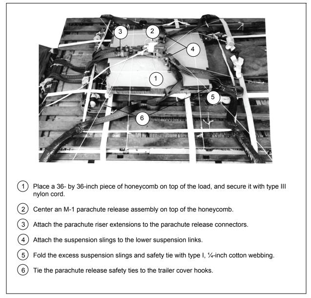
Figure 4-18. M-1 Parachute Release Installed
