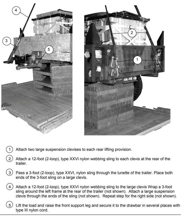
Figure 3-17. Trailer Lifting Slings Installed
