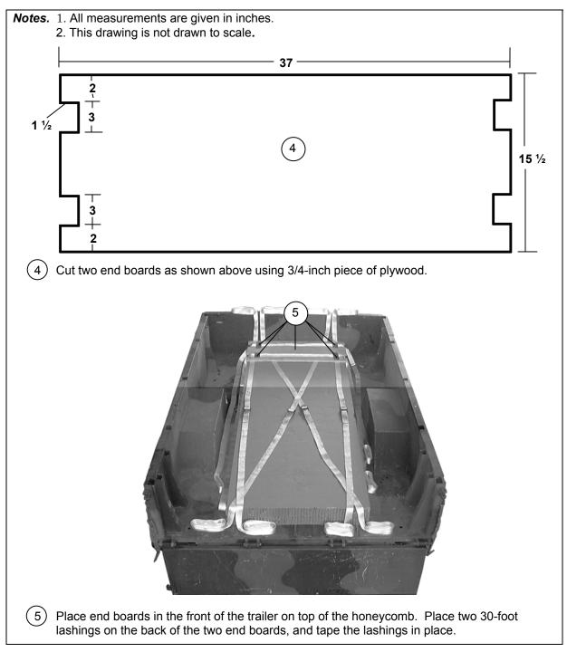
Figure 2-13. Honeycomb, Lashings, and End Boards Positioned in the Trailer (Continued)
