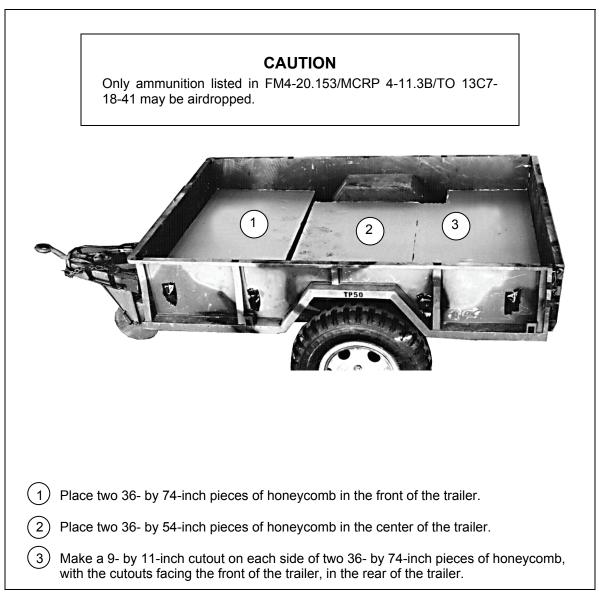
Figure 4-8. Accompanying Load and Trailer Components Stowed
