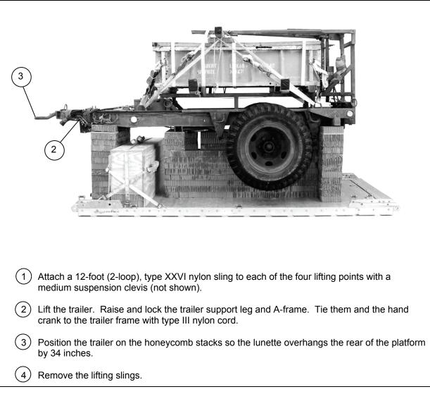
Figure 7-10. MICLIC Trailer Lifted and Positioned on Platform
