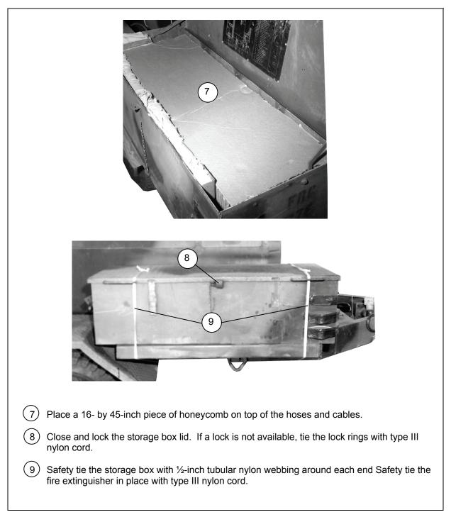
Figure 9-13. Storage Box 3 Prepared and Secured (Continued)
