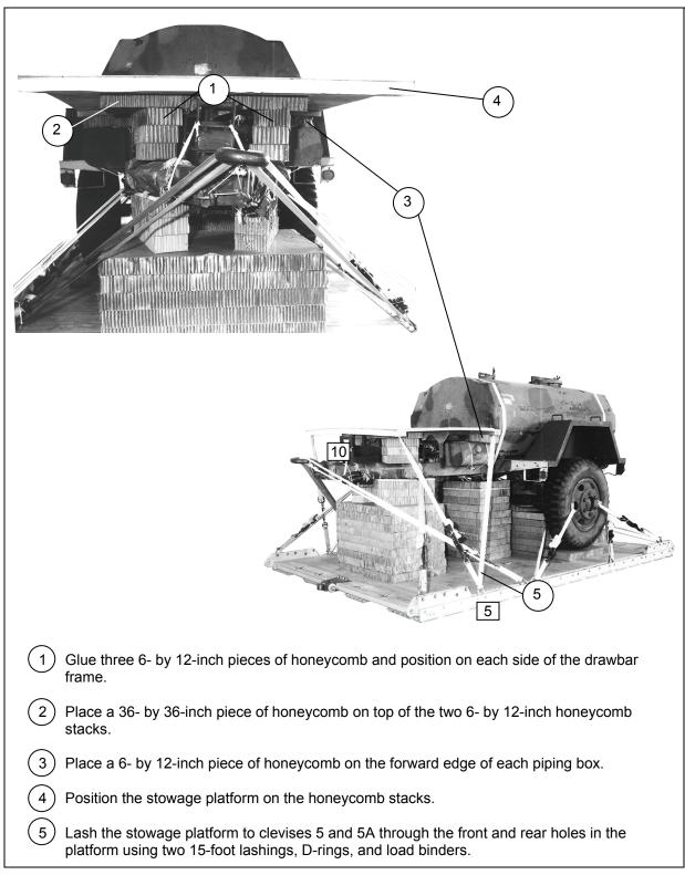
Figure 5-13. Parachute Stowage Platform Installed
