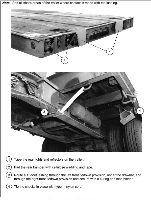
Figure 8-9. Rear of Trailer Prepared
