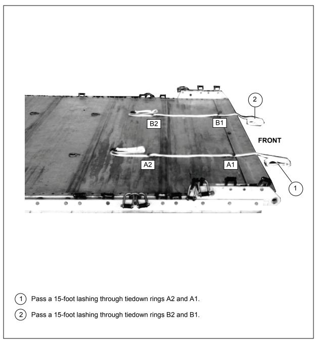
Figure 6-4. Front Accompanying Load Prepared and Stowed on Platform
