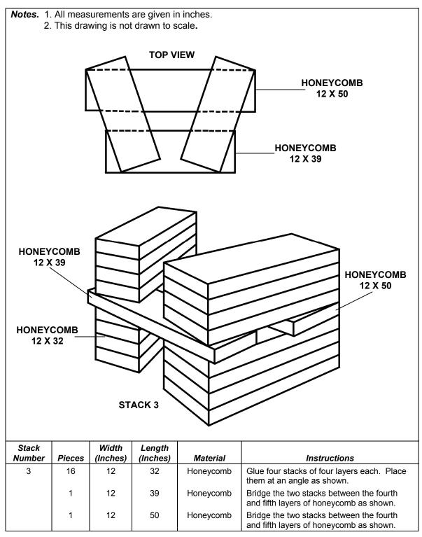
Figure 10-4. Honeycomb Stack 3 Built
