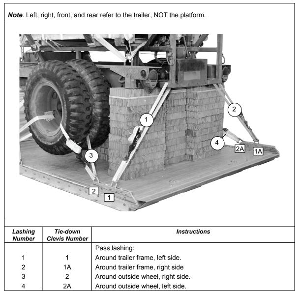
Figure 7-11. Lashing 1 through 4 Installed
