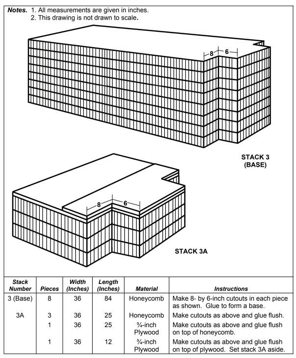
Figure 7-4. Components of Stack 3 Prepared
