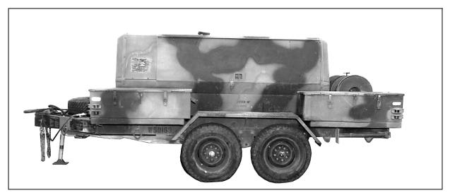
Figure 9-1. Ingersol-Rand Model, 250-CFM, Trailer-Mounted Air Compressor
