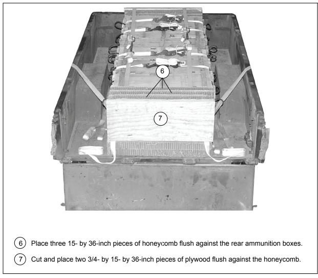
Figure 2-14. Ammunition Boxes Lashed and Secured in the Trailer (Continued)
