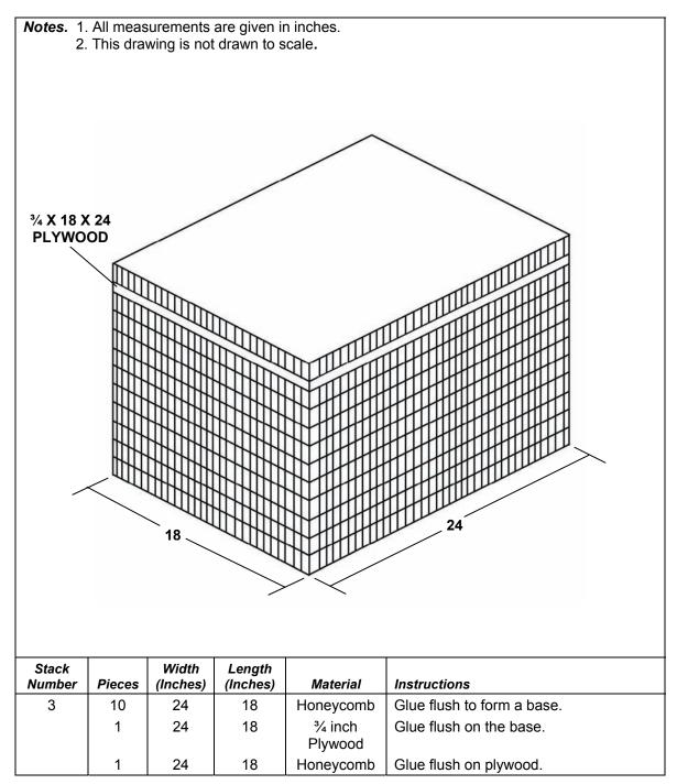
Figure 5-5. Honeycomb Stack 3 Prepared
