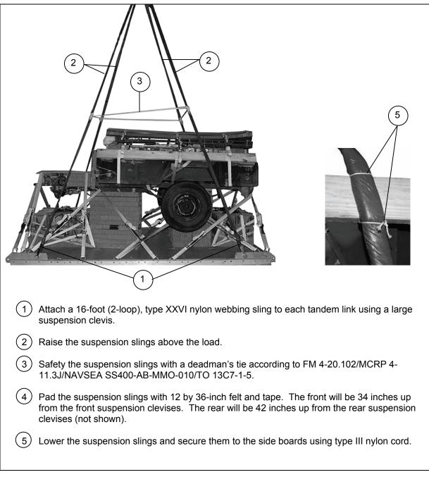
Figure 2-22 Suspension Slings Installed and Safety Tied
