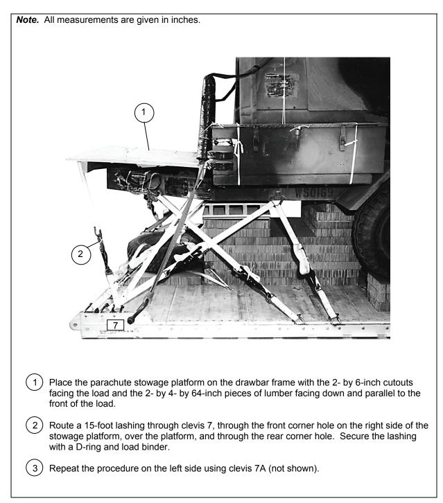
Figure 9-23. Parachute Stowage Platform Installed
