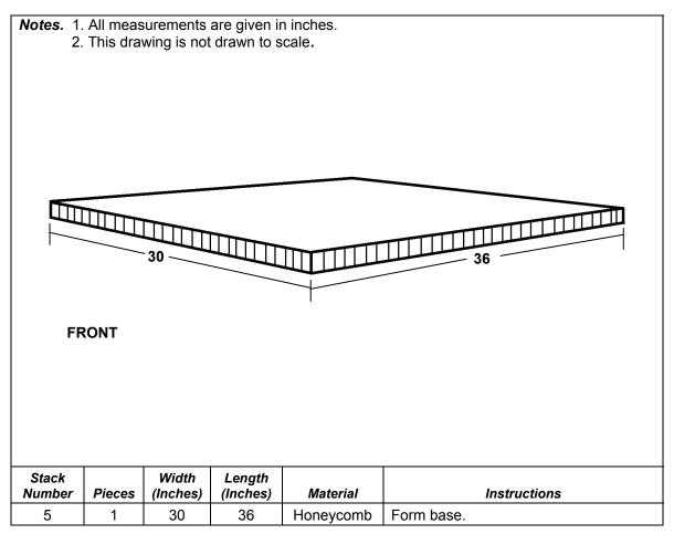
Figure 9-6. Stack 5 Built
