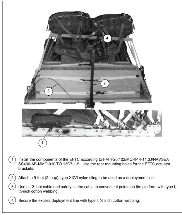
Figure 6-19. Extraction System Installed
