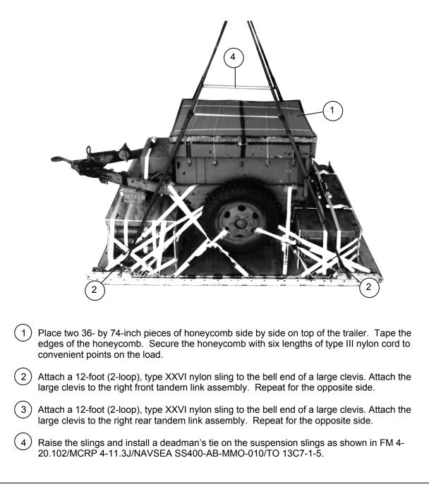
Figure 6-14. Suspension Slings Installed and Safety Tied
