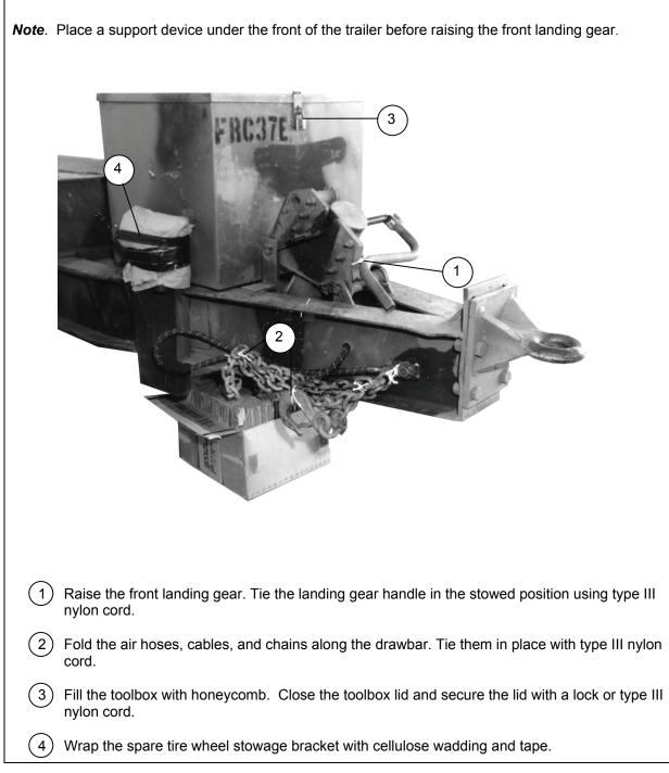
Figure 8-8. Trailer Components Secured
