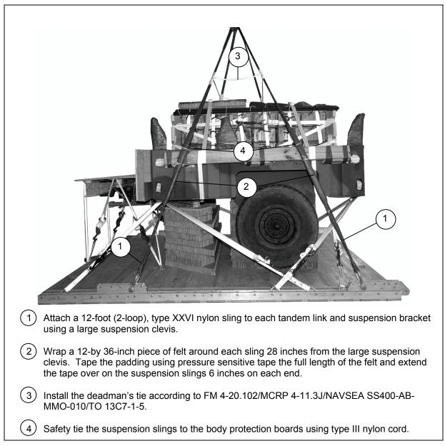
Figure 3-23. Suspension Slings Installed and Safety Tied
