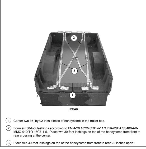
Figure 2-13. Honeycomb, Lashings, and End Boards Positioned in the Trailer
