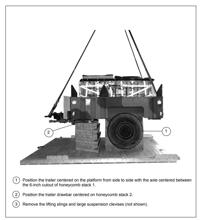
Figure 3-18. Trailer Positioned
