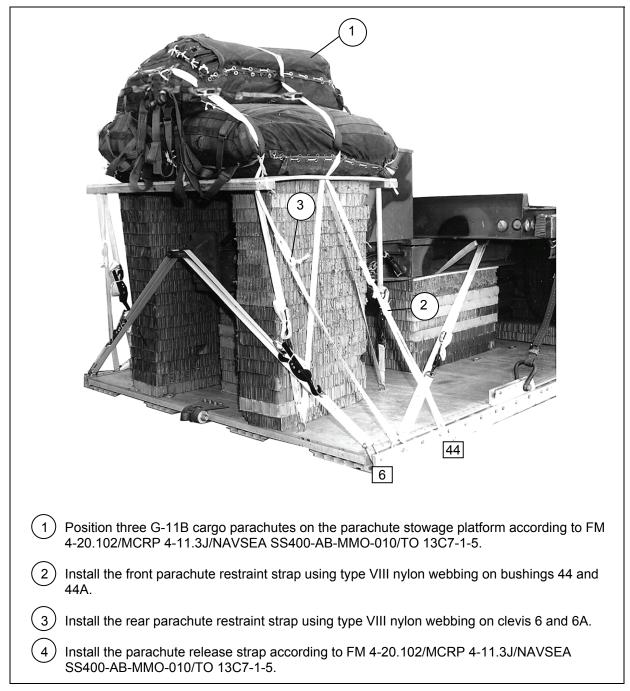
Figure 8-21. Cargo Parachutes Positioned and Restrained
