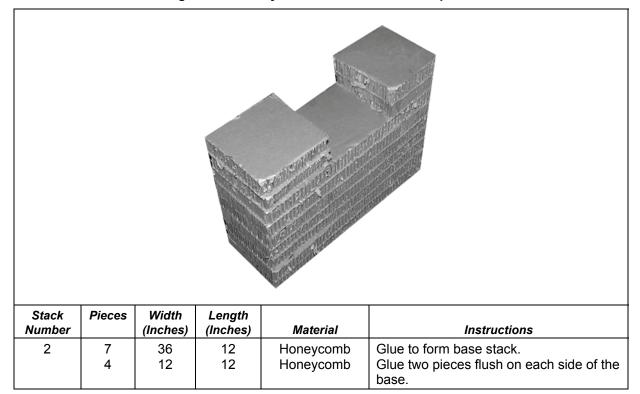
Figure 2-8. Honeycomb Stack 2 Prepared
