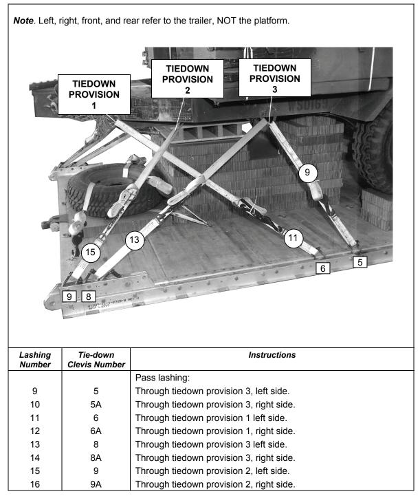
Figure 9-20. Lashings 9 through 16 Installed
