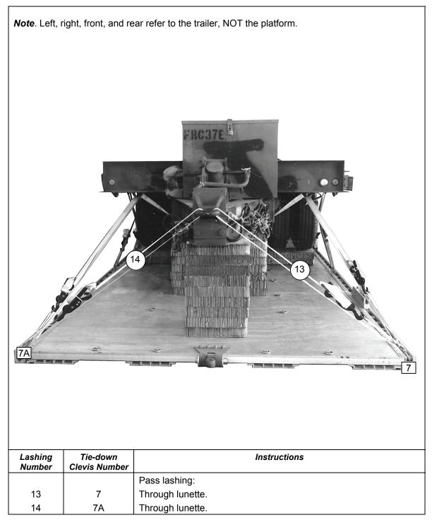
Figure 8-16. Lashings 13 and 14 Installed
