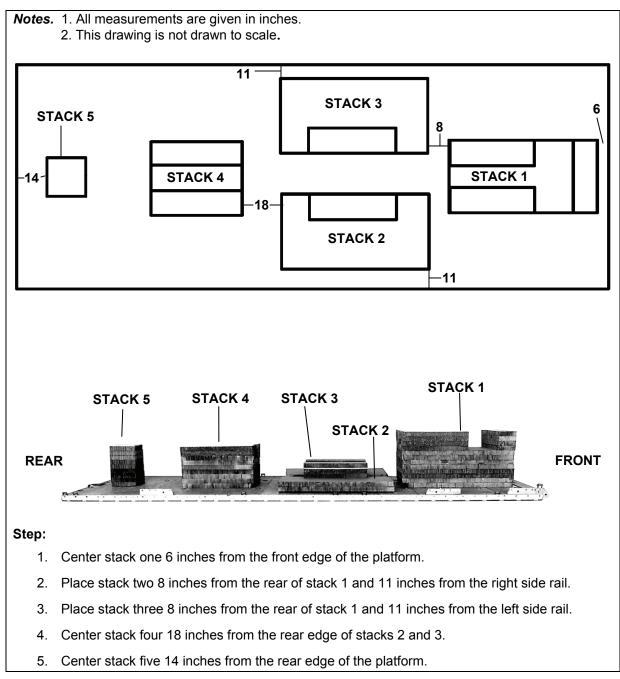
Figure 8-7. Honeycomb Stacks Positioned on Platform
