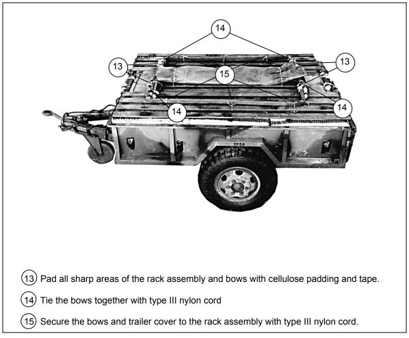
Figure 4-8. Accompanying Load and Trailer Components Stowed (Continued)
