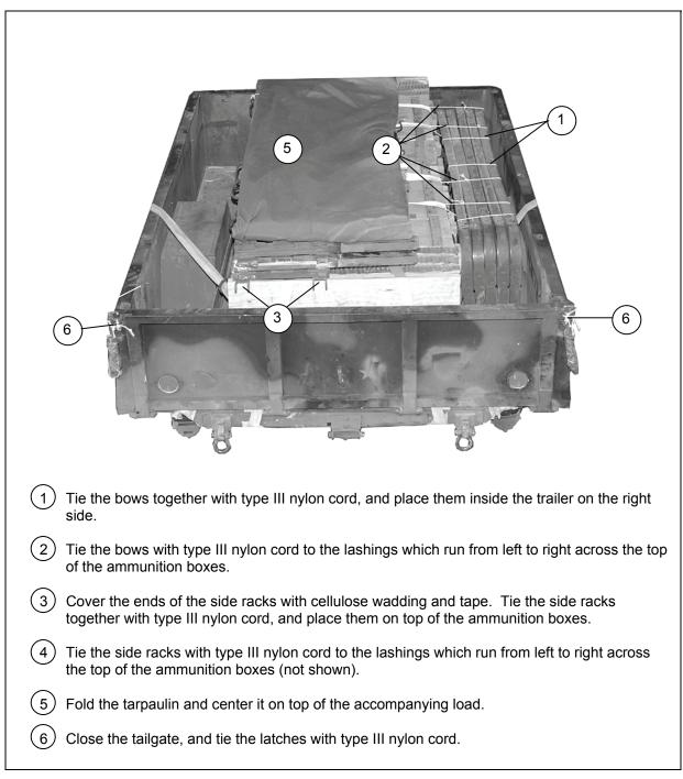
Figure 2-15. Trailer Components Stowed.
