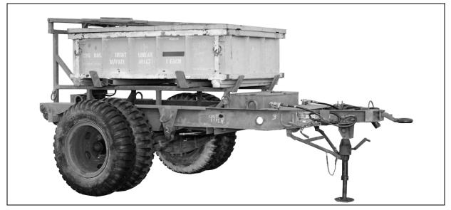
Figure 7-1. MICLIC on 2 <sup>1</sup>/<sub>2</sub>-Ton Trailer
