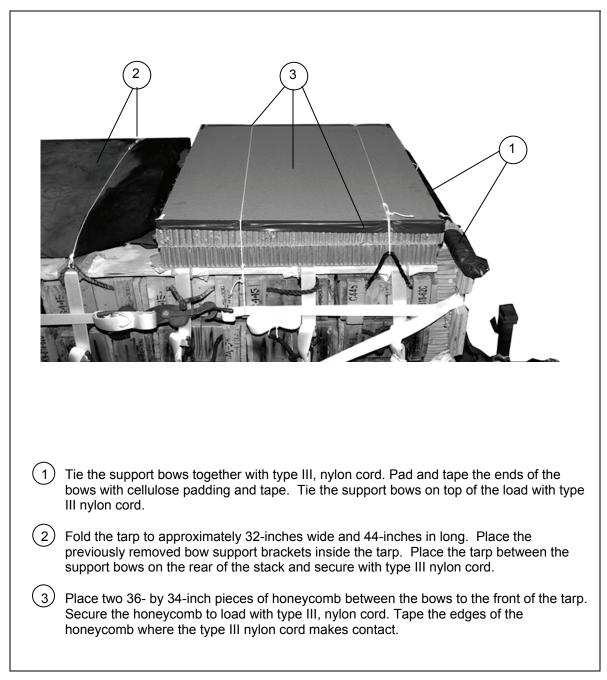
Figure 3-15. Support Bows and Tarp Positioned and Secured
