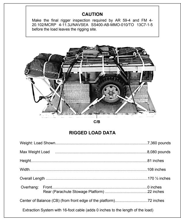
Figure 4-20. 1 ½-Ton trailer Rigged on a 12-Foot, Type V Platform for Low-Velocity Airdrop
