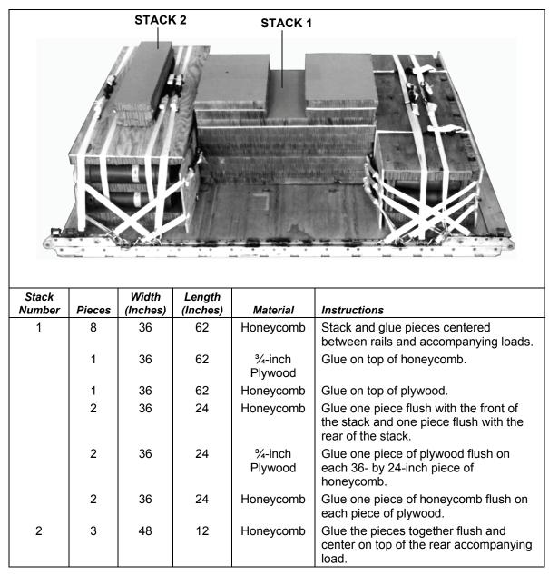
Figure 6-8. Honeycomb Stacks 1 and 2 Built and Positioned
