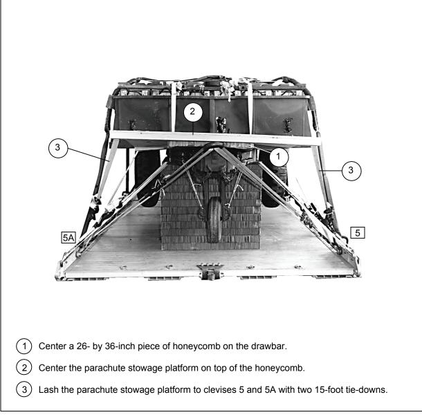
Figure 4-16. Parachute Stowage Platform Installed
