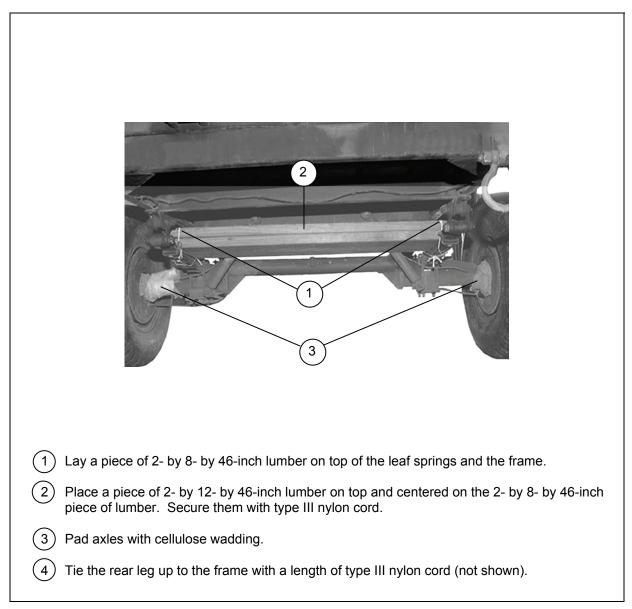
Figure 2-12. Rear of Trailer Prepared
