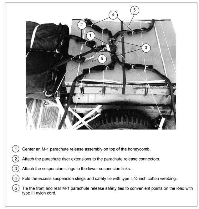
Figure 6-18. M-1 Parachute Release Installed
