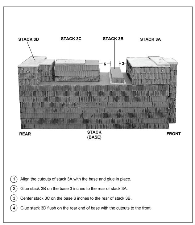
Figure 7-5. Stack 3 Assembled
