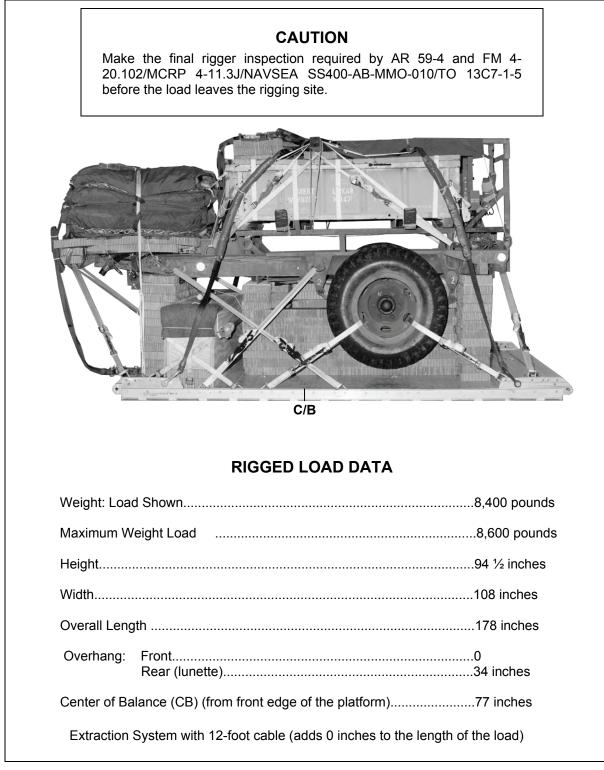
Figure 7-18. MICLIC on 2 <sup>1</sup>/<sub>2</sub>-Ton Trailer Rigged on a 12-Foot, Type V Platform for Low-Velocity Airdrop
