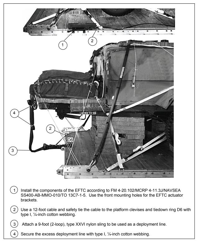
Figure 10-15. Extraction System Installed
