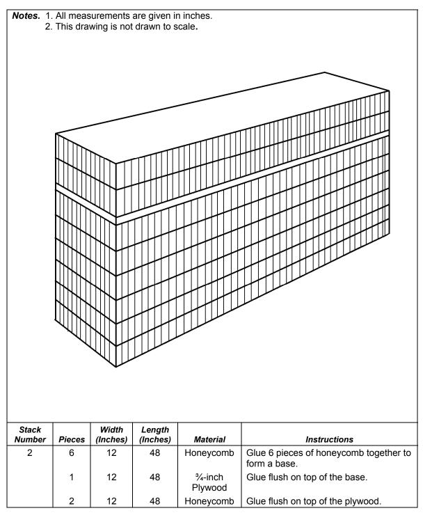
Figure 4-4. Honeycomb Stack 2 Prepared
