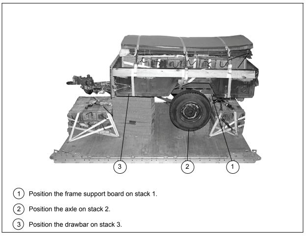
Figure 2-17. Trailer Positioned
