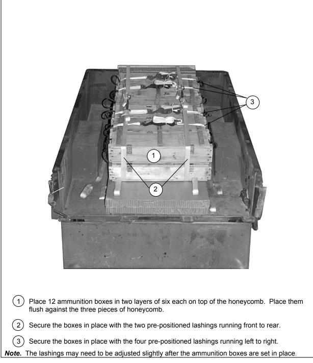
Figure 2-14. Ammunition Boxes Lashed and Secured in the Trailer
