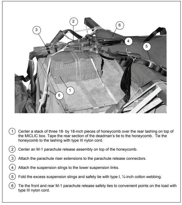
Figure 7-16. M-1 Parachute Release Installed
