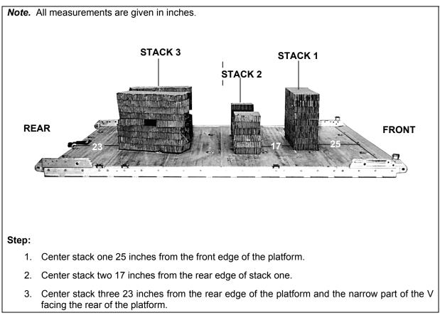
Figure 10-5. Honeycomb Stacks Positioned on Platform
