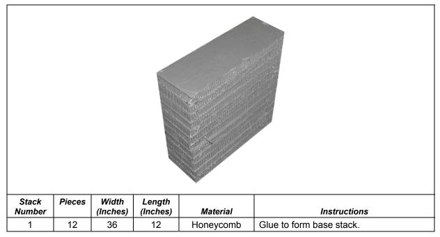
Figure 2-7. Honeycomb Stack Number I Prepared
