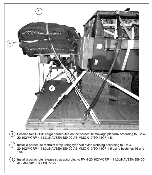
Figure 3-24. Cargo Parachutes Positioned and Restrained
