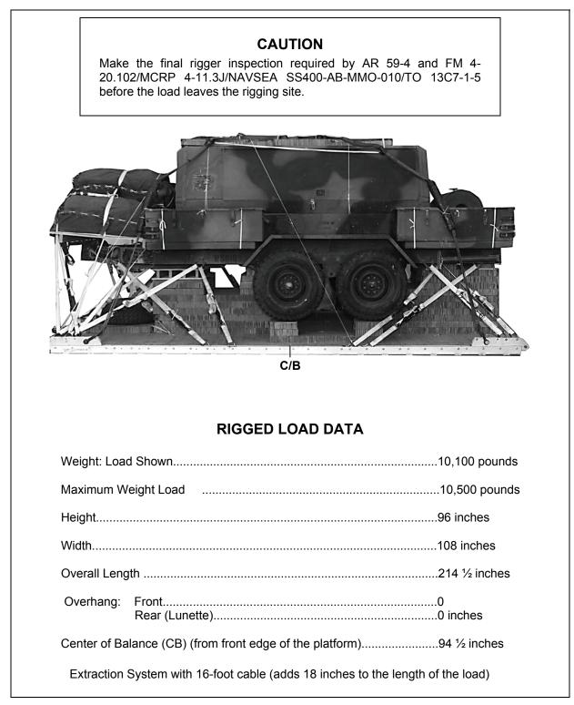
Figure 9-27. Ingersol-Rand Model, 250-CFM, Trailer-Mounted Air Compressor Rigged on a 16-Foot, Type V Platform for Low-Velocity Airdrop
