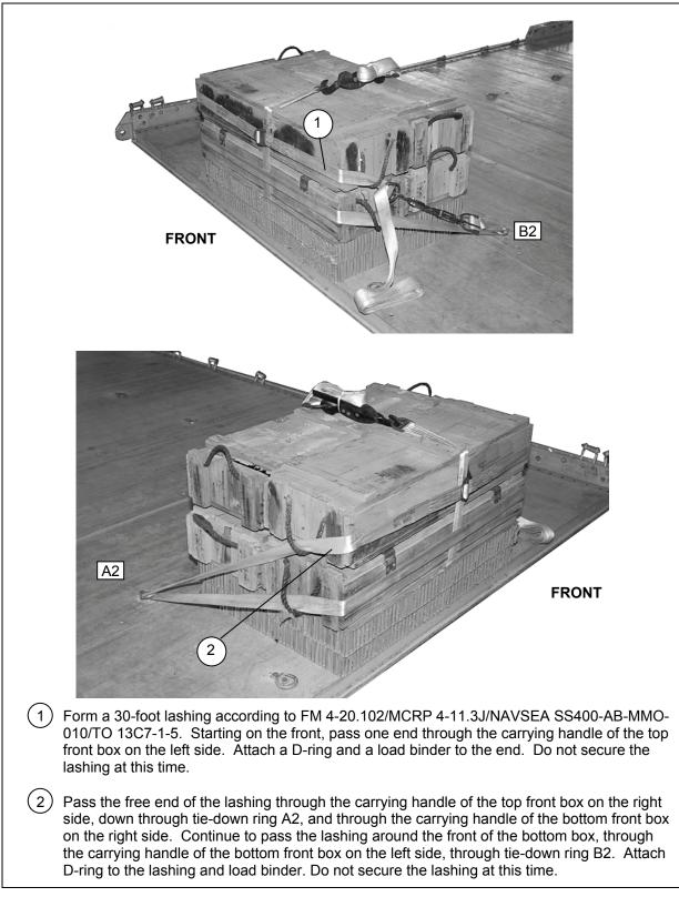
Figure 2-4. Ammunition Boxes Lashed and Secured on the Front of the Platform
