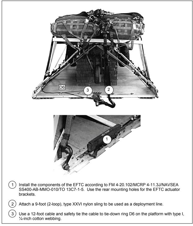
Figure 4-19. Extraction System Installed
