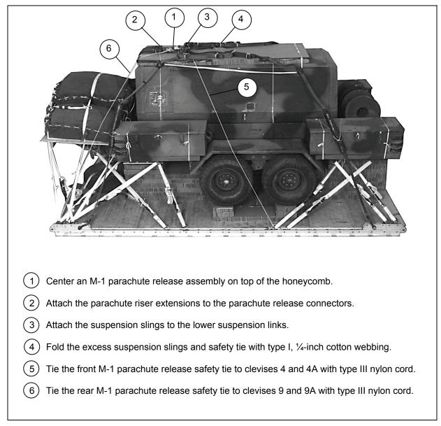
Figure 9-25. M-1 Parachute Release Installed
