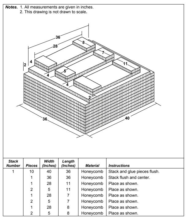
Figure 5-3. Honeycomb Stack 1 Prepared
