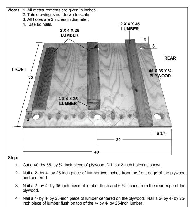
Figure 3-21. Parachute Stowage Platform Built
