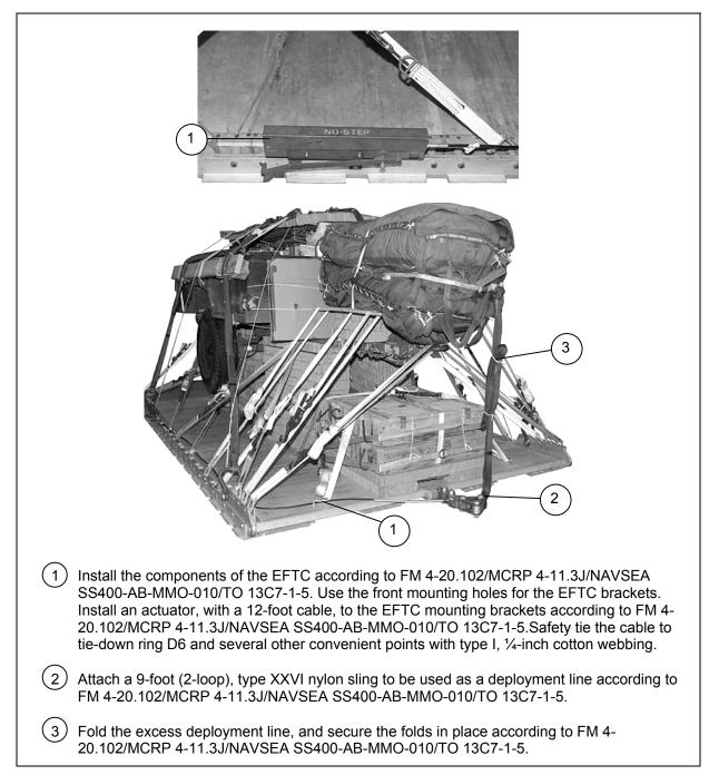
Figure 2-24. Extraction System Installed
