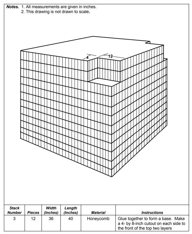
Figure 4-5. Honeycomb Stack 3 Prepared
