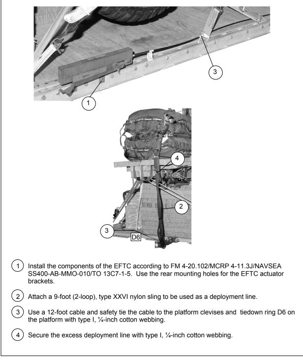
Figure 7-17. Extraction System Installed
