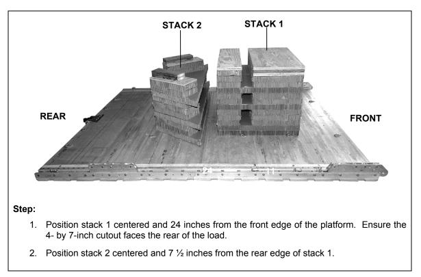
Figure 3-5. Honeycomb Stacks Positioned on Platform
