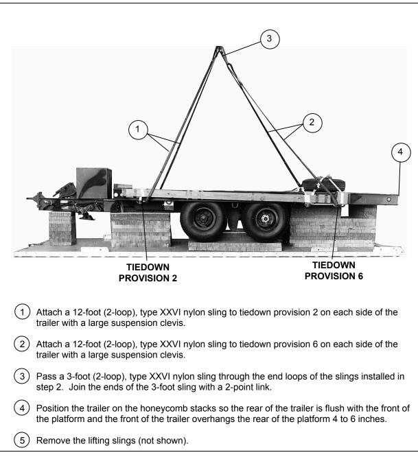
Figure 8-13. Trailer Lifted and Positioned on Platform
