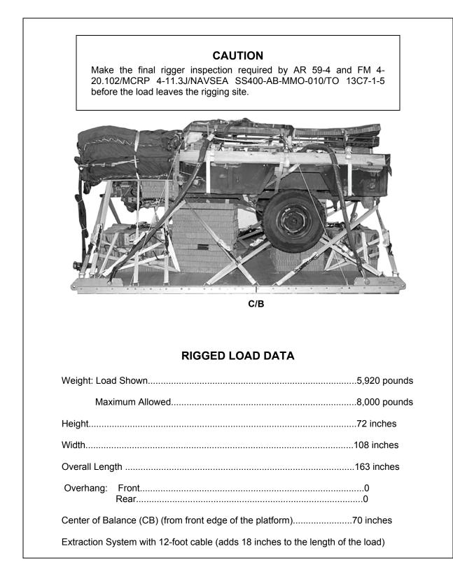
Figure 2-25. M101A2, <sup>3</sup>/<sub>4</sub>-Ton Trailer and Accompanying Load on a Type V Platform Rigged for Low-Velocity Airdrop
