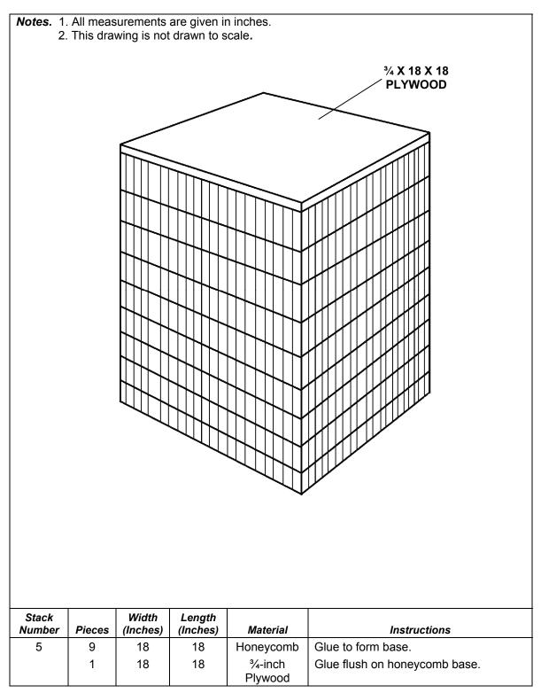
Figure 8-6. Stack 5 Built
