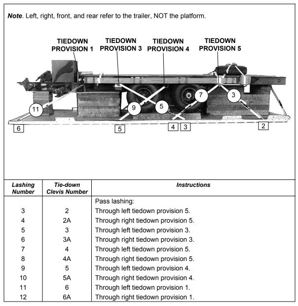
Figure 8-15. Lashings 3 through 12 Installed
