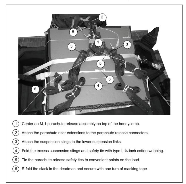
Figure 3-25. M-1Parachute Release Installed
