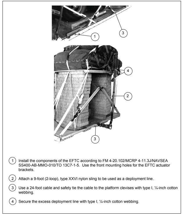
Figure 8-23. Extraction System Installed
