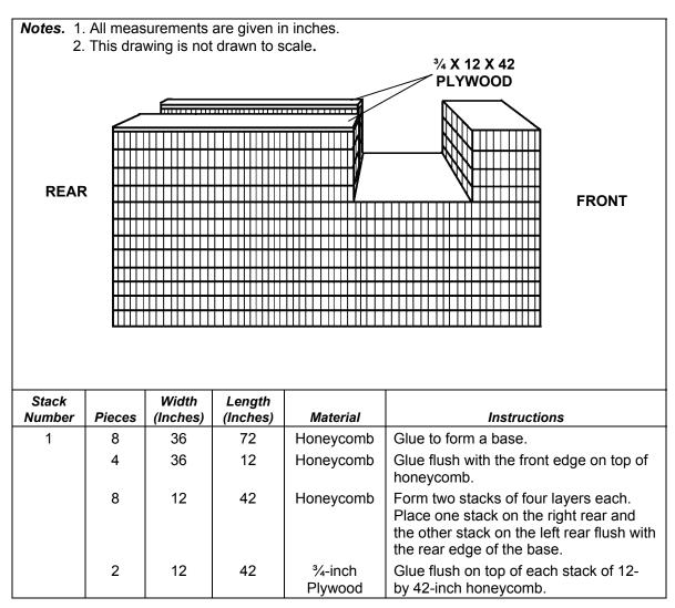
Figure 8-3. Honeycomb Stack 1 Built
