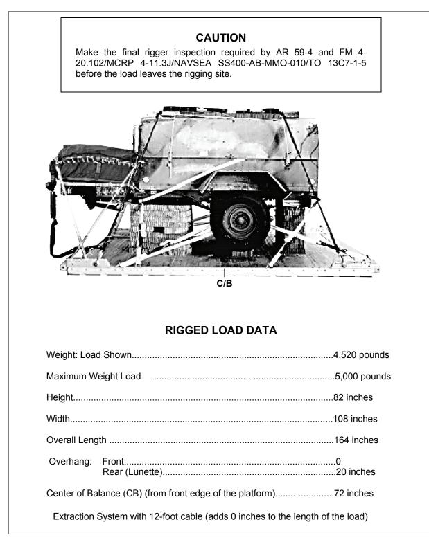
Figure 10-16. Trailer-Mounted Engineer Electrical Tool Outfit Rigged on a 12-Foot, Type V Platform for Low-Velocity Airdrop
