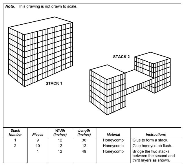
Figure 10-3. Honeycomb Stack 1 and 2 Built
