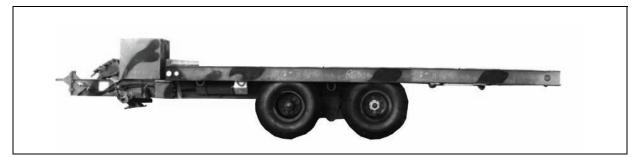
Figure 8-1. 15-Ton Tilt Bed Trailer
