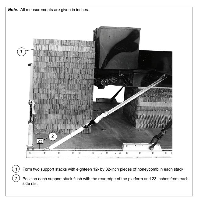
Figure 8-18. Parachute Stowage Platform Support Stacks Prepared
