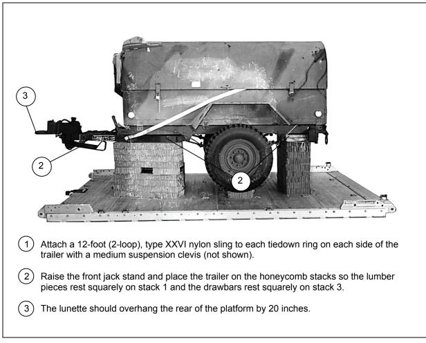
Figure 10-9. Trailer Lift Slings Installed
