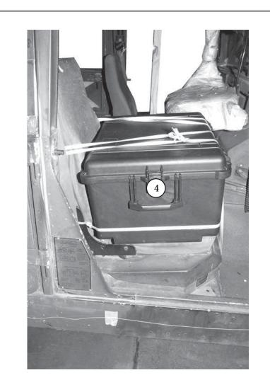
) Place the transit case in the passenger seat and secure to the seat with 1/2-inch tubular nylon webbing.
