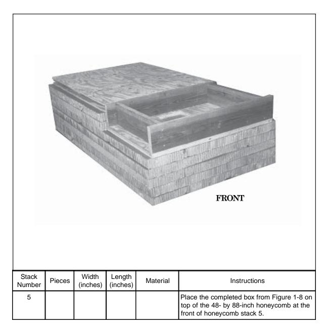
Figure 1-8. Box for Honeycomb Stack 5 Prepared (Continued)
