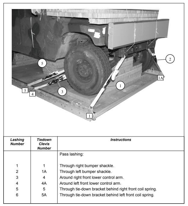
Figure 2-14. Lashings 1 through 6 Installed
