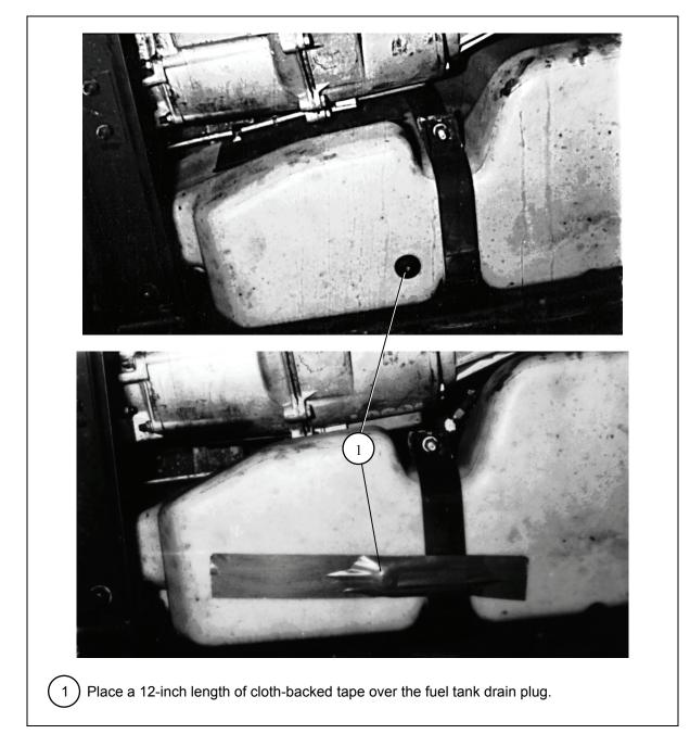
Figure 1-8. Fuel Tank Drain Plug Prepared
