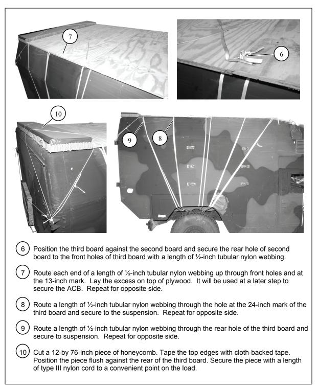
Figure 2-12. Roof Cover Installed (Continued)
