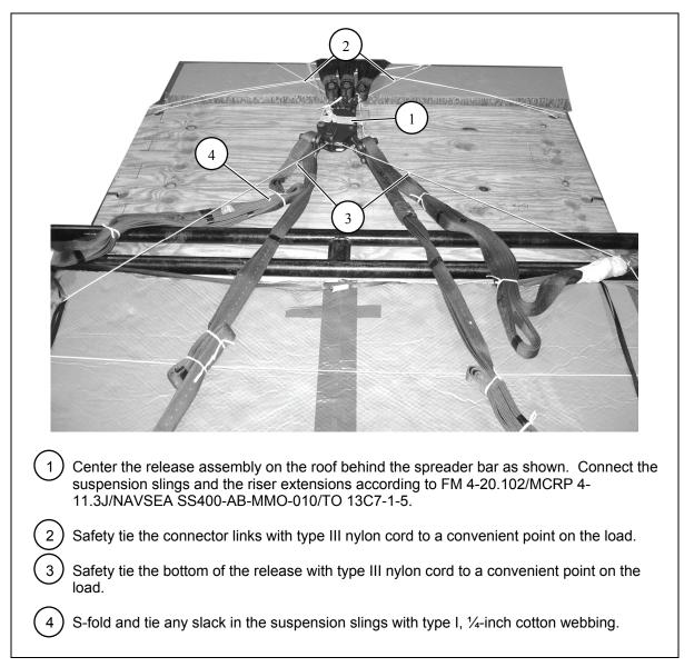
Figure 1-27. M-1 Release Installed
