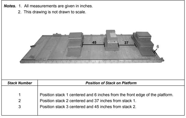
Figure 2-3. Honeycomb Stacks Placed on Platform
