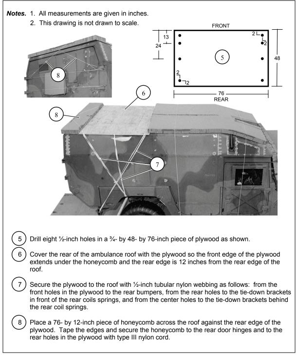
Figure 1-19. Roof Cover and ACB Supports Installed (Continued)
