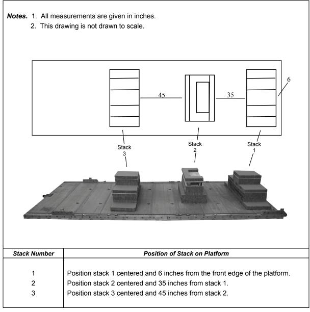
Figure 1-5. Honeycomb Stacks Placed on Platform
