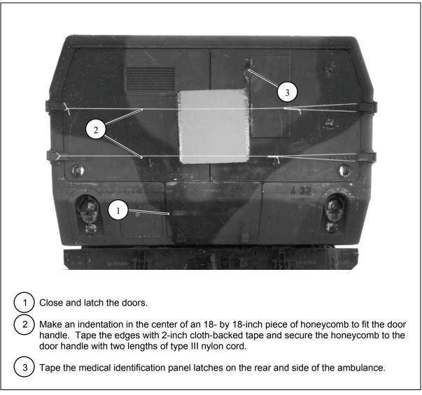
Figure 1-14. Doors Secured and Latches Covered
