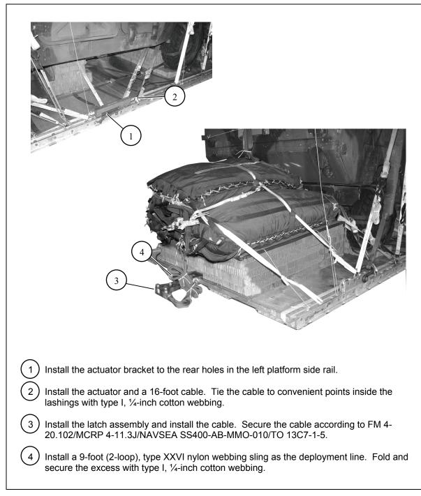
Figure 1-26. EFTC Installed
