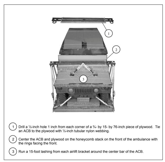
Figure 1-20. ACB Installed on Front of Ambulance
