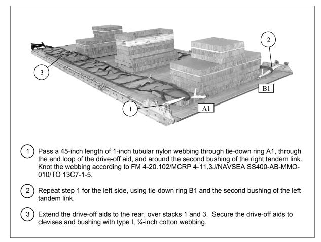
Figure 1-6. Drive-Off Aids Installed on Platform
