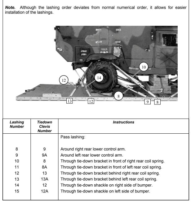
Figure 1-18. Lashings 8 through 15 Installed
