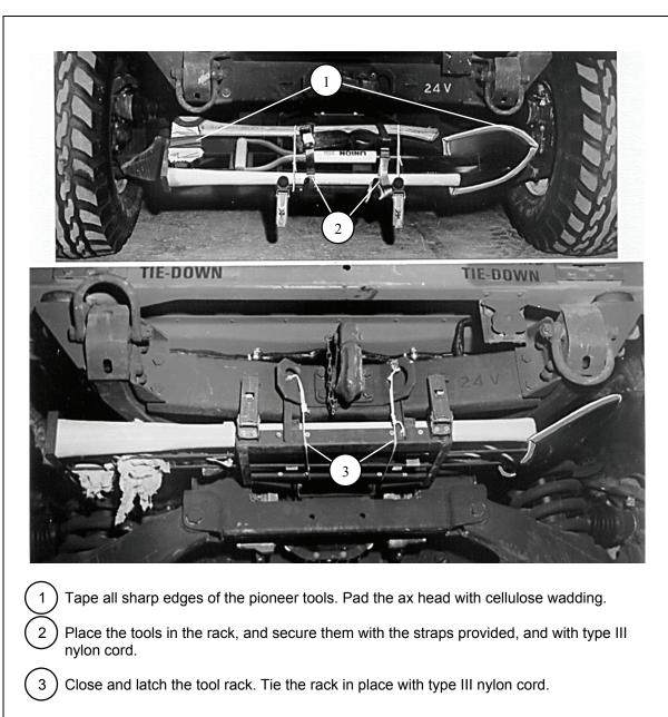
• Prepare and secure the pioneer tool kit according to TM 9-2320-280-10/TO 36A12-1A-2091-1/TM 2320-10/6, and as shown in Figure 1-12.
