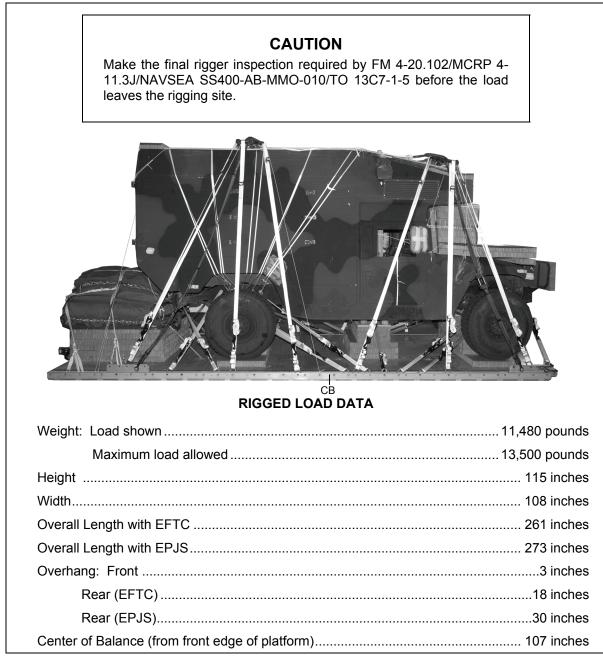
Figure 2-22. M997, 4-Litter Ambulance Rigged for Low-Velocity Airdrop
