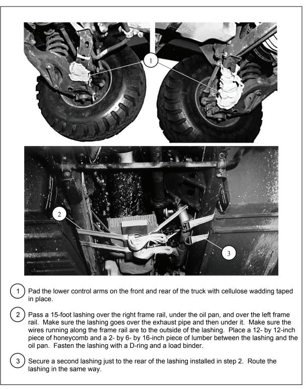
• Prepare the underside of the truck as shown in Figure 1-10.
