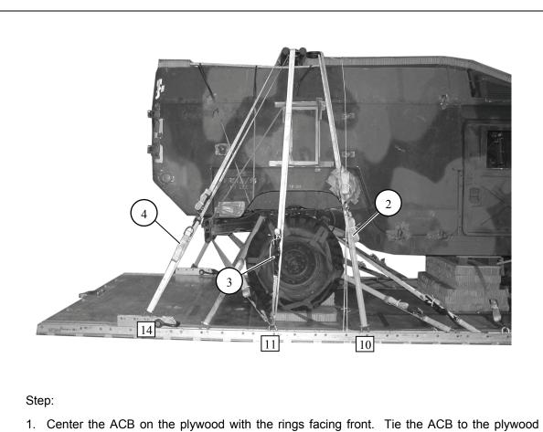
Install and lash the rear ACB to the platform as shown in Figure 1-22. •
