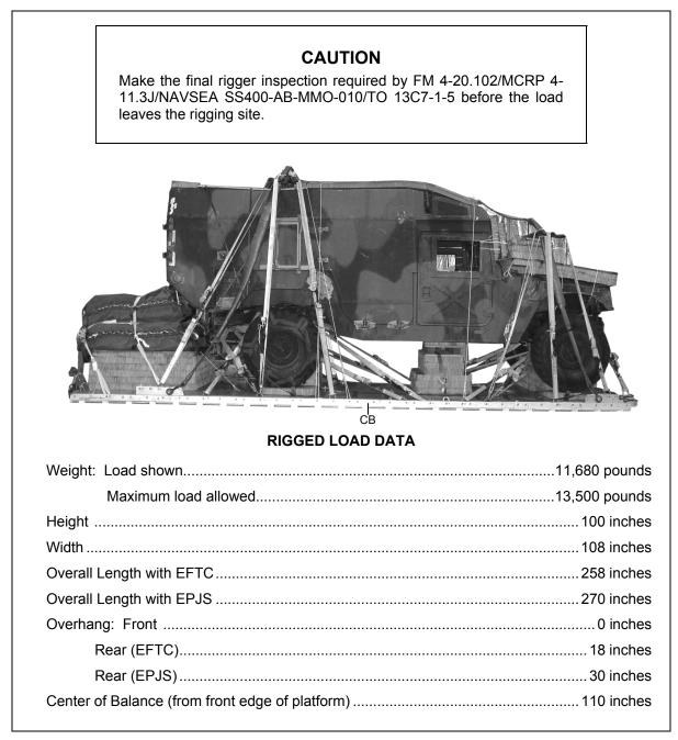
Figure 1-28. M996, 2-litter Armored Ambulance (HMMWV) Rigged for Low-Velocity Airdrop
