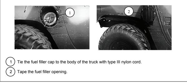
Figure 1-7. Fuel Tank Filler Cap and Opening Prepared
