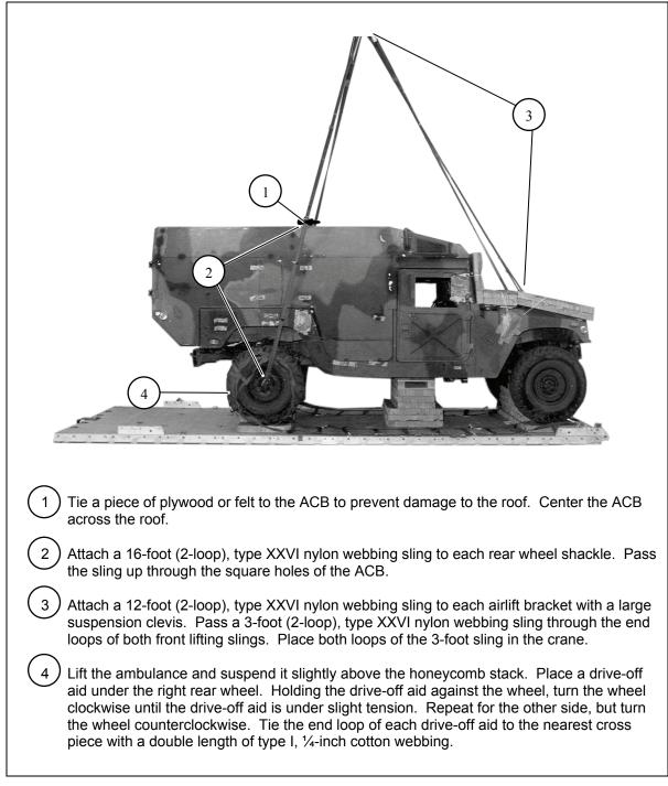
Figure 1-15. Lifting Slings Installed, Ambulance Lifted, and Drive-off Aids Installed
