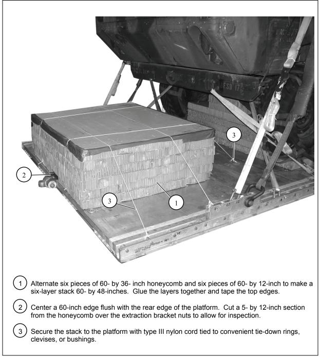
Figure 1-24. Parachute Stowage Platform Prepared and Installed
