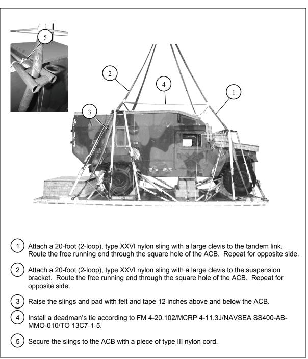
• Install the suspension slings and the deadman's tie as shown in Figure 1-23.
