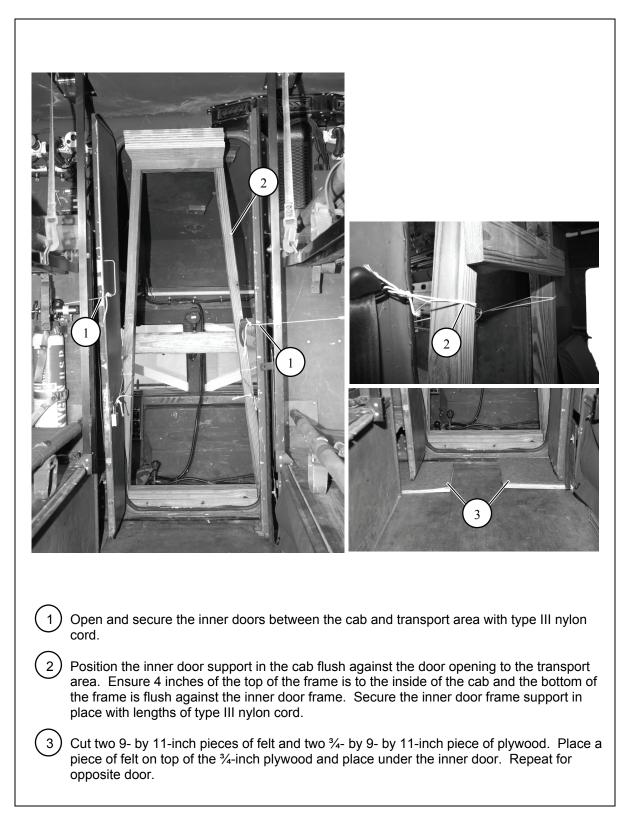
Figure 2-5. Inner Door Support Positioned
