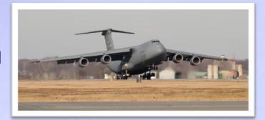
operations. The C-5M is an upgraded version of the C-5 Galaxy, complete with a modernized glass cockpit and upgraded engines and avionics.
