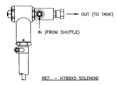
The reported delayed activation was remedied by replacement of the original L-H788X5 solenoid with Bucyrus' Solenoid Kit #241103.
