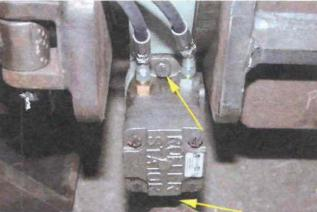
BOLTS TO BE TIGHTENED ON WORM GEAR TILT BOX
