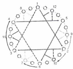
NOTE: USE A STAR SHAPED TIGHTENING SEQUENCE WHEN TIGHTENING BOLTS.
