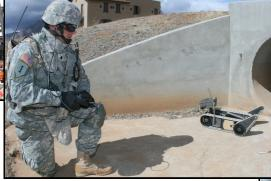
Searching culvert with Small Unmanned Ground Vehicle
