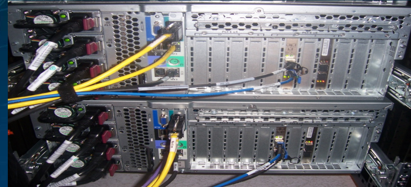
10G uses 802.1q trunking and twinax cabling
