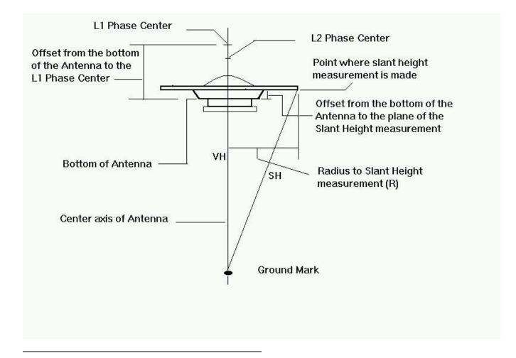
Radius to Slant Height Measurement (R): This is the horizontal distance from the vertical center axis of the antenna to the point where the slant height measurement (SH) is made.
