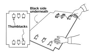
**9** Cover the thumbtacks with thin strips of duct tape to prevent them from falling out of the cardboard.
