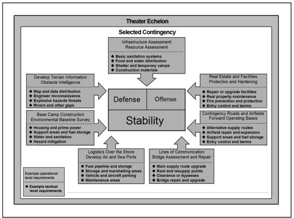
Figure 5-1. Contingency perspective of engineer requirements
