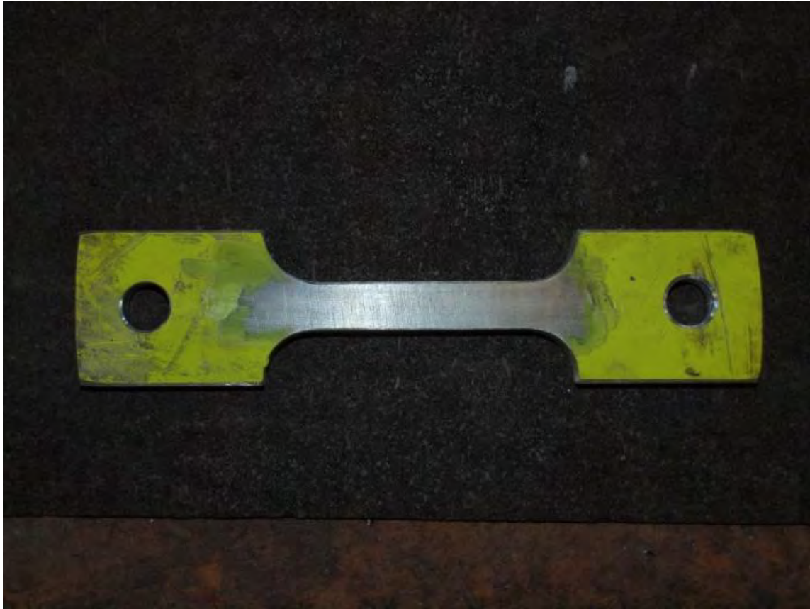
Figure 30. View of the tensile specimen machined from the incident tank.
