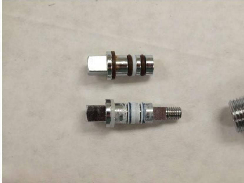
Figure 16. View of the incident valve stem (top) as compared to the exemplar valve stem.
