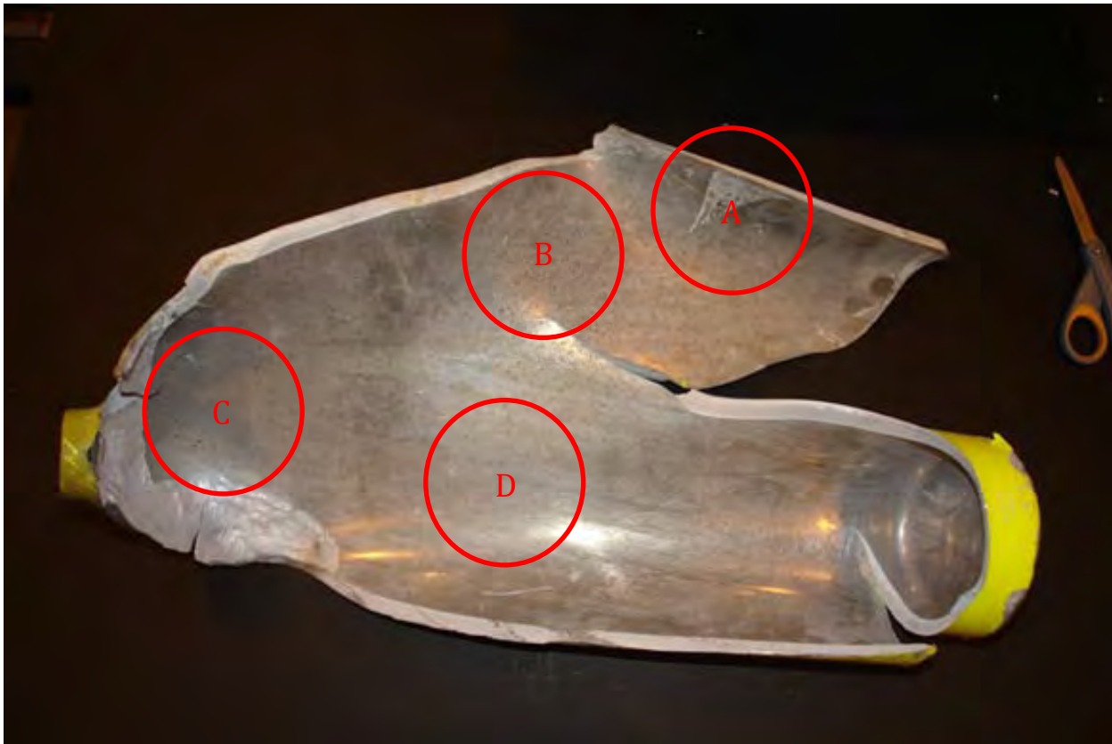
Figure 1. Solvent was areas for FTIR sampling.
