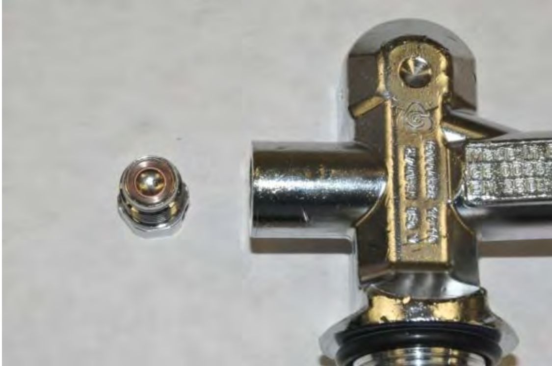
Figure 12. View of the exemplar pressure burst disk assembly showing the burst disk and retaining ring.
