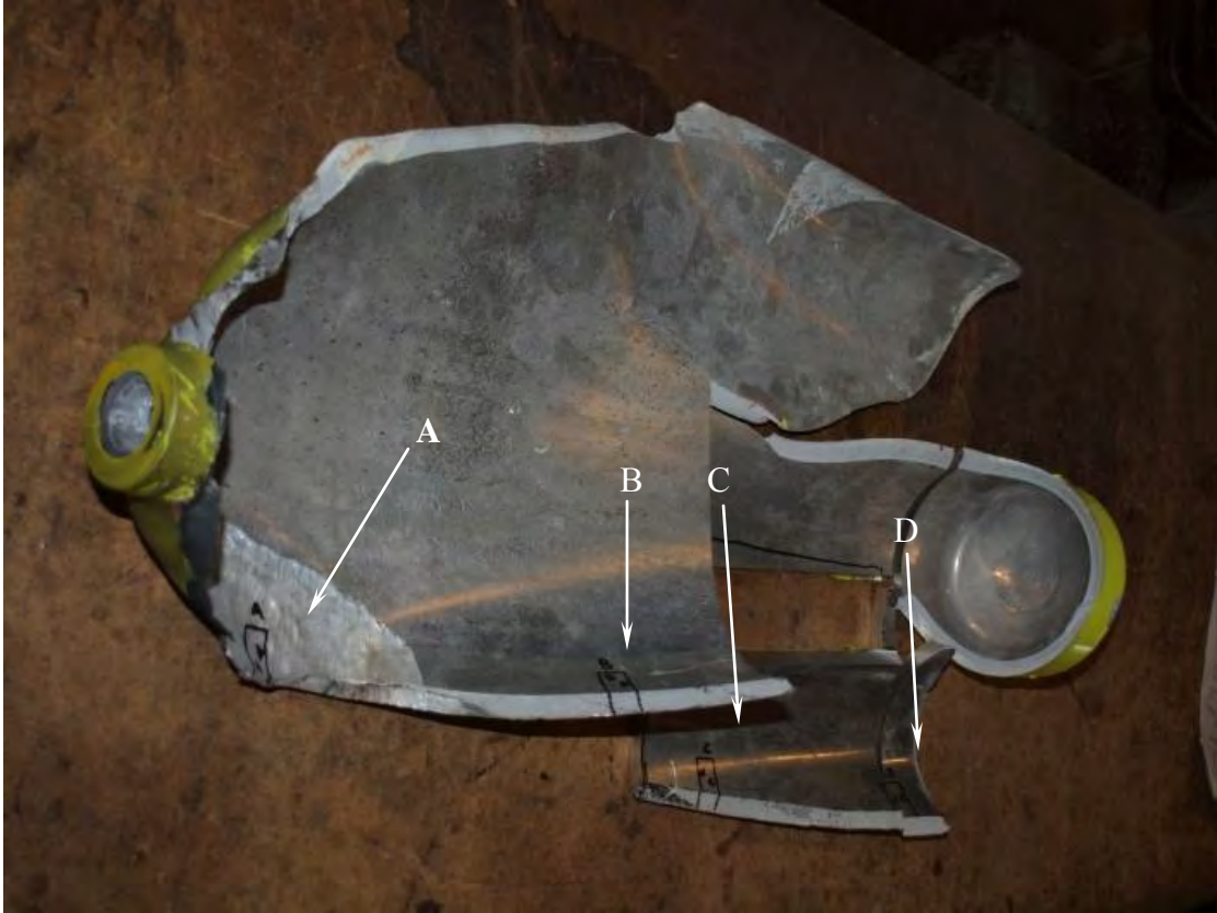
Figure 29. View of the incident cylinder showing the locations of the four metallography/microhardness specimens.
