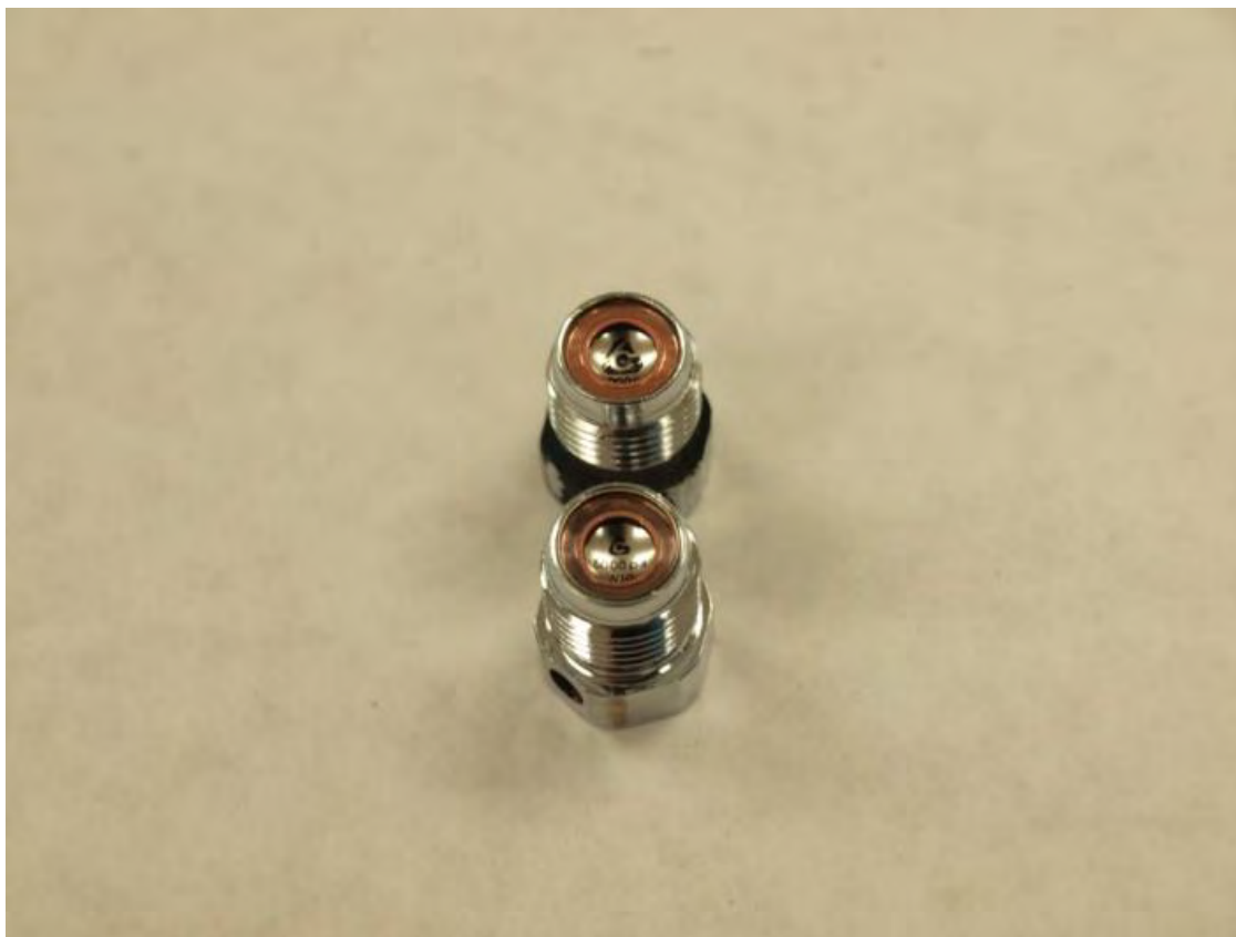
Figure 18. View of the incident burst disk assembly (upper) as compared to the exemplar burst disk assembly (lower).
