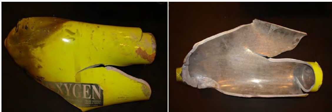
Figure 4. Larger portion of high pressure gas cylinder
