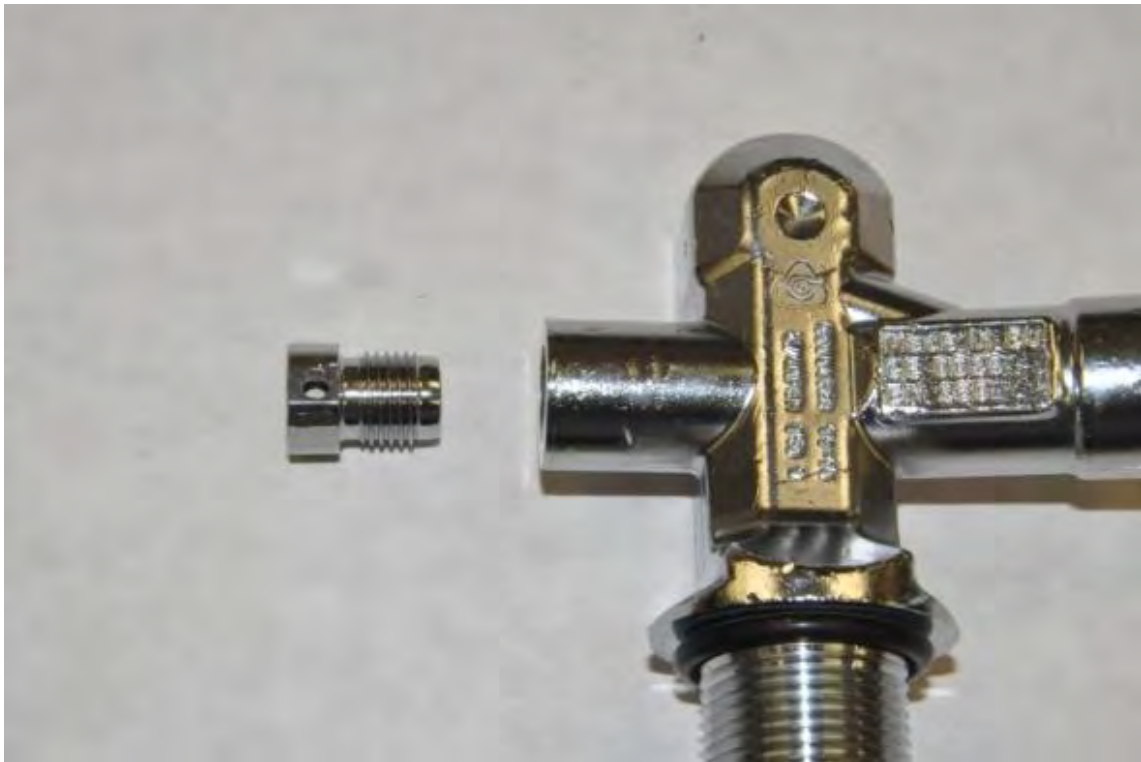
Figure 11. Rear view of the exemplar pressure burst disk assembly as removed from the valve body.
