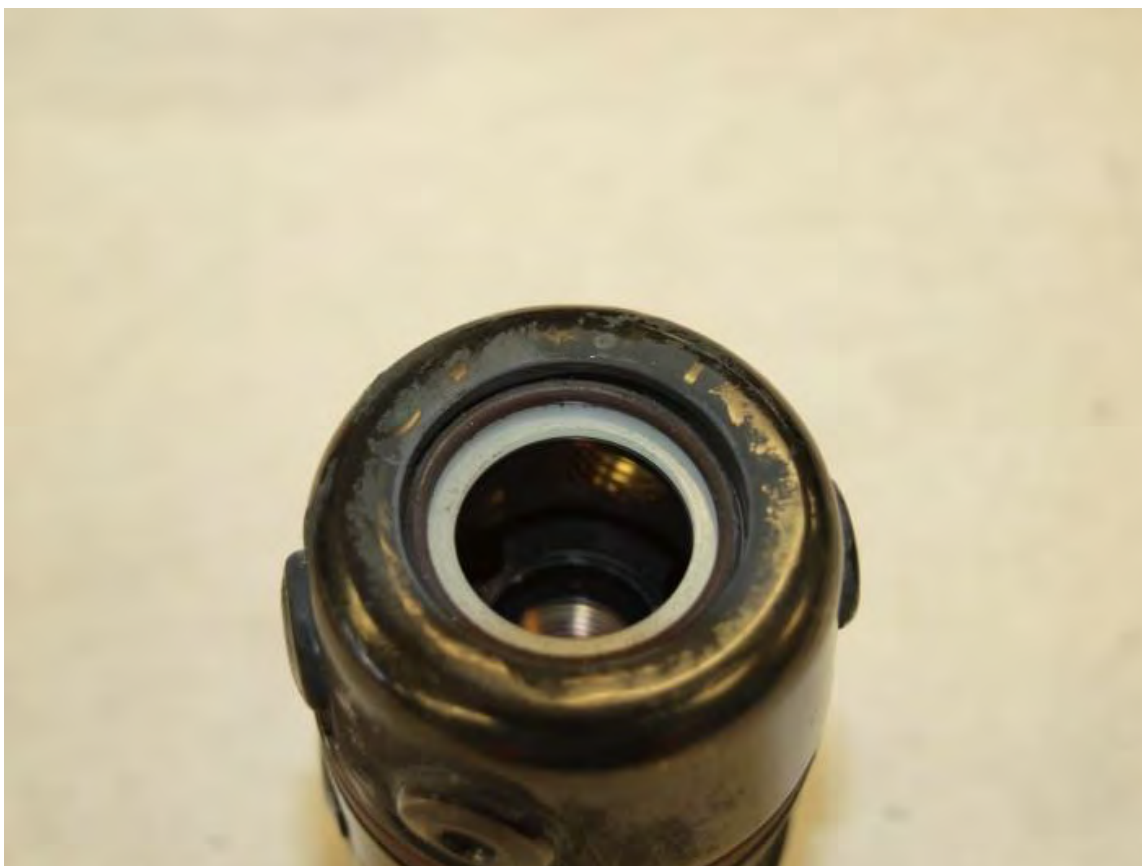
Figure 22. View into the low pressure portion of the incident regulator showing the O-ring and washer.
