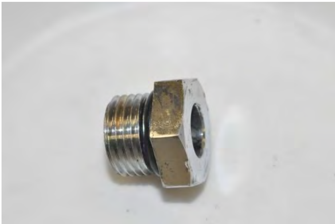
Figure 15. View of the incident cylinder valve gland nut showing the presence of the intact O-ring.
