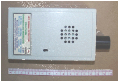
FIGURE 24 (LEFT): HANDHELD RECEIVER FOR THE RELUME DEVICE; PROVIDES A SPEECH OR TACTILE MESSAGE TO PEDESTRIAN WHEN IT IS POINTED AT THE PEDHEAD.
