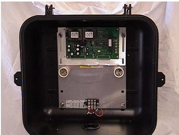
FIGURE 3: CAMPBELL CONTROL UNIT INSTALLED A 16 INCH PEDHEAD.
