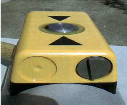
FIGURE 5: GEORGETOWN PUSHBUTTON SEEN FROM BOTTOM, SHOWING VIBRATING ARROW LOCATION.
