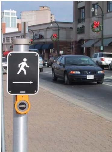
FIGURE 13: POLARA NAVIGATOR UNIT INSTALLED ON A STUB POLE IN SILVER SPRING, MD.
