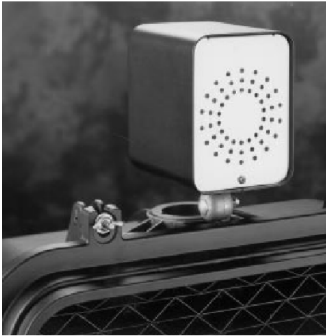
FIGURE 29: PHOTO OF THE US TRAFFIC DEVICE MOUNTED ON TOP OF A PEDESTRIAN SIGNAL HEAD.
