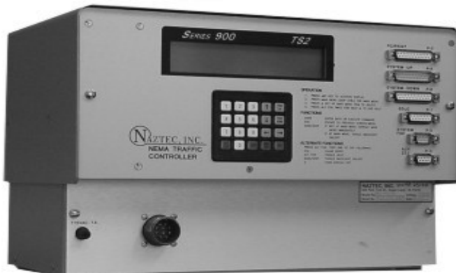
FIGURE 38. NAZTEC SERIES 900 TS 2 CONTROLLER SHOWING KEYPAD FOR ENTERING INFORMATION AND WIRING CONNECTIONS.
