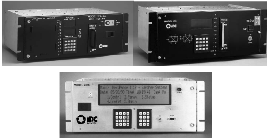
FIGURE 46 (UPPER LEFT). US TRAFFIC 170 CONTROLLER SHOWING KEYPAD FOR ENTERING INFORMATION AND WIRING CONNECTIONS.
