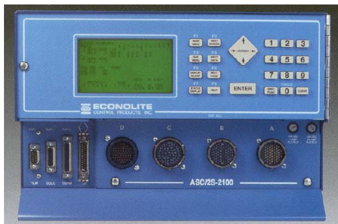
FIGURE 36. ECONOLITE ASC/2S-2100 CONTROLLER SHOWING KEYPAD FOR ENTERING INFORMATION AND WIRING CONNECTIONS.
