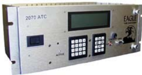
FIGURE 42. EAGLE 2070 ATC CONTROLLER SHOWING KEYPAD FOR ENTERING INFORMATION AND WIRING CONNECTIONS.
