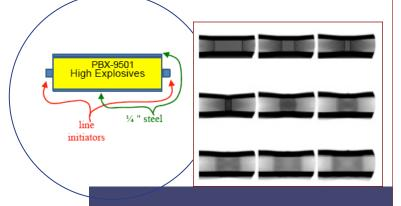
800 meV proton radiography has been used to diagnose HE burn characteristics and the equation of state of the resulting HE detonation products. In a recent experiment, a piece of HE is line-initiated at each end. pRad images the detonation fronts as they approach each other in the explosives and, after pass each other, characterizes the shocks traversing the detonated HE products.
