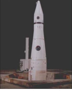
Exoatmospheric Reentry Vehicle Interceptor Subsystem (ERIS)
