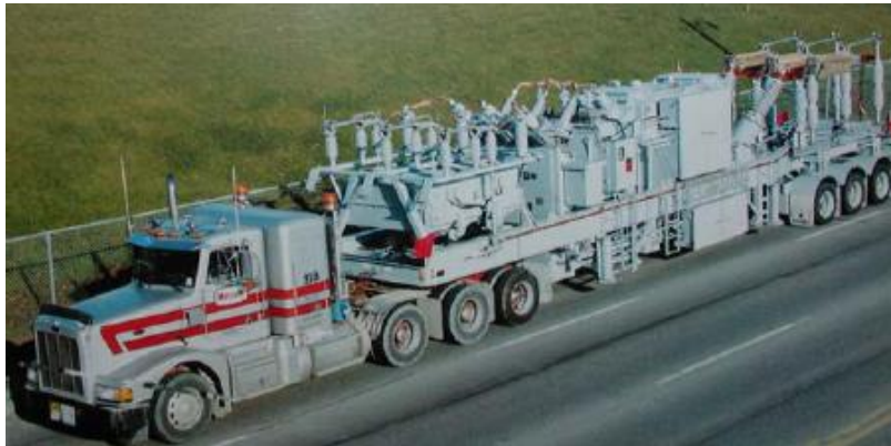
Figure 25. Trailer-Mounted Mobile Transformer
