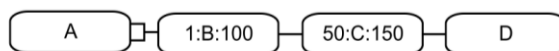
Figure 86: Recommended method for laying out entity features. Entity features B and C overlap in position, and semantically the assertion is made that entity feature D exists after entity feature C though its location is not represented.
