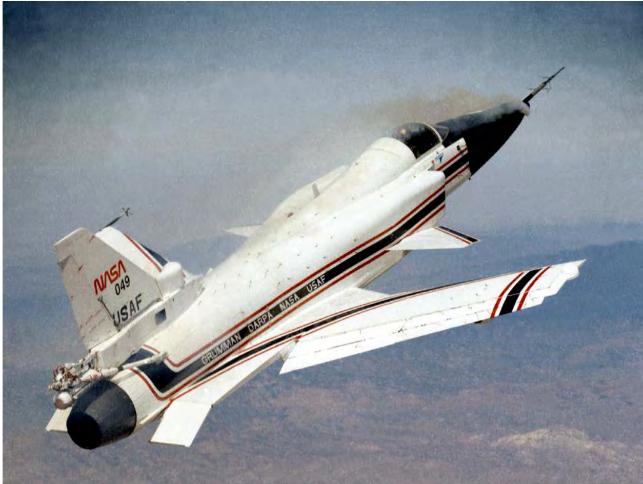
Figure 3-24. This photo shows the X-29 during a September 1991 research flight. Smoke generators in the nose of the aircraft were used to help researchers see the behavior of the air flowing over the aircraft. The smoke here is demonstrating forebody vortex flow (NASA photo EC91-491-6).
