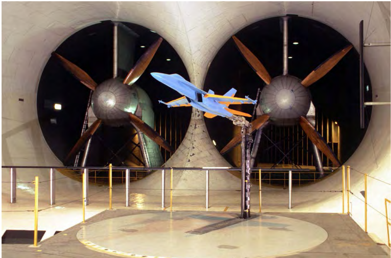
Figure 3-16. This photo shows a 1.5 percent High-Speed Research Technology Concept Aircraft (TCA) baseline aft body model in Langley's 16-foot transonic tunnel (NASA photo EL-1999-00196).
