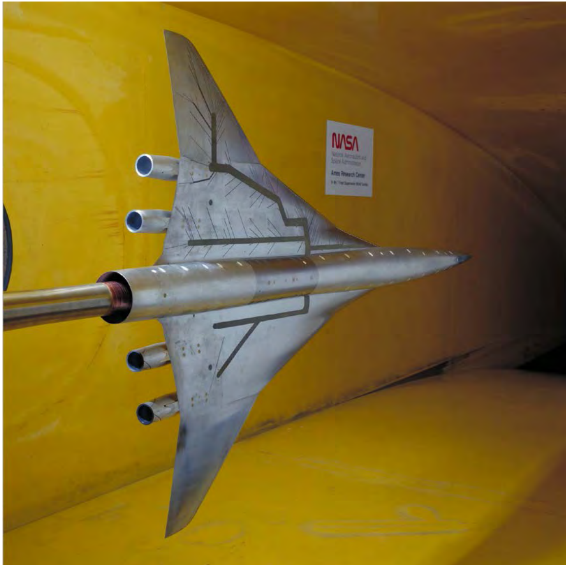
Figure 3-35. A series of High-Speed Civil Transport wind-tunnel tests were conducted using the 9- by 7-foot tunnel from December 1993 to February 1994. (NASA-ARC Photo AC94-0057-7).
