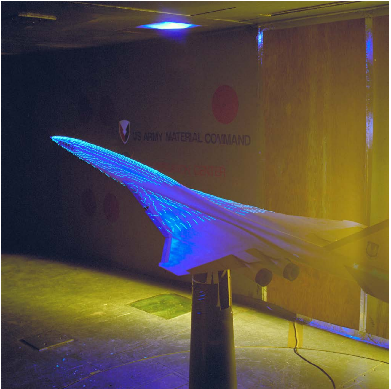
Figure 3-33. This photo shows the Boeing High-Speed Civil Transport being tested in ultraviolet light with tufts in the no. 1 7- by 10-foot wind tunnel. (NASA-ARC photo AC96-0047-47).
