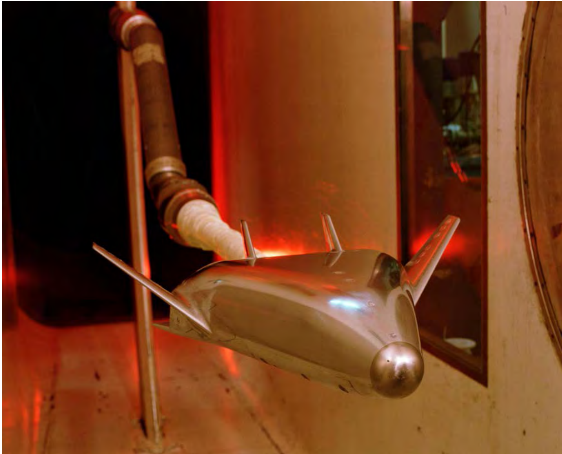
Figure 3-42. The photo shows a metal model of the X-33 reusable launch vehicle (about 15 inches [38 centimeters] long by 15 inches wide) being tested for the Lockheed Martin Skunk Works in Langley's Low-Turbulence Pressure Tunnel. The subsonic tests were conducted at a speed of Mach 0.25. (NASA-LaRC photo EL-1997-00041).
