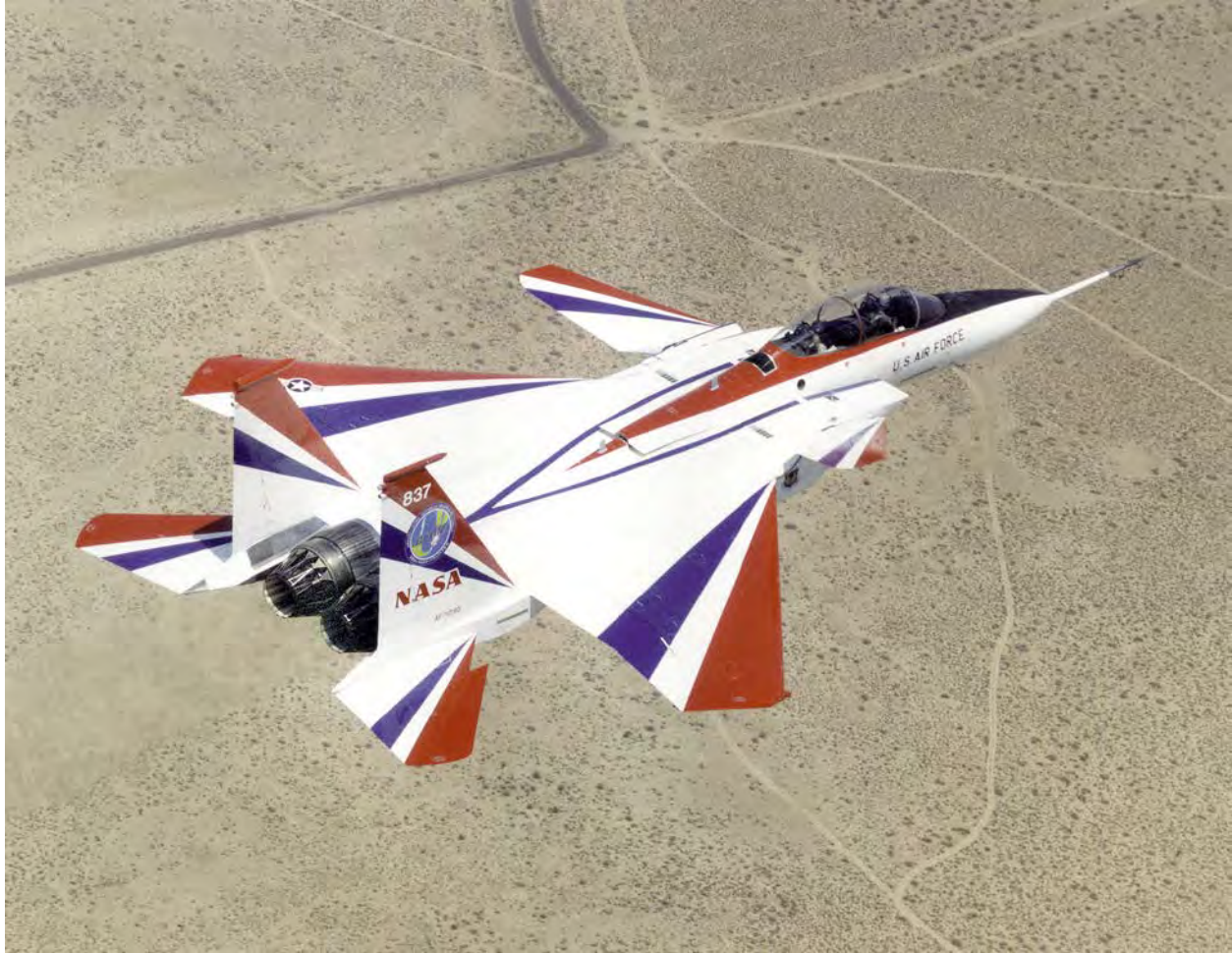
Figure 3-13. The F-15 ACTIVE in flight over the Mojave desert during a High Stability Engine Control (HISTEC) flight. The twin-engine F-15 is equipped with new Pratt & Whitney nozzles that can turn up to 20 degrees in any direction, giving the aircraft thrust control in the pitch and yaw directions. NASA pilot Rogers Smith and photographer Carla Thomas fly the F-18 chase to accompany the flight (NASA photo EC97-44177-15).
