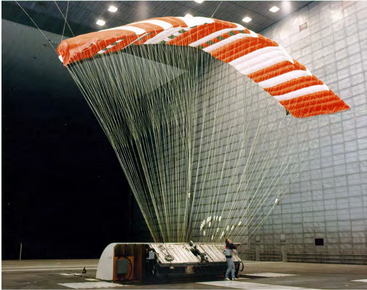
Figure 3-38. The Pioneer Aerospace Parafoil undergoes testing in the world's largest wind tunnel, the 80- by 120-foot tunnel at NASA Ames Research Center, 1990. (NASA HQ-GRIN photo GPN-2000-001646).
