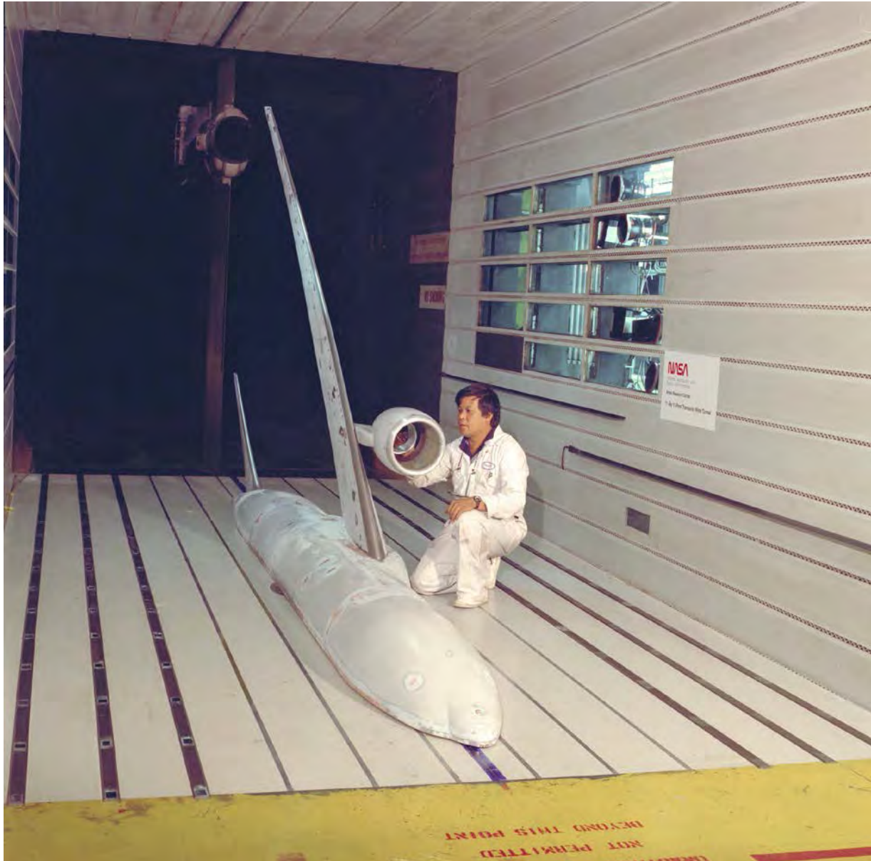
Figure 3-34. A Boeing 777 model in the 11-foot (3.35-meter) wind tunnel during testing in August 1991 (NASA-ARC photo AC91-0470-2).
