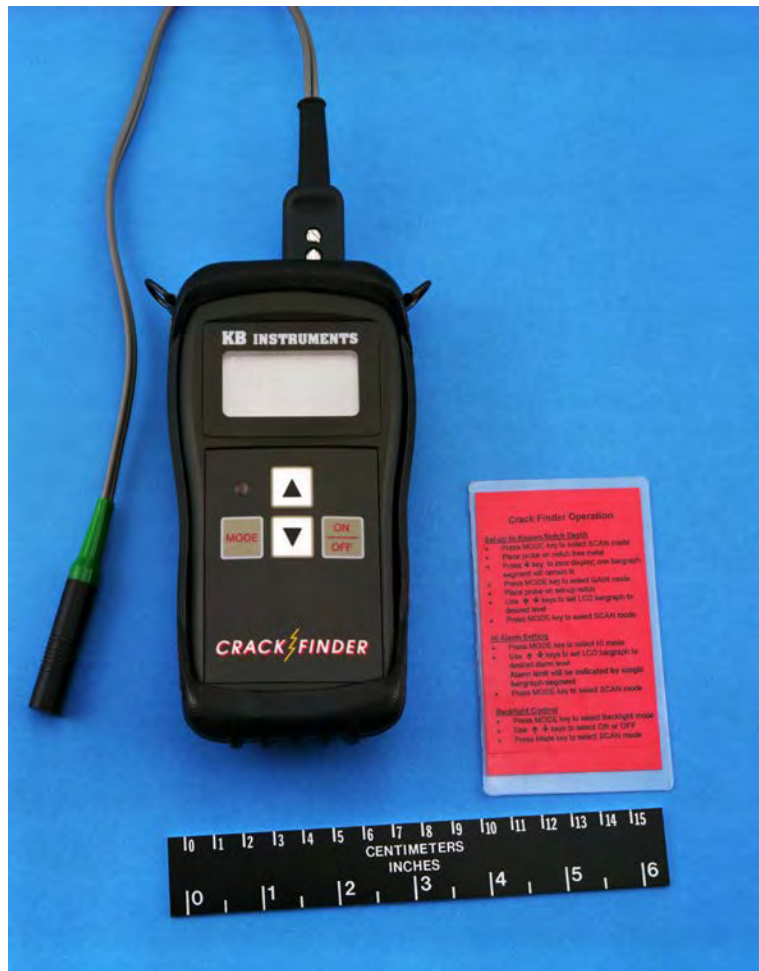
Figure 3-9. The Crack Finder, a commercially available instrument with a 0.5-inch Self-Nulling Eddy Current Probe developed from NASA technology, uses a probe to detect fatigue cracks in conducting materials. The probe technology enables the device to be manufactured in a very small package and eliminates the complicated calibration and test setup procedures commonly required by other eddy-current techniques (NASA-LaRC photo EL-1996-00145).
