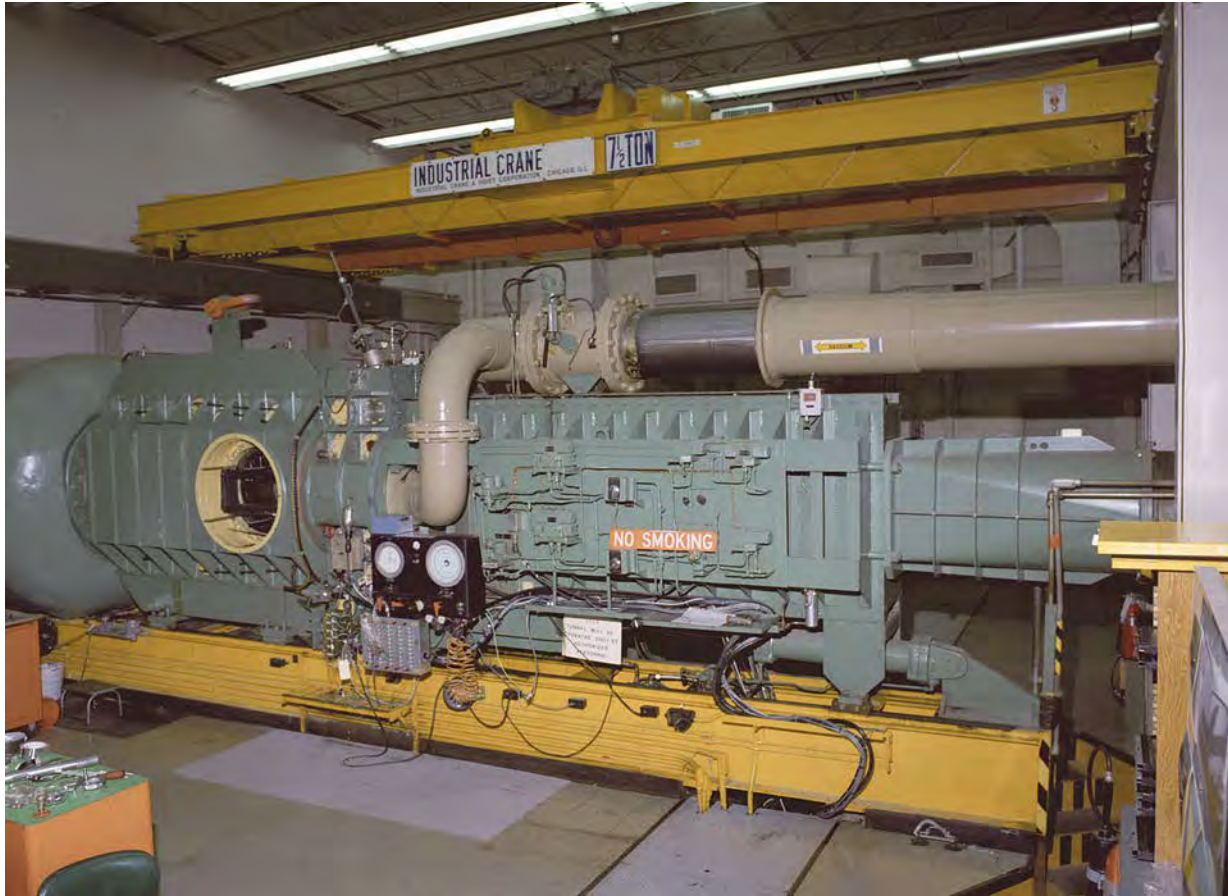
Figure 3-53. This photo shows an overall view of the Marshall 14- by 14-Inch Trisonic Wind Tunnel. It is capable of running at subsonic, transonic, or supersonic speeds (NASA-MSFC photo MSFC-8891417).
