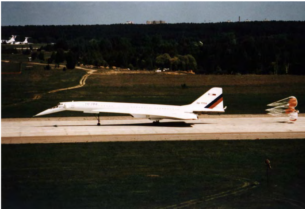
Figure 3-18. The Russian Tu-144LL SST Flying Laboratory landing with drag chutes at the Zhukovsky Air Development Center near Moscow, Russia, in July 1997 (NASA photo no. EC97-44203-2, NASA/IBP).
