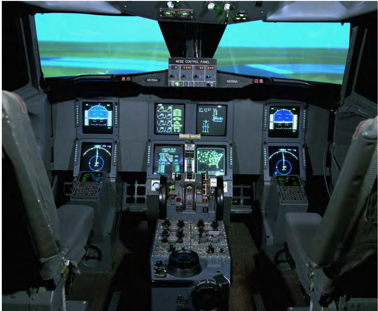
Figure 3-11. This photo shows the eight CRT displays on the Transport Systems Research Vehicle Simulator. The simulator was used as a research tool for projects such as the Cockpit Weather Information (CWIN) displayed on the center lower right CRT (NASA-LaRC photo EL-1996-00095).
