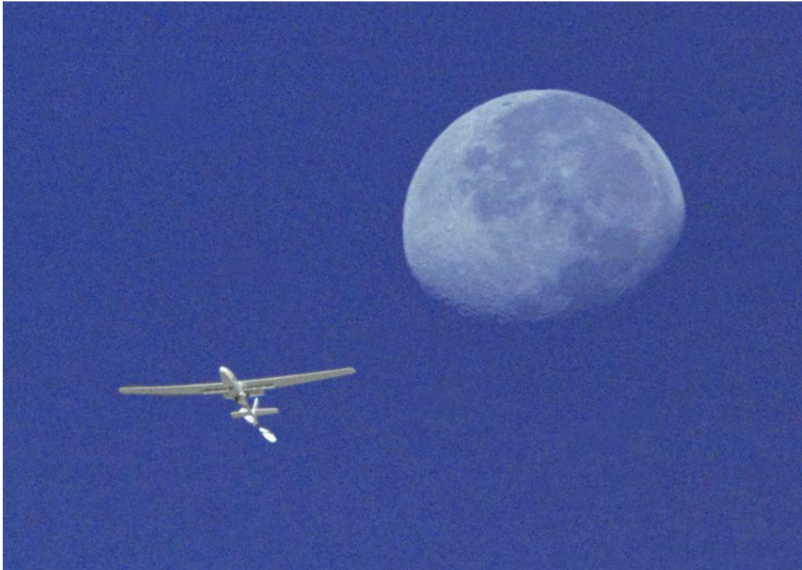
Figure 3-19. The Perseus A, a remotely-piloted, high-altitude research aircraft, is seen here framed against the moon and sky during a research mission at the Dryden Flight Research Center, Edwards, California, in August 1994 (NASA-DFRC photo EC94-42742-7).
