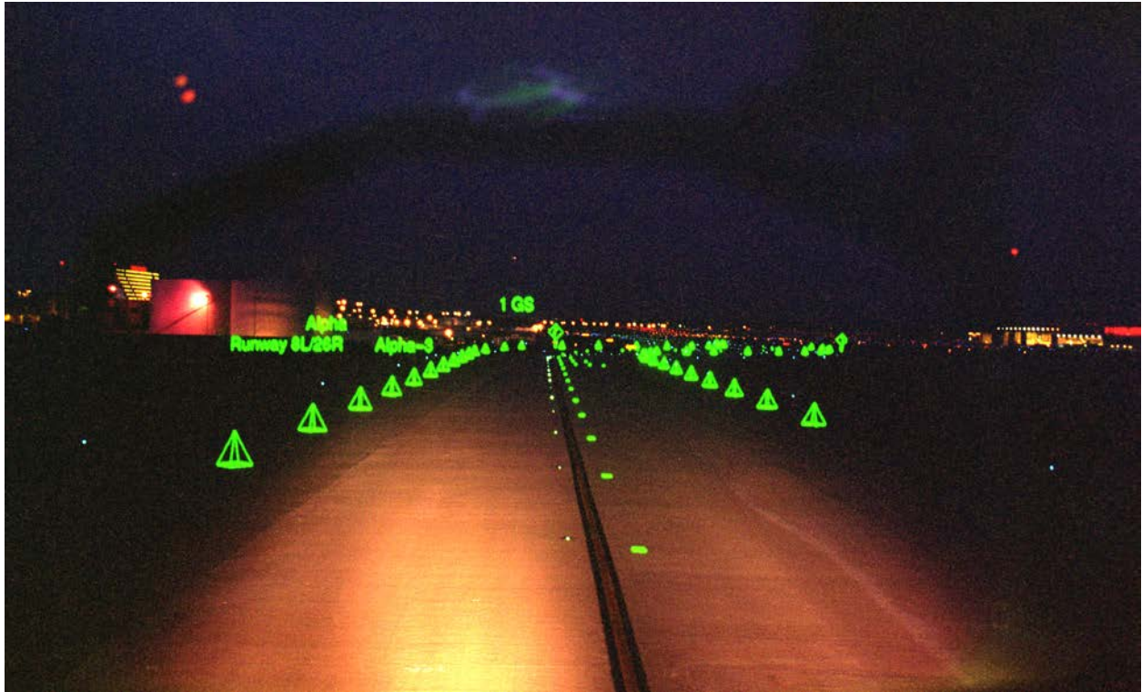
Figure 3-12. This photograph was taken from the cockpit window of NASA's 757 research aircraft during flight demonstration of airport capacity and safety enhancement technologies at Hartsfield-Atlanta International Airport in August 1997. As the 757 approached the runway, computer-generated graphics outlined the correct runway and its precise location on a "head-up display" mounted between the pilot and the windshield (NASA-LaRC photo EL-1998-00111).
