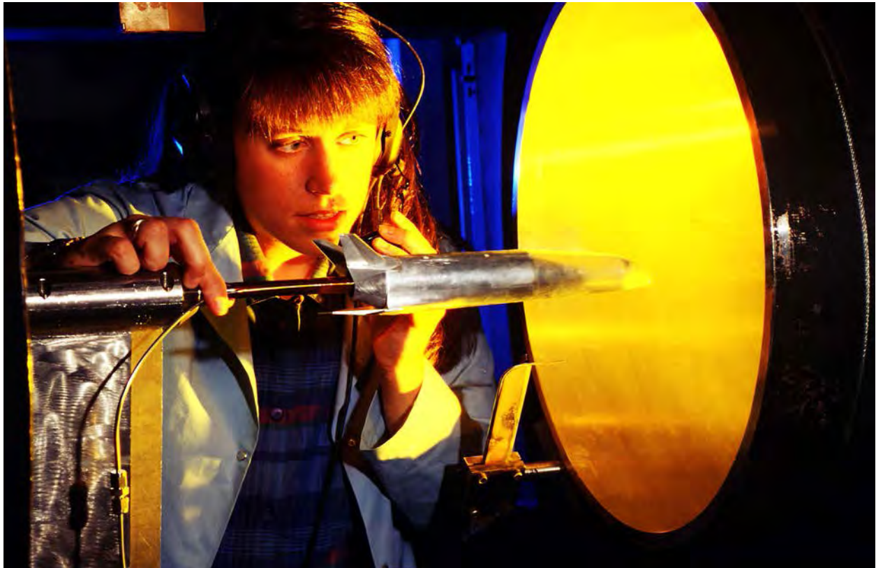
Figure 3-46. A NASA research engineer prepares a Rockwell X-33 model for testing in the Mach 6 CF4 wind tunnel, 1995 (NASA-LaRC photo EL-1996-00160).
