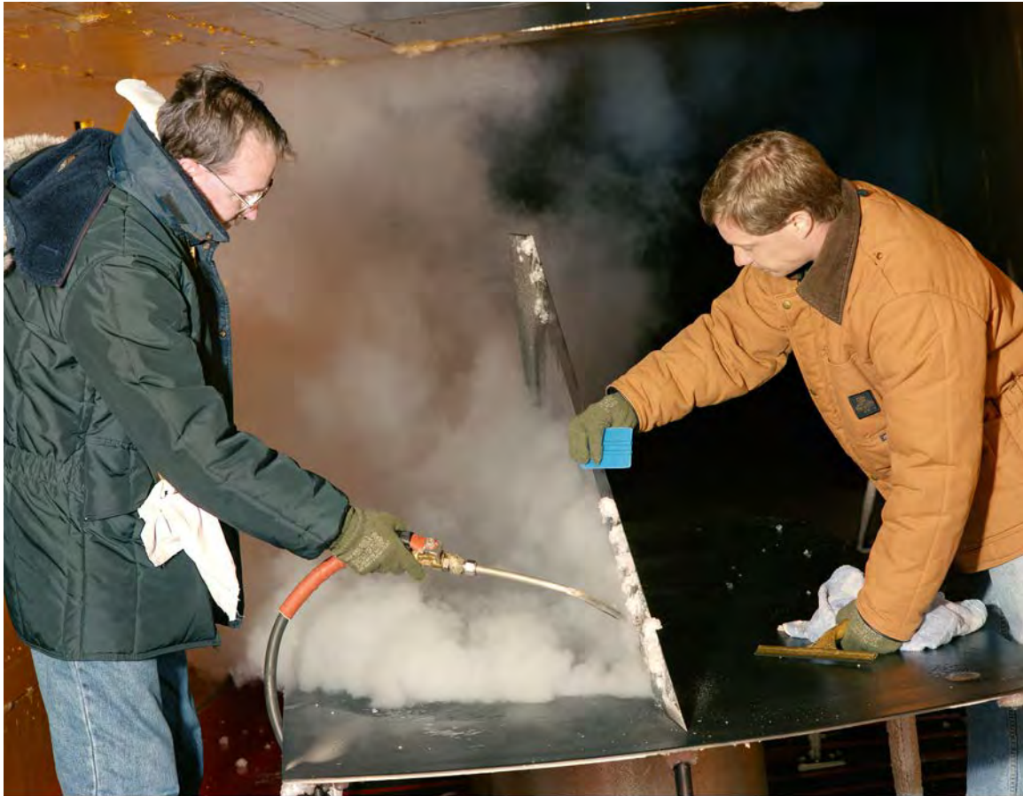
Figure 3-52. This photo shows an icing test of a delta wing in the Icing Research Tunnel (NASA-GRC photo C-95-2932).
