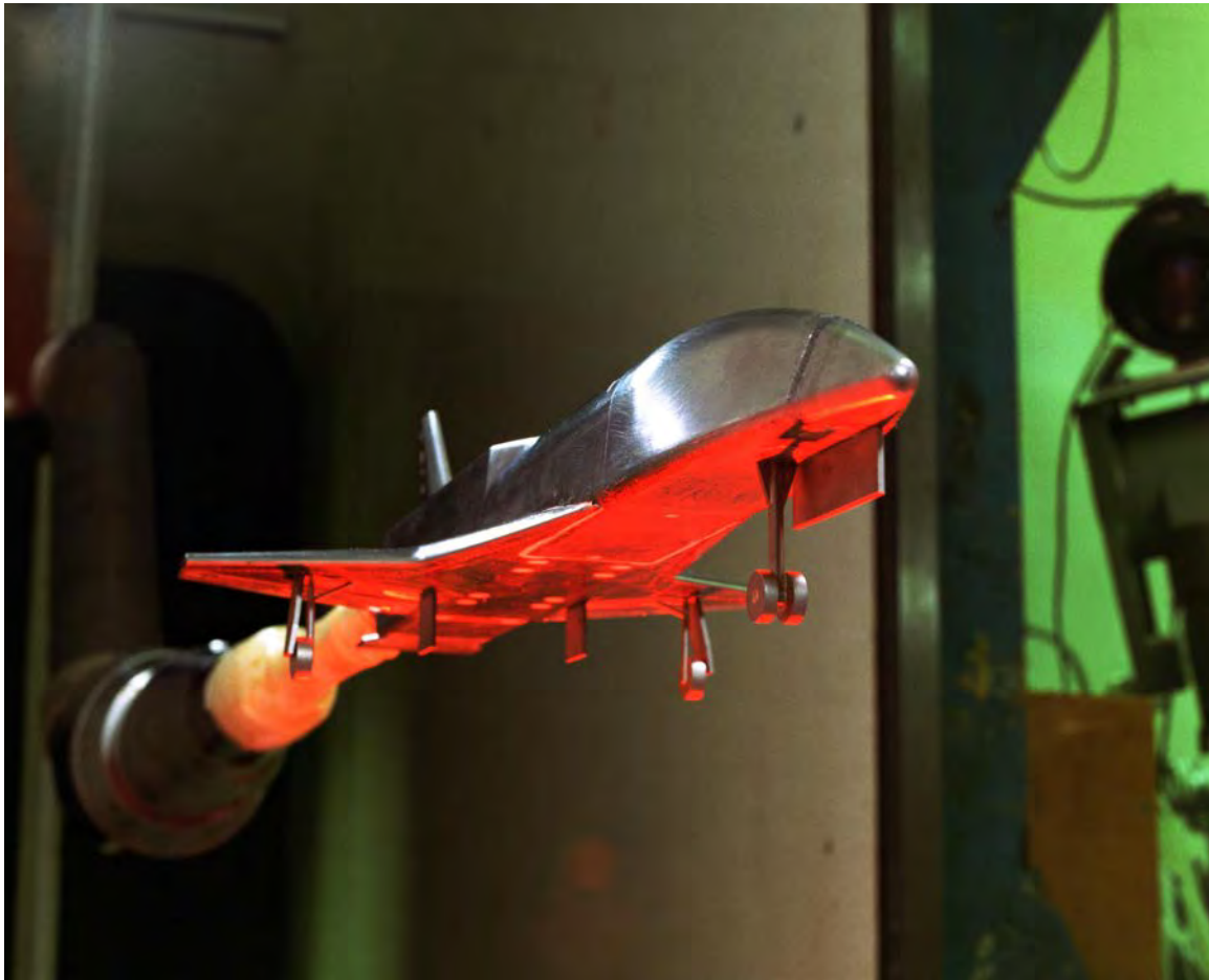
Figure 3-56. A metal model of the X-34 reusable launch vehicle being tested in the Low-Turbulence Pressure Tunnel at Langley Research Center, 1997 (NASA-LaRC photo EL-1997-00048).
