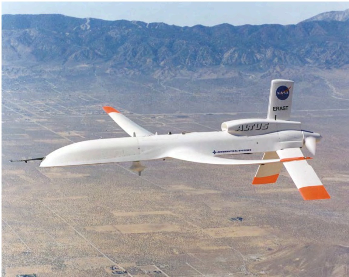
Figure 3-21. The San Gabriel range is visible as the remotely piloted Altus II flies over Southern California's high desert, 29 June 1998 (NASA photo: EC98-44684, General Atomics).
