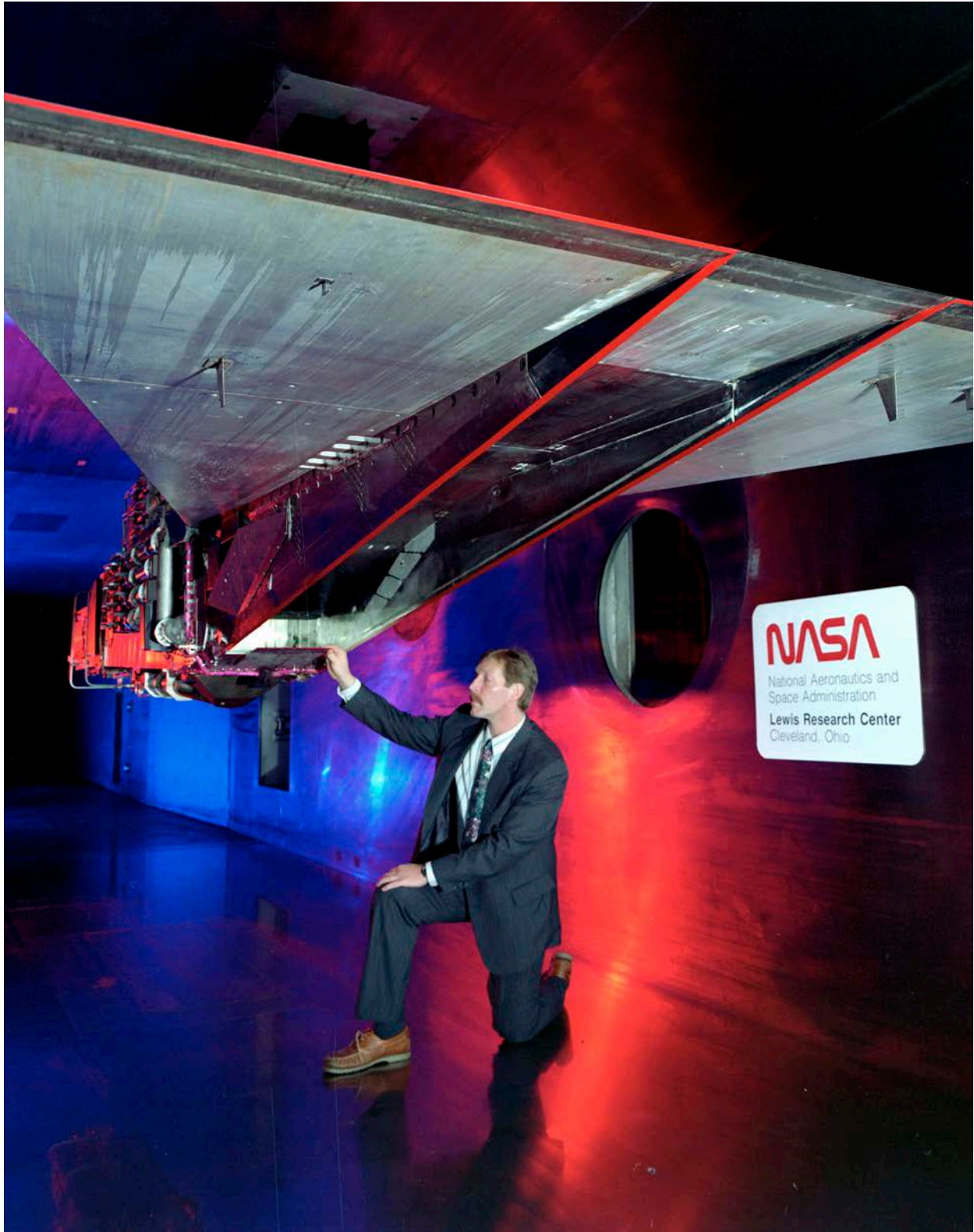
Figure 3-47. A researcher checks the configuration of the Mach 5 inlet mounted in the 10- by 10-Foot Supersonic Wind Tunnel (NASA-GRC photo C-1992-5734).
