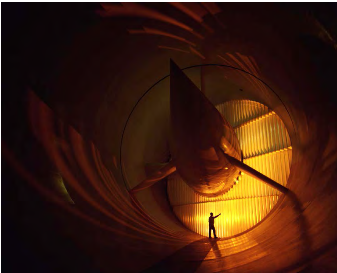
Figure 3-45. This photo shows a technician preparing to unlatch the door built into one of the guide vanes of the 16-Foot Transonic Wind Tunnel (NASA-LaRC photo EL-1996-0003).
