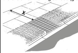
sides of a curb ramp, curb ramps are allowed to have **returned curbs**. A curb ramp with returned curbs is required to have a landing with maneuvering space at the top of the ramp ("**x**" in the illustration to the left) that is at least 48 inches because people using mobility devices need an area to turn when getting on and off the ramp. [§ 4.7.5; Fig. 12(b)]
