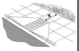
than 48 inches, then the slope of the flared sides must be no more than 8.33 percent (1:12). If "x" is 48 inches or more, then the flared sides may slope up to 10 percent (1:10) but not more. [§ 4.7.5; Fig. 12(a)]
