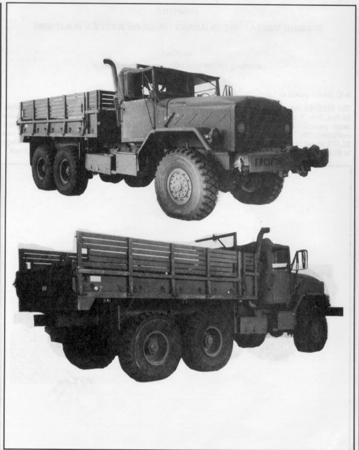
Figure 8-2. Front and rear views of unrigged M925A1, 5-ton cargo truck
