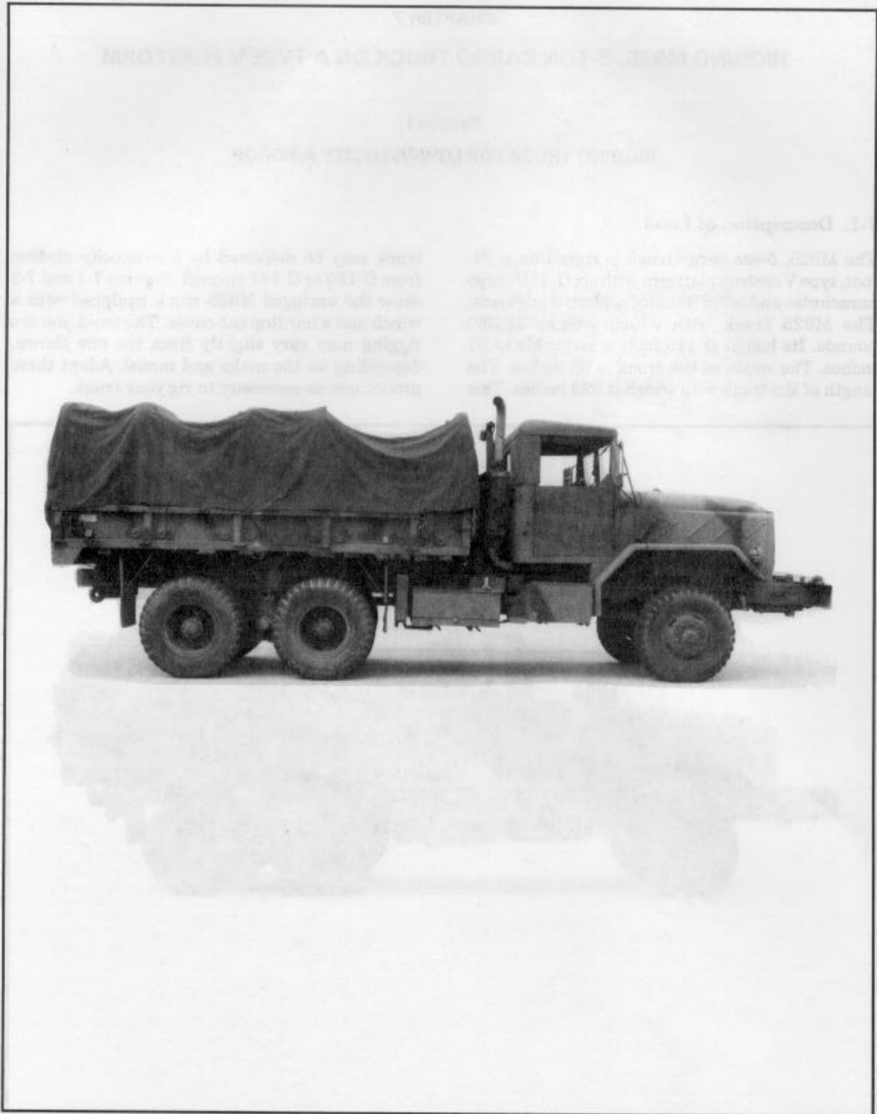
Figure 7-2. Right side of unrigged M925, 5-ton cargo truck
