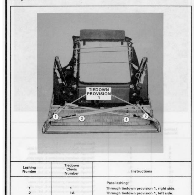
Figure 4-28. Lashings 1 through 4 installed
