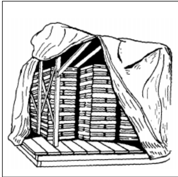
Figure 8-1. Cement Stored Under Tarpaulins
