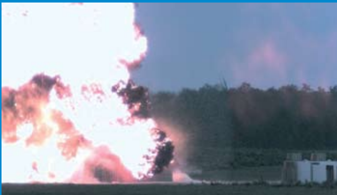
Fig. 4: The first explosion. Note the blast wave between the fireball on the left and the reaction structure on the right.
