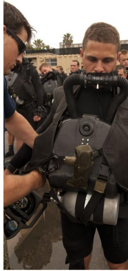
The closed-circuit oxygen underwater breathing apparatus, MK 25, is used by SEALs so that their presence can go undetected during dive missions. While the upside of the unit is that it prevents any exhaust bubbles from surfacing, it also comes with a long list of risks not found with open-circuit units. (U.S. Navy photo by MC2 Dominique Canales)
