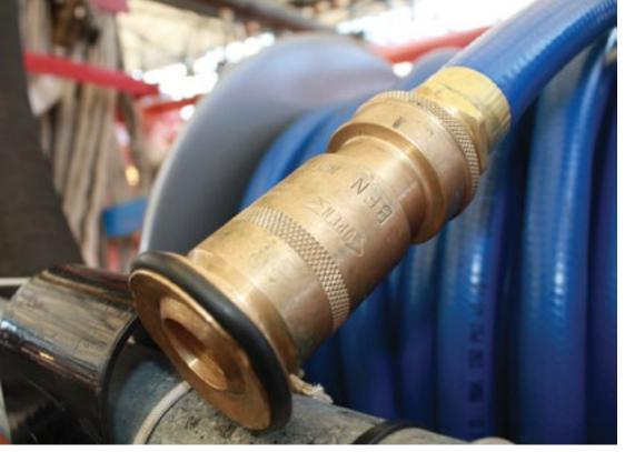
Norfolk Naval Shipyard and USS *Newport News* project team develops this non-collapsible fire hose to enhance firefighting capability.
